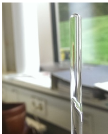
Figure SI-6. Photography of dissolving PDMS gel in IPC/CDCl 3 solution
