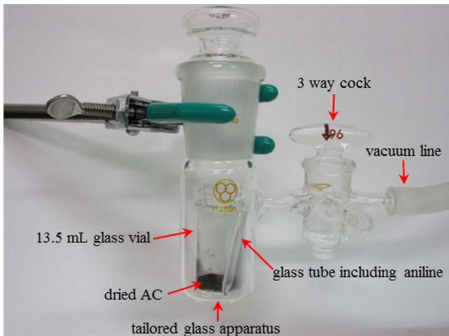
**Figure S1.** Experimental setup for sample preparation.
