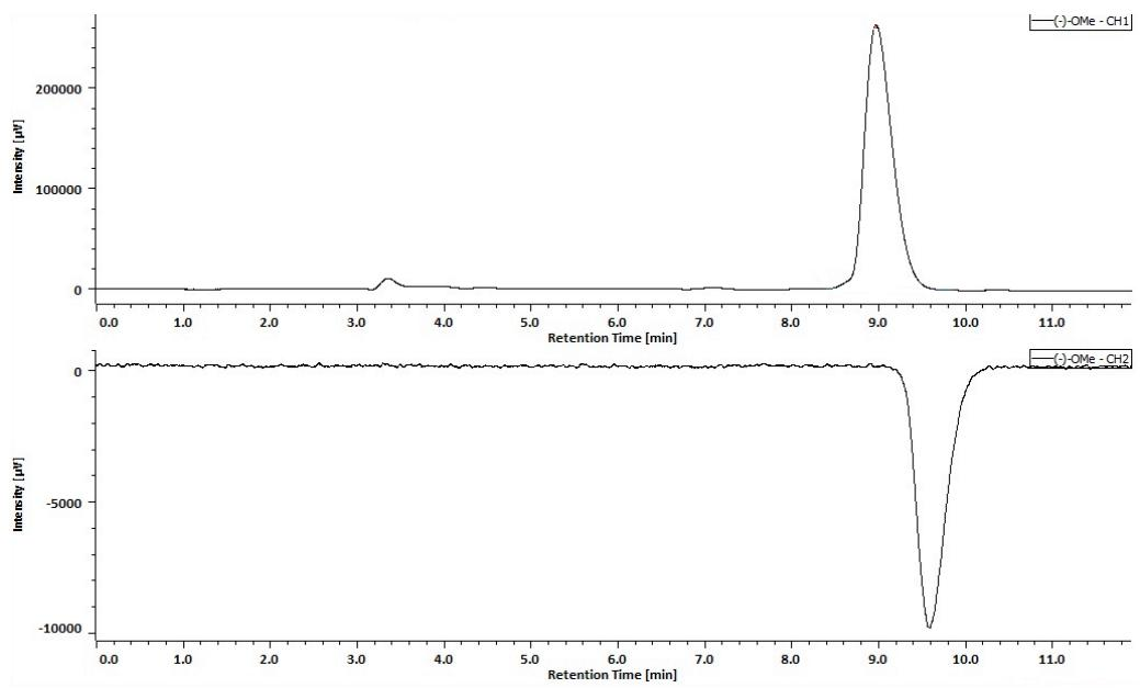
**Figure S9** SFC chart of the separated (-)-6. Column CHIRALPAK IA (eluent=  $\text{CH}_2\text{Cl}_2$  0.5 mL/min,  $\text{CO}_2$  0.8 mL/min), UV and CD detector absorbed at 254 nm.
