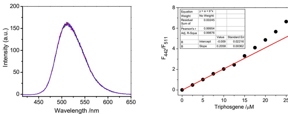
**Fig. I.** Left: Multi-recorded fluorescence spectra of the solution of 5  $\mu\text{M}$  Phos-1. Right: Calibration curve of fluorescence ratio ( $F_{442}/F_{511}$ ) of 5  $\mu\text{M}$  Phos-1 solutions as a function of triphosgene concentration,  $\lambda_{\text{ex}} = 410 \text{ nm}$ .
