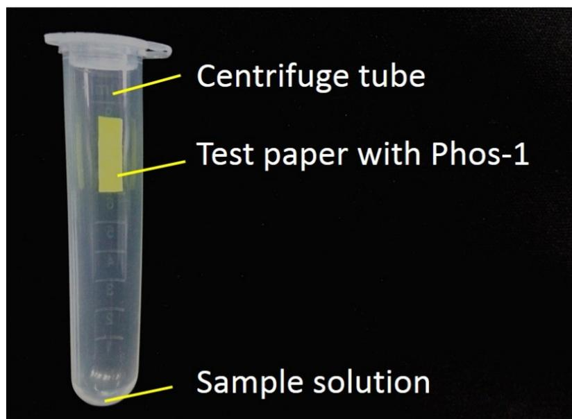
**Fig. S6** Schematic diagram of detection device of phosgene gas and other sample vapor.
