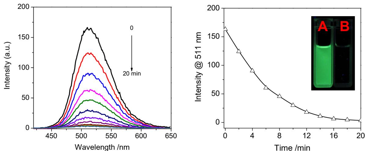
**Fig. S5** Left: Time-dependent fluorescence spectra of Phos-1 (5 μM) DCE solution after bubbled a NO bubble, recorded over 20 min,  $\lambda_{\text{ex}} = 410$  nm. Right: Plot of fluorescence intensity at 511 nm vs. time. Inset: fluorescence images of above solutions before (A) and after (B) under 365 nm light.
