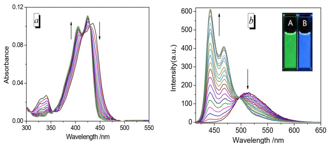
**Fig. S2** Time-dependent UV/vis absorption (left) and fluorescence (right) spectra of Phos-1 (5  $\mu\text{M}$ ) in the presence of triphosgene (25  $\mu\text{M}$ ) in DCE containing TEA (250  $\mu\text{M}$ ). Data were recorded over 20 min,  $\lambda_{\text{ex}} = 410$  nm. Inset: photos of above solutions of Phos-1 before (A) and after (B) under 365 nm light.
