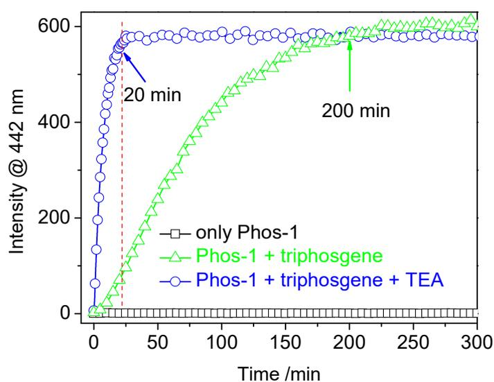
**Fig. S3** Time-dependent fluorescence intensity of 5  $\mu\text{M}$  Phos-1 (black) DCE solutions in the presence of 25  $\mu\text{M}$  triphosgene without (green) or with 250  $\mu\text{M}$  TEA (blue), excitation at 410 nm.
