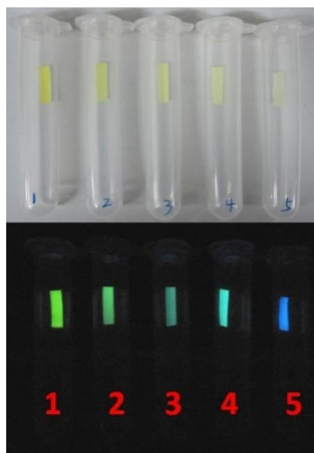
**Fig. S7** Photograph of color (up) and fluorescence (down) response of the Phos-1 test papers upon exposure to vapor of various amounts of triphosgene. (1): 0 mg/L, (2): 1 mg/L, (3): 2 mg/L, (4): 3 mg/L, (5): 4 mg/L, in 25  $\mu$ L DCE solution containing 0.4 % v/v TEA.
