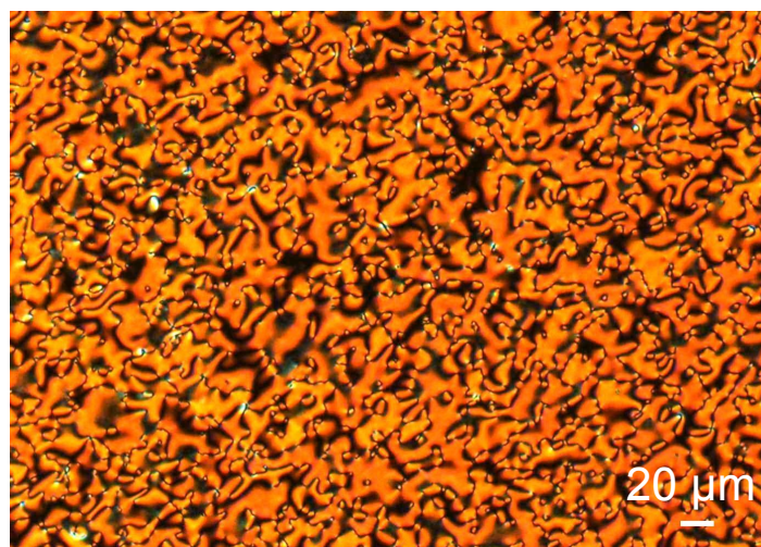
Fig. S11 Polarizing optical micrograph of compound 7b at room temperature on cooling from the isotropic melt between crossed polarizers.
