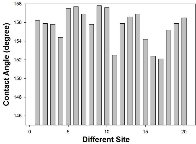
Figure S1. The contact angles of an entire super-hydrophobic substrate
