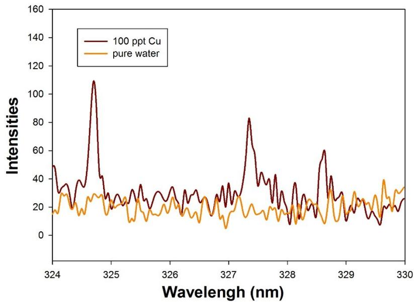
Figure S2. The LIBS signal of pure water and 100 *ppt* Cu solution using the sample container with super-hydrophobic substrate
