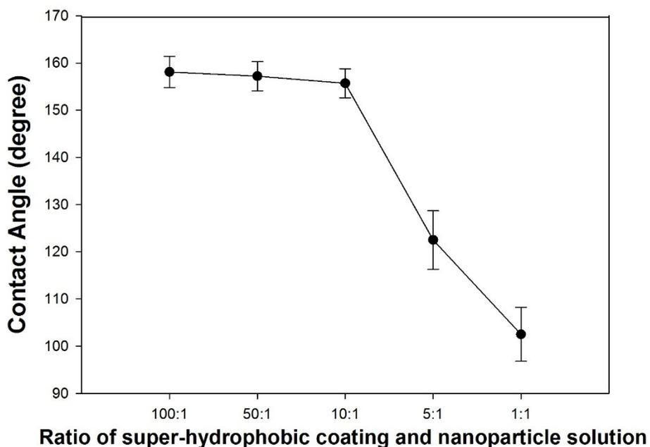
Figure S3. The contact angle of different ratio of super-hydrophobic coating and nanoparticle solution
