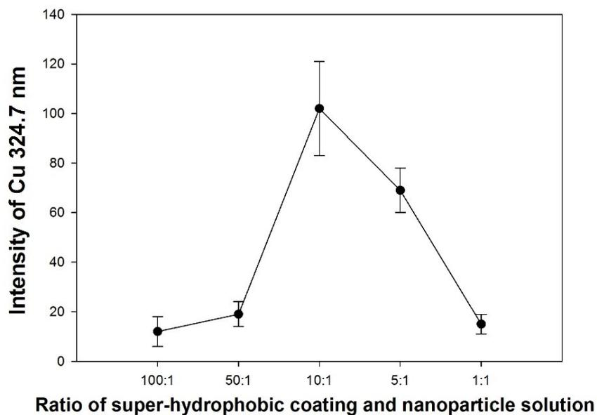
Figure S4. The LIBS intensity of Cu 324.7 nm line (100 ppt Cu solution) of different ratio of super-hydrophobic coating and nanoparticle solution
