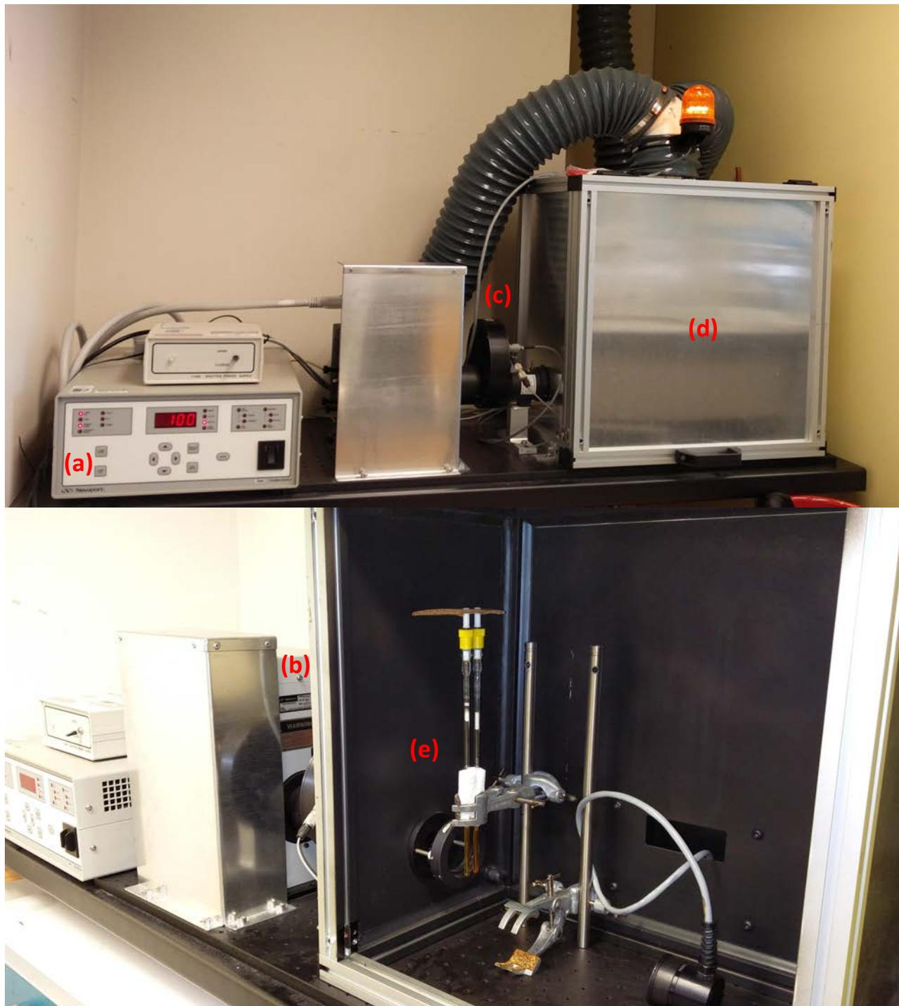
**Figure S-4:** Photolysis equipment (100 W Hg arc lamp): power supply (a), arc lamp (b), safety shutter and IR filter (c), interlocked reaction chamber (d), quartz NMR tubes held in beam (e).
