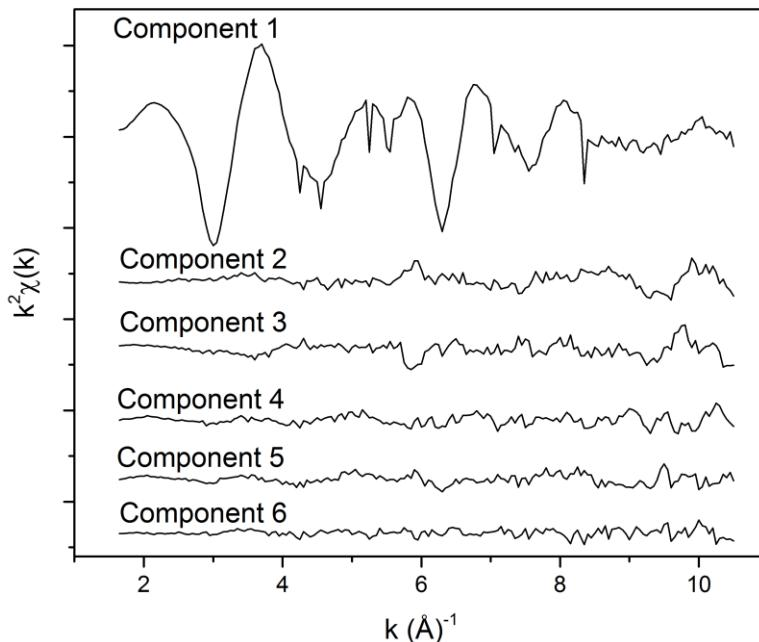
Figure S4. The first six principal components derived from nine Eu L<sub>III</sub>-edge  $k^2$ -weighted EXAFS spectra of a Eu solution with 7.5 mM Me-BTPhen in an ionic liquid solvent. Components 7-9 (not shown) are similar to components 2 – 6. These data reveal only one mathematical component in the EXAFS spectra, indicating an adequate fit should be achievable from a single appropriate structure model.
