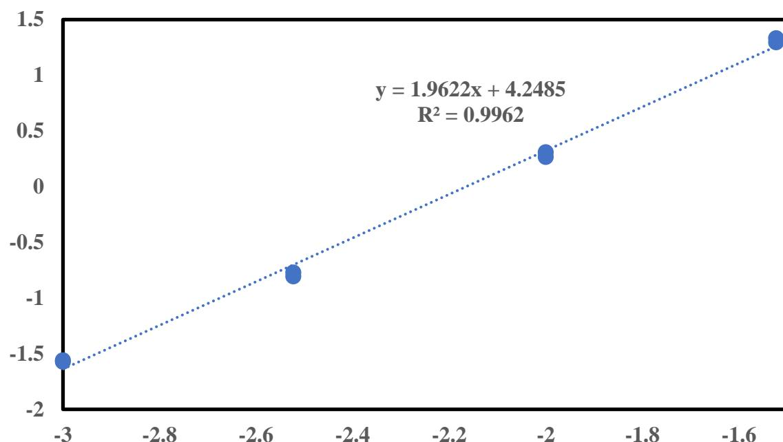
Figure S3. Slope Analysis of Me-BTPhe with Eu extracted from 0.1 M  $\text{HNO}_3$ . The y-axis represents the  $\log D_{\text{Eu}}$  and the x-axis is the  $\log[\text{Me-BTPhe}]$ .
