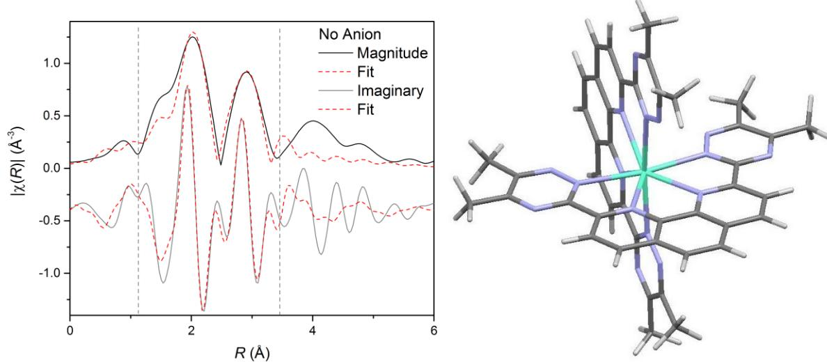
Figure S7. (Left) Rejected XAFS fit from structure model  $[\text{Eu}(\text{Me-BTPhen})_2]^{3+}$ . (Right) DFT-optimized structure model used for preparation of the structure model.
