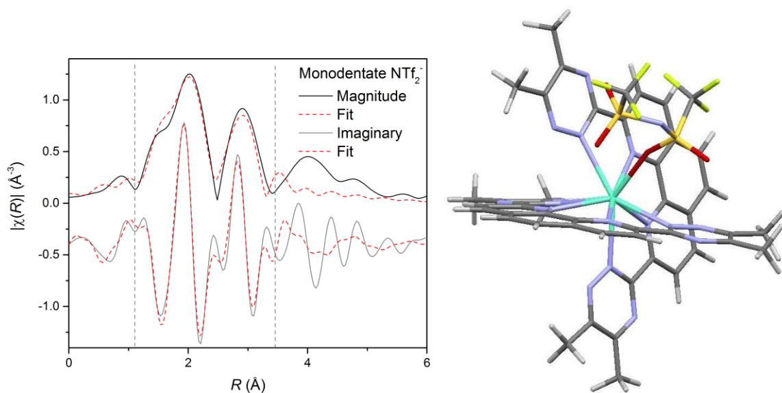
Figure S10. (Left) Rejected XAFS fit from structure model  $[\text{Eu}(\text{Me-BTPhen})_2\text{NTf}_2]^{2+}$ . (Right) DFT-optimized structure model used for preparation of the structure model.
