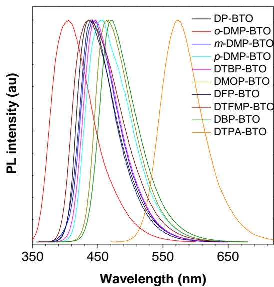
**Fig. S4** Photoluminescence (PL) spectra of the powders of the new luminogens.
