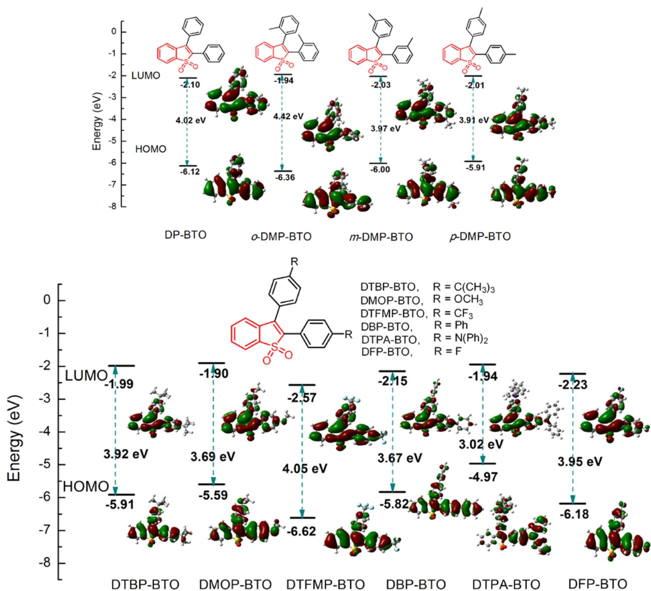
**Fig. S2** The HOMOs and LUMOs of the new luminogens at the B3LYP/6-31G (d, p) level in the gas phase based on the ground-state geometries.
