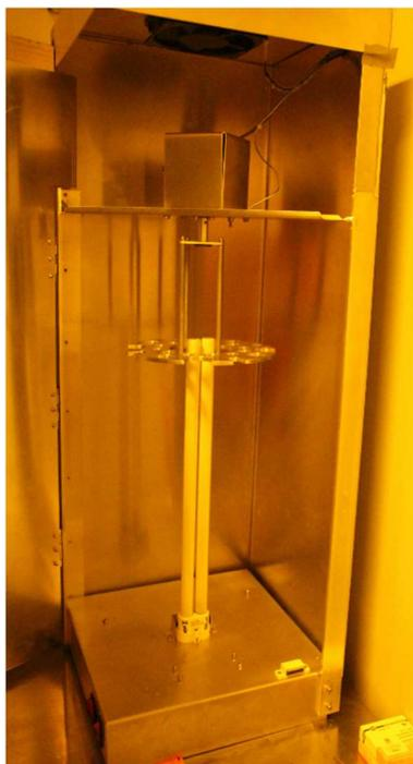
**Figure S17.** Picture of the employed custom built photoreactor equipped with the Philips PL-L lamp.
