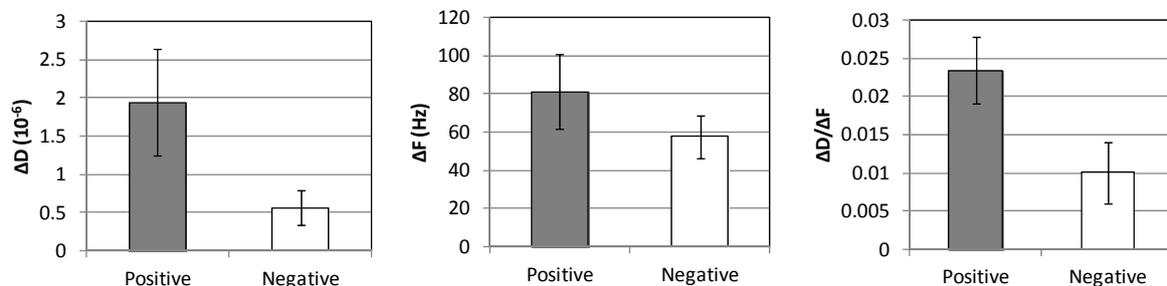
Fig. S3: Comparison of changes in frequency (F), dissipation (D) and acoustic ratio ( $\Delta D/\Delta F$ ) between positive and negative PCR reactions (measurements were repeated 5 times).
