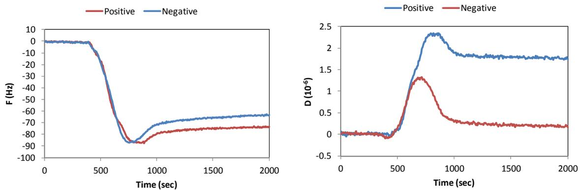
Fig. S2: Comparison of changes in frequency (F) and dissipation (D) of a positive and a negative PCR reaction monitored in real-time with QCM-E4.
