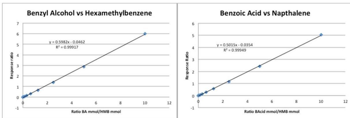
**Figure S4:** Plot of calibration curves for benzyl alcohol and benzoic acid against a hexamethylbenzene internal standard.
