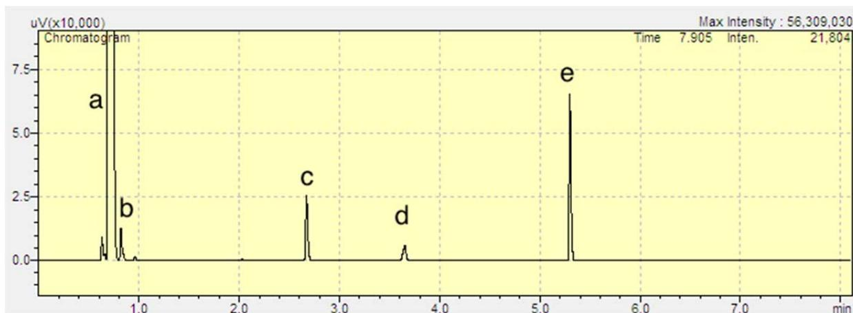
**Figure S5:** Representative GC chromatogram of conversion of benzyl alcohol to benzoic acid. Peaks: a) Ethyl acetate; b) toluene; c) benzyl alcohol; d) benzoic acid; e) hexamethylbenzene.
