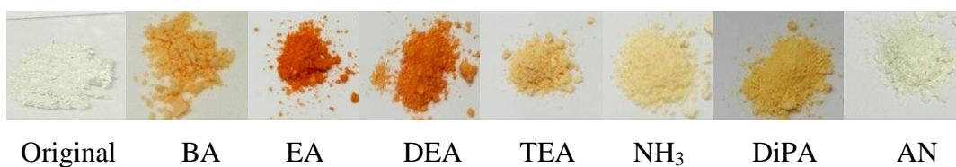
Fig. S5 Pictures showing the color change of powder samples of the UiO-67-dmbpy when exposed to ammonia/amine vapors. BA = butylamine, EA = ethylamine, DEA = diethylamine, TEA = triethylamine, DiPA = diisopropylamine, AN = aniline.
