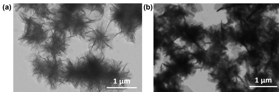
Fig. S4 TEM photos of  $\text{CPO}@\text{Ca}_3(\text{PO}_4)_2$  hybrid composites with or without SA coating.
