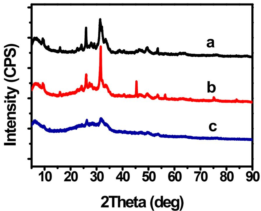
Fig. S3 X-ray diffraction (XRD) spectra of  $\text{Ca}_3(\text{PO}_4)_2$  (Curve (a)),  $\text{BSA}@\text{Ca}_3(\text{PO}_4)_2$  (Curve (b)): SA-coated  $\text{BSA}@\text{Ca}_3(\text{PO}_4)_2$  (Curve (c)).
