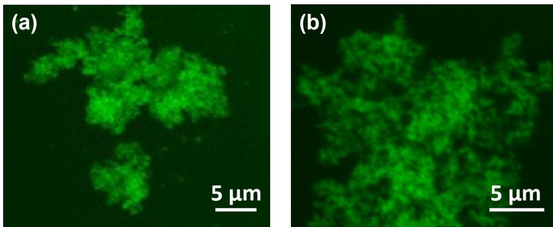
Fig.S1 CLSM micrograph of (a)BSA@Ca<sub>3</sub>(PO<sub>4</sub>)<sub>2</sub> and (b)SA-coated BSA@Ca<sub>3</sub>(PO<sub>4</sub>)<sub>2</sub>.
