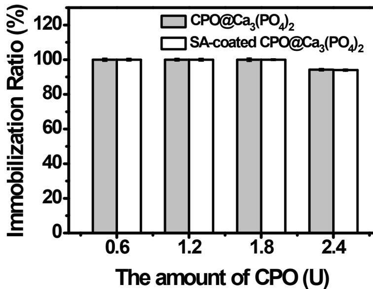
Fig. S5 The immobilization capacity of CPO@Ca<sub>3</sub>(PO<sub>4</sub>)<sub>2</sub> and SA-coated CPO@Ca<sub>3</sub>(PO<sub>4</sub>)<sub>2</sub> hybrid composites. (Experiment conditions: PBS buffer (10mM, pH 7.4, 180  $\mu$ L), aqueous CaCl<sub>2</sub> solution (180 mM, 20  $\mu$ L), containing different amount of CPO.)
