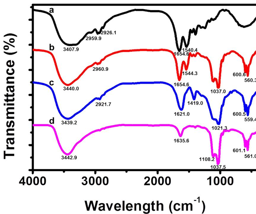
Fig. S2 The FTIR spectra of BSA (Curve (a)), BSA@Ca<sub>3</sub>(PO<sub>4</sub>)<sub>2</sub> (Curve (b)), SA-coated BSA@Ca<sub>3</sub>(PO<sub>4</sub>)<sub>2</sub> (Curve (c)), and Ca<sub>3</sub>(PO<sub>4</sub>)<sub>2</sub> (Curve (d)).
