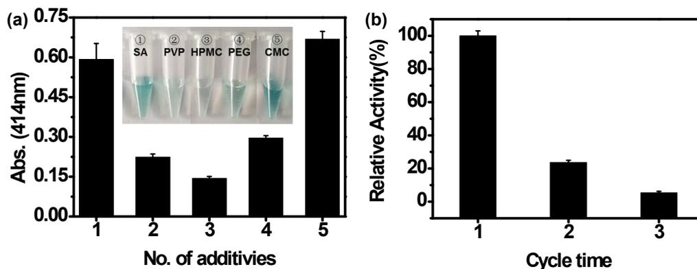
Fig. S8 (a) The enzyme activity with of different additives coating CPO@Ca<sub>3</sub>(PO<sub>4</sub>)<sub>2</sub>, inset: photographs showing visible detection; (b) The reusability of CMC-coated CPO@Ca<sub>3</sub>(PO<sub>4</sub>)<sub>2</sub>. (For the CPO activity assay, 400  $\mu$ L of phosphoric acid buffer solution (pH 2.75, 10 mM) containing 0.5 U CPO and 0.25 mM ABTS<sup>2-</sup>, 4.4 mM H<sub>2</sub>O<sub>2</sub> followed by reaction for 10 min at room temperature).
