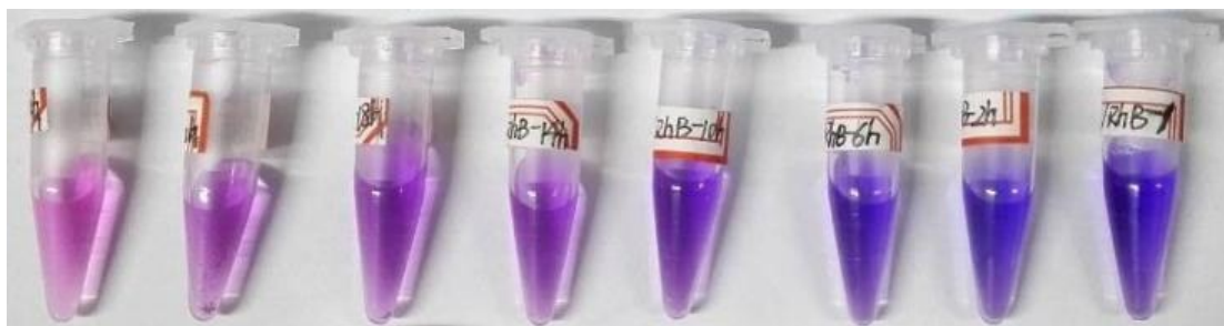
Fig. S20. Photographs of the color change of the mixed dyes MB/RhB solutions before and after adsorption experiments at given intervals with CIAC-120 . Time increases in the order from the right to the left.
