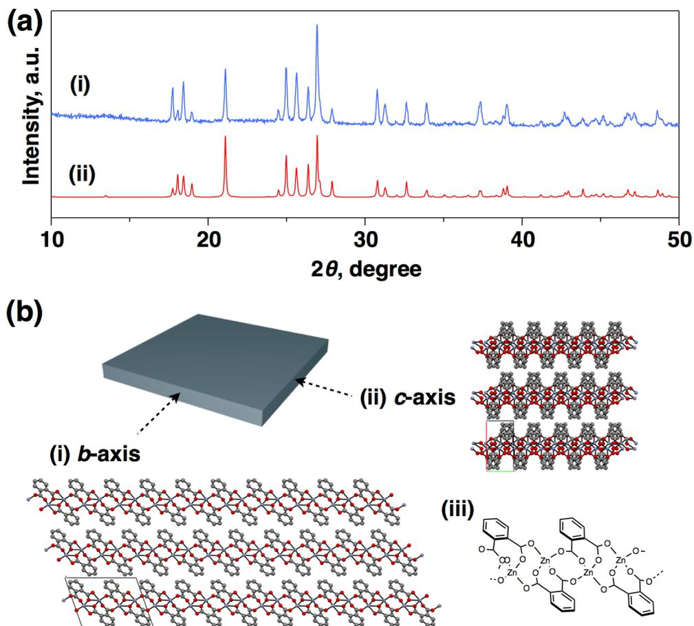
**Fig. S1** (a) Comparison of XRD diffraction patterns: (i) as-prepared MOF powder in this study and (ii) calculated XRD pattern from the cif file (CCDC-908149; ref. 13). (b) representative crystal structure from (i) *b*-axis, (ii) *c*-axis, and (iii) chemical structure drawing of repeating unit.
