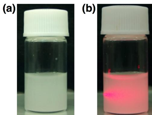
**Fig. S2** Photographs of the DMF dispersion of as-prepared Zn-MOF powder (a, under room lighting; b, with red laser irradiation). The concentration of Zn-MOF sample in DMF is 2 mg/mL.
