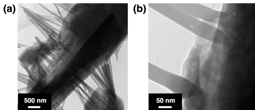
**Fig. S3** TEM images of the MOF crystal surface in the process of the fiber growing, taken at (a) moderate and (b) high magnification.
