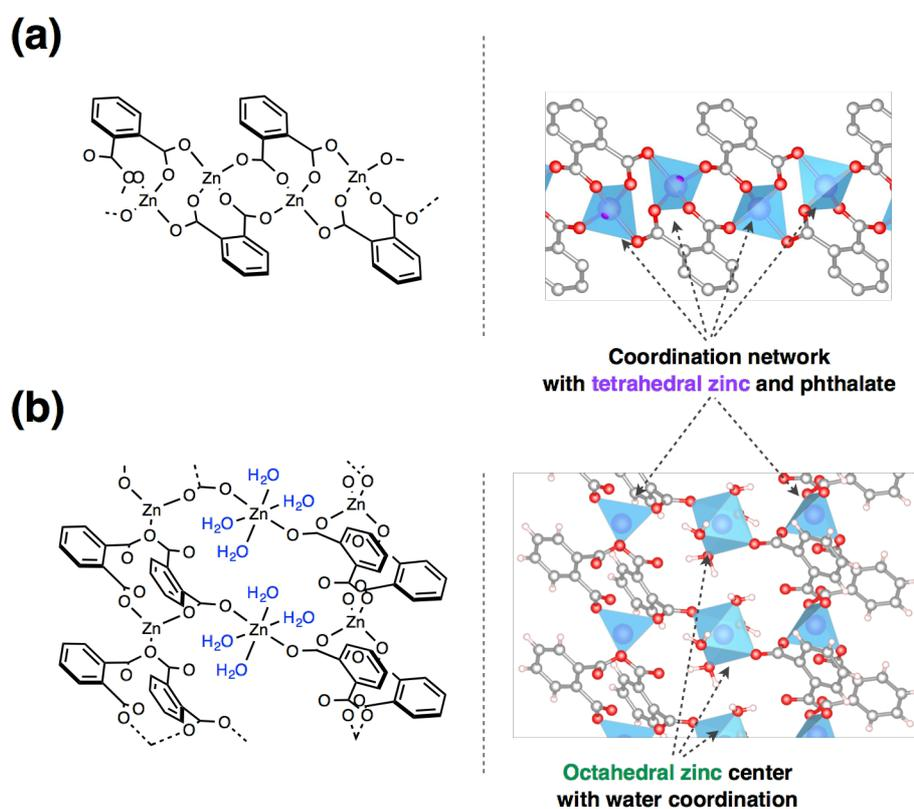
**Fig. S4** Comparison of coordination network structure of (a) MOF sheet and (b) MOF fiber.
