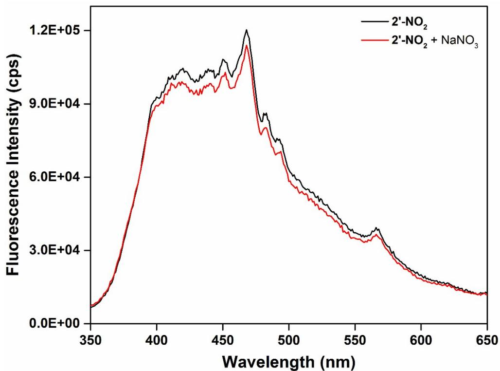
**Figure S30.** Fluorescence response of 2'-NO<sub>2</sub> compound before (black) and after (red) addition of NaNO<sub>3</sub> at 900 s.
