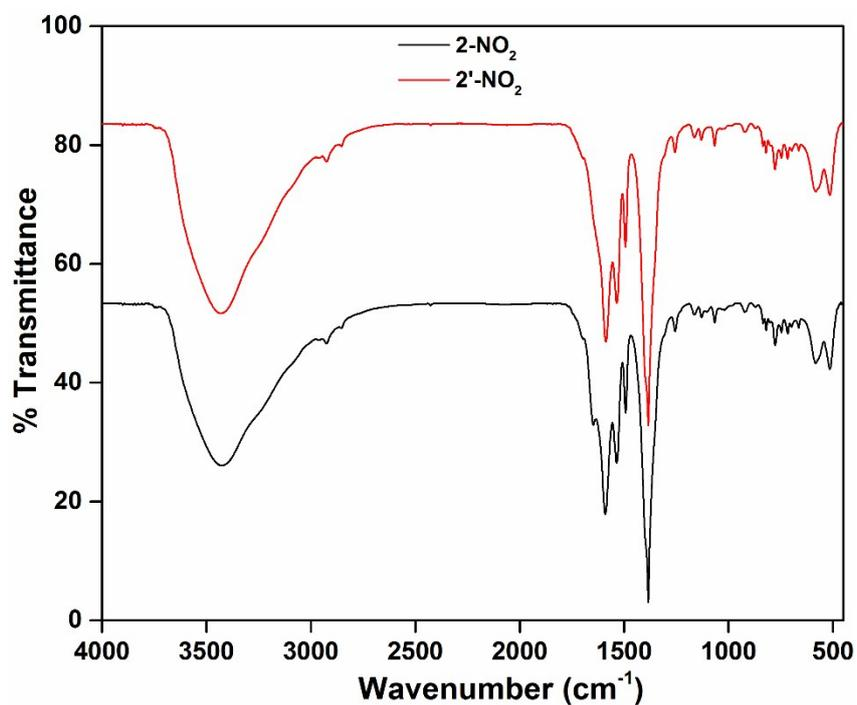
**Figure S2.** FT-IR spectra of as-synthesized 2-NO<sub>2</sub> (black) and activated 2'-NO<sub>2</sub> (red) compound.
