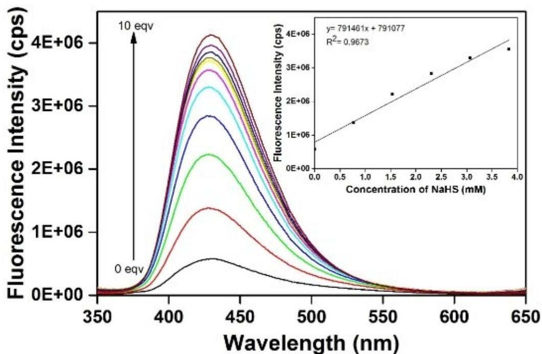
**Figure S33.** Fluorescence response of Zr-UiO-66-N<sub>3</sub> with increasing concentrations of NaHS. All the experiments were carried out in HEPES buffer (10 mM, pH 7.4).
