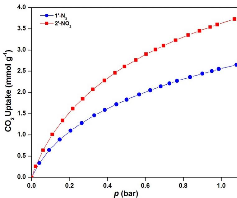
**Figure S4.** Low-pressure  $\text{CO}_2$  adsorption isotherms of the thermally activated  $1'\text{-N}_3$  (blue, circles) and  $2'\text{-NO}_2$  (red, squares) measured at  $0\text{ }^\circ\text{C}$ .
