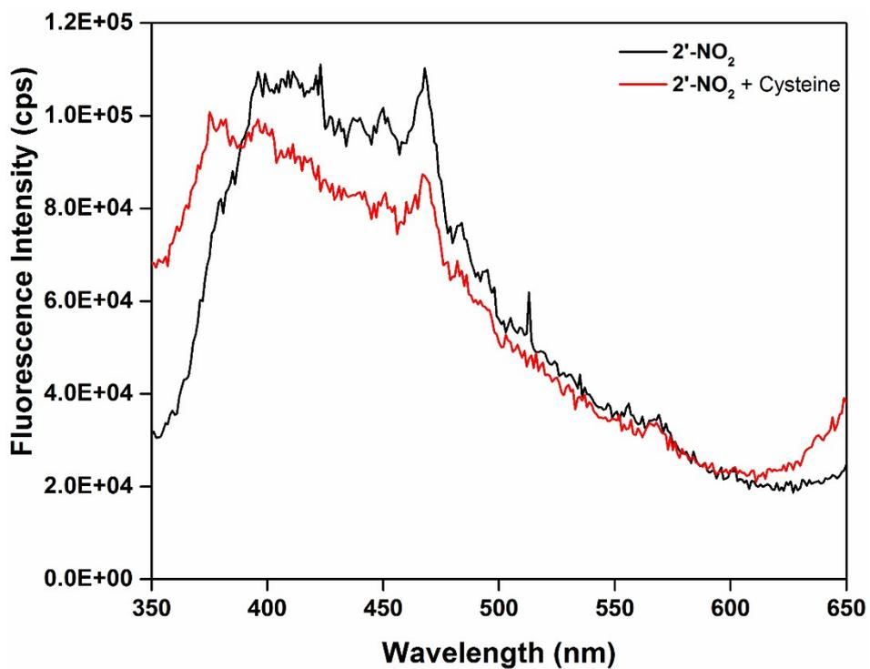
**Figure S23.** Fluorescence response of 2'-NO<sub>2</sub> compound before (black) and after (red) addition of cysteine at 900 s.
