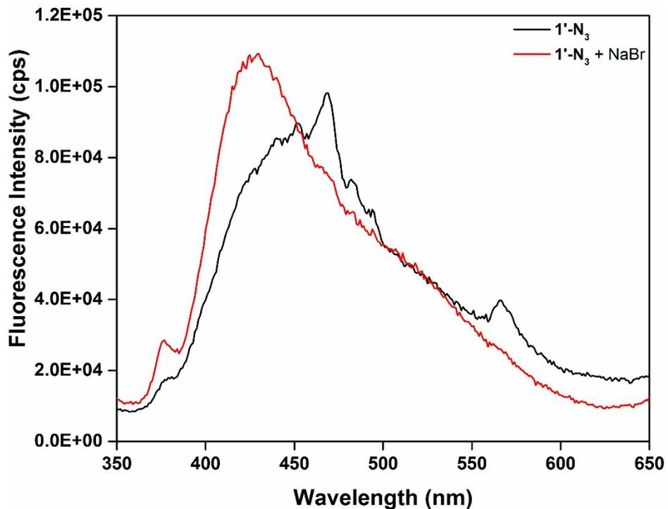
**Figure S18.** Fluorescence response of 1'-N<sub>3</sub> compound before (black) and after (red) addition of NaBr at 900 s.
