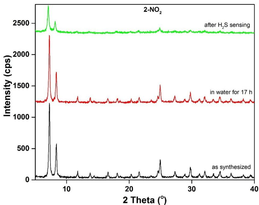
**Figure S10.** XRPD patterns of 2-NO<sub>2</sub> compound in water (red) and after H<sub>2</sub>S sensing experiment (green).
