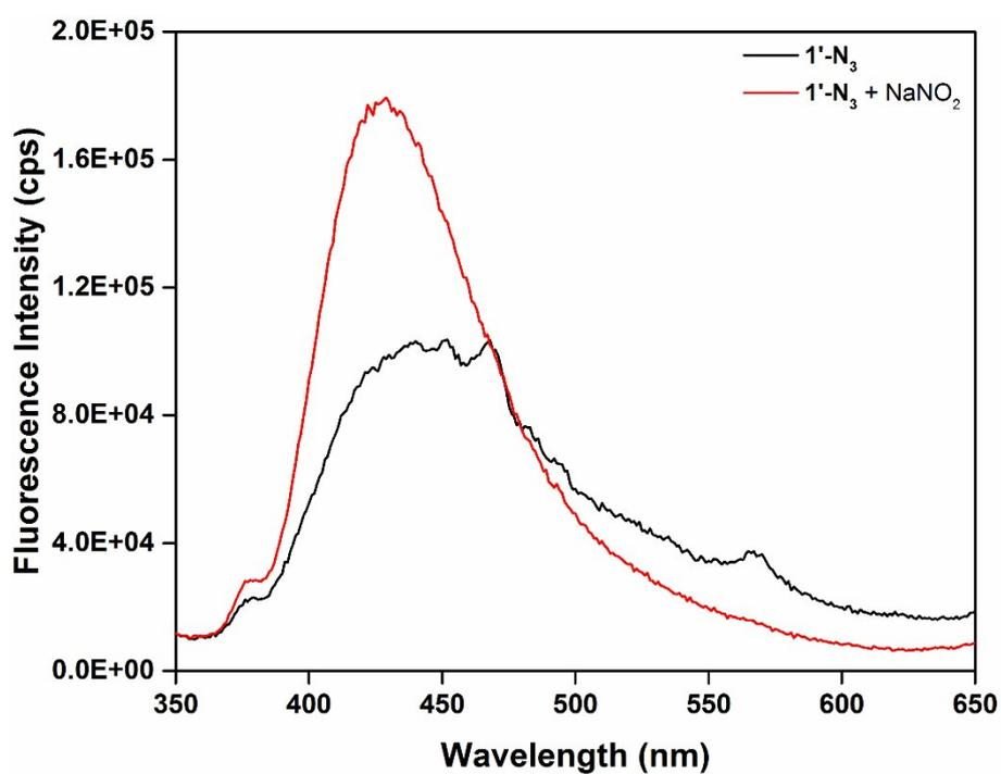
**Figure S20.** Fluorescence response of 1'-N<sub>3</sub> compound before (black) and after (red) addition of NaNO<sub>2</sub> at 900 s.
