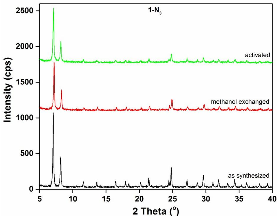
**Figure S7.** XRPD patterns of **1-N<sub>3</sub>** compound in different forms: (i) as-synthesized (black), (ii) methanol-exchanged (red) and (iii) activated at 90 °C (green).
