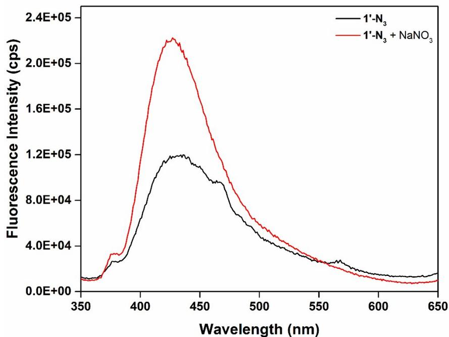
**Figure S21.** Fluorescence response of 1'-N<sub>3</sub> compound before (black) and after (red) addition of NaNO<sub>3</sub> at 900 s.
