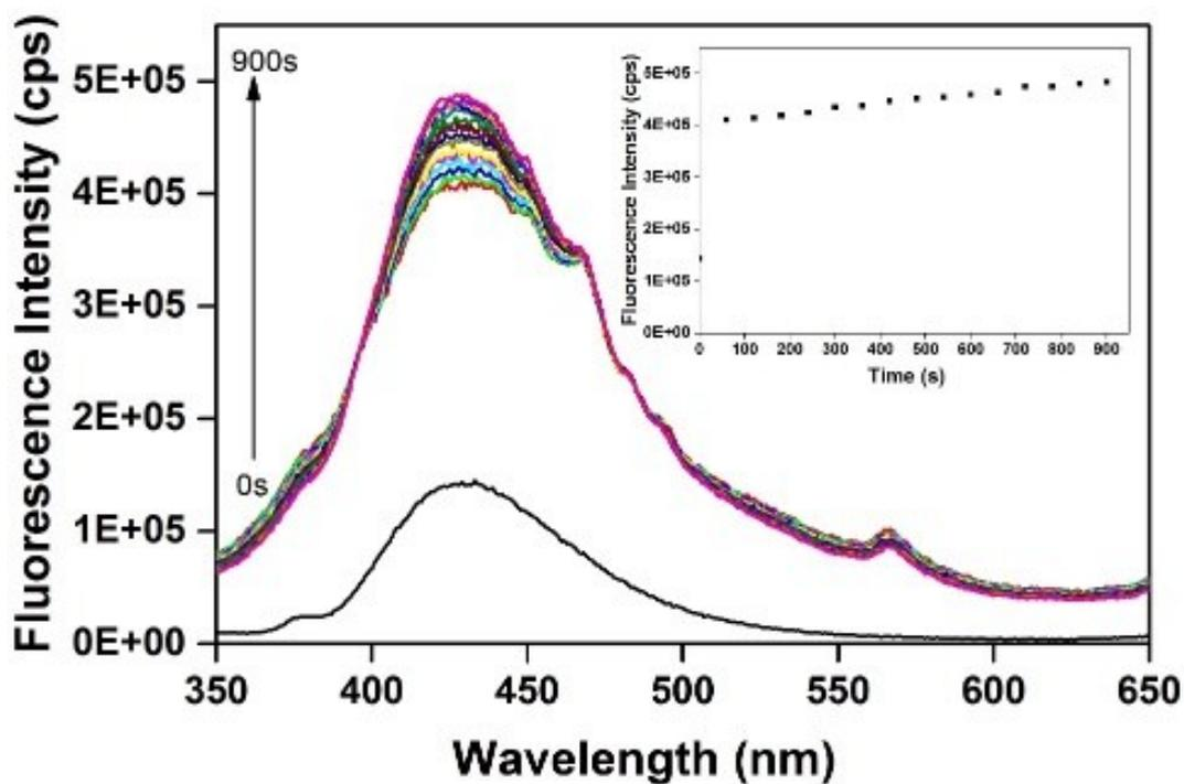
**Figure S12.** Fluorescence turn-on response of Zr-UiO-66-NO<sub>2</sub> towards addition of NaHS at a regular time interval (60 s) up to 900 s. Inset: Time-dependence of the emission intensity at 429 nm.
