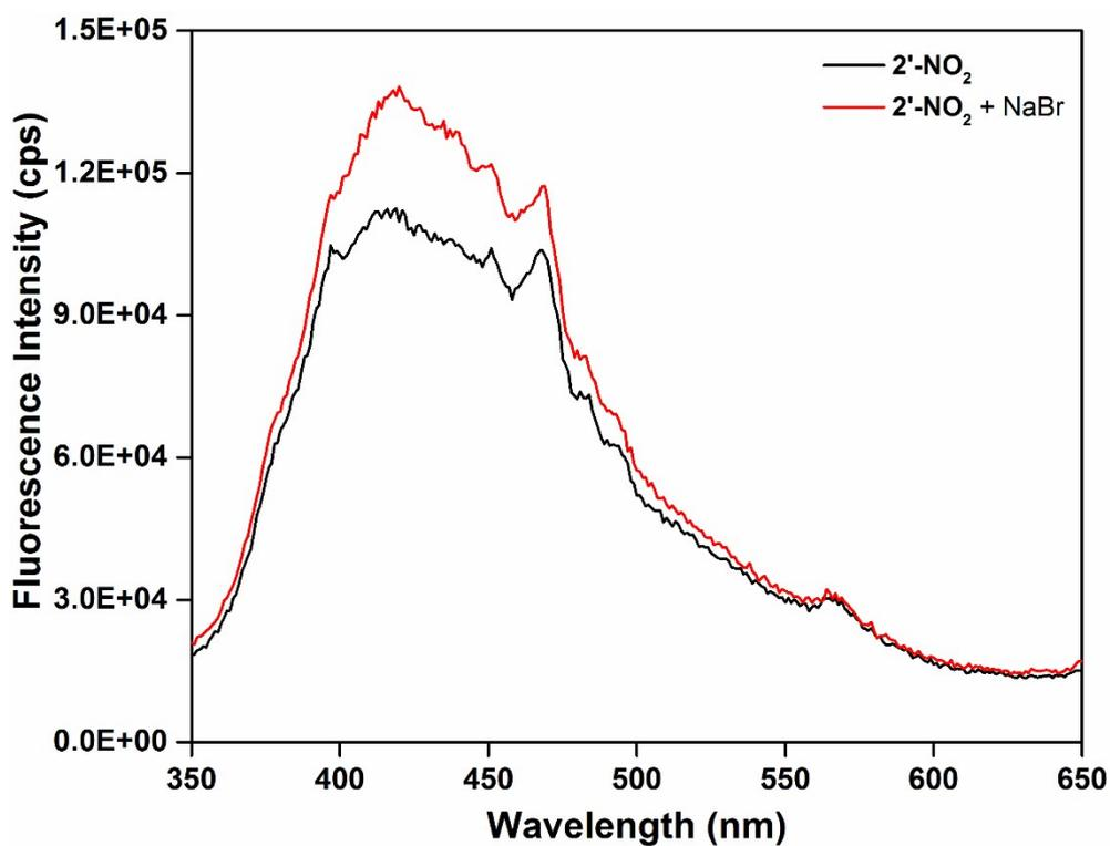
**Figure S27.** Fluorescence response of 2'-NO<sub>2</sub> compound before (black) and after (red) addition of NaBr at 900 s.
