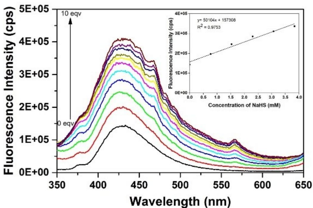
**Figure S34.** Fluorescence response of Zr-UiO-66-NO<sub>2</sub> with increasing concentrations of NaHS. All the experiments were carried out in HEPES buffer (10 mM, pH 7.4).
