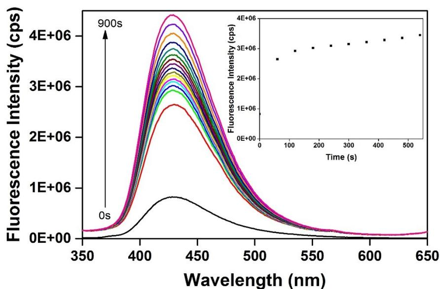
**Figure S11.** Fluorescence turn-on response of Zr-UiO-66-N<sub>3</sub> towards addition of NaHS at a regular time interval (60 s) up to 900 s. Inset: Time-dependence of the emission intensity at 429 nm.
