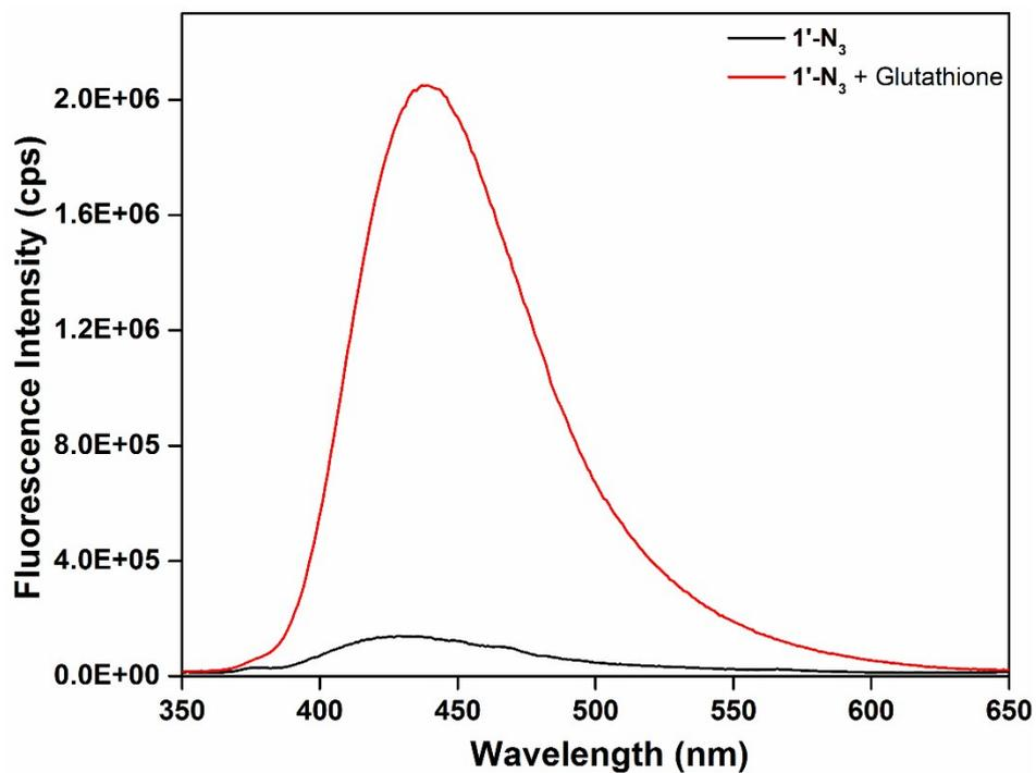
**Figure S16.** Fluorescence response of 1'-N<sub>3</sub> compound before (black) and after (red) addition of glutathione at 900 s.
