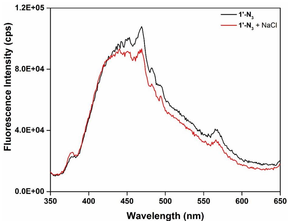
**Figure S17.** Fluorescence response of 1'-N<sub>3</sub> compound before (black) and after (red) addition of NaCl at 900 s.
