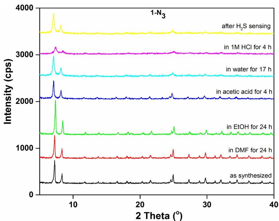
**Figure S8.** XRPD patterns of **1-N<sub>3</sub>** compound in different solvents: as-synthesized (black), DMF (red), EtOH (green), acetic acid (blue), water (cyan), 1M HCl (pink) and after H<sub>2</sub>S sensing experiment (yellow).
