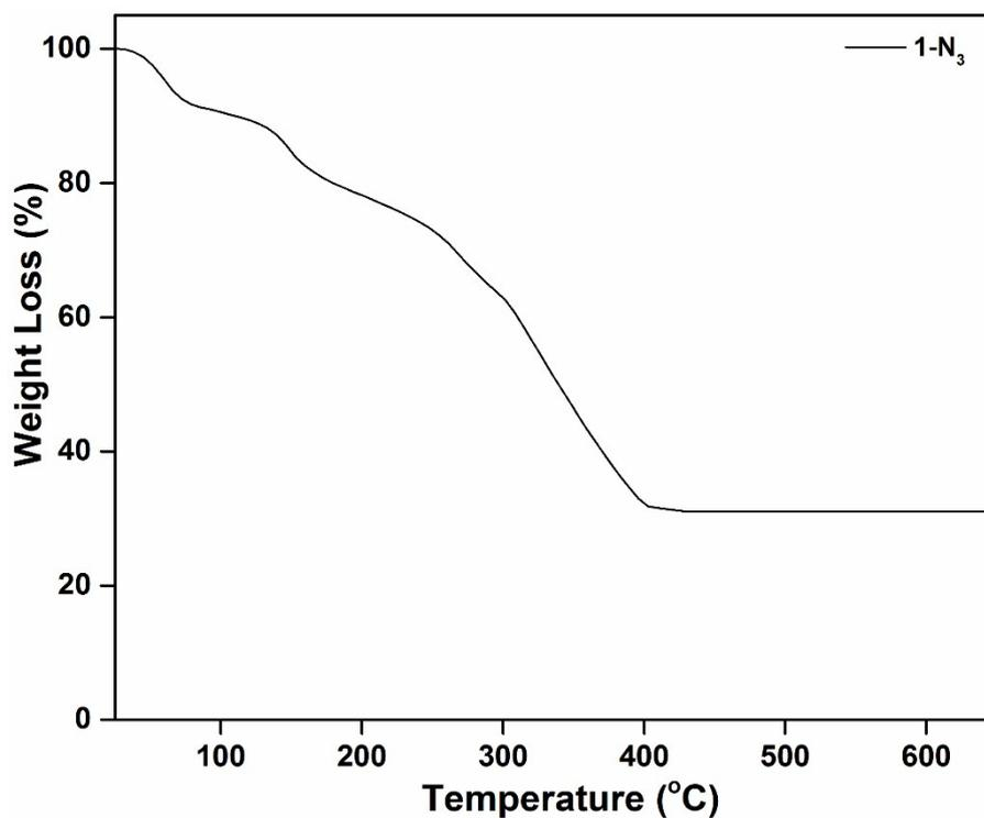
**Figure S5.** TG curves of as-synthesized **1-N<sub>3</sub>** compound recorded in an air atmosphere in the temperature range of 25-650 °C with a heating rate of 5 °C min<sup>-1</sup>.
