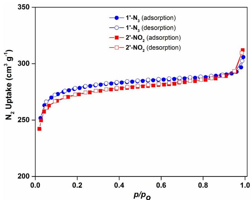
**Figure S3.**  $\text{N}_2$  adsorption (solid symbols) and desorption (empty symbols) isotherms of the thermally activated  $1'\text{-N}_3$  (blue, circles) and  $2'\text{-NO}_2$  (red, squares) recorded at  $-196\text{ }^\circ\text{C}$ .
