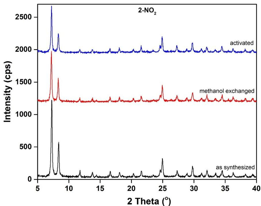
**Figure S9.** XRPD patterns of 2-NO<sub>2</sub> compound in different forms: (i) as-synthesized (black), (ii) methanol-exchanged (red) and (iii) activated at 90 °C (blue).
