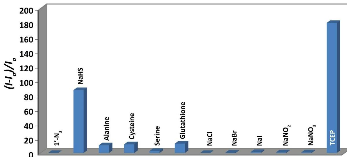
**Figure S31.** Relative fluorescence response of 1'-N<sub>3</sub> towards TCEP (10 equivalents per azide group) after 900 s of analyte addition.
