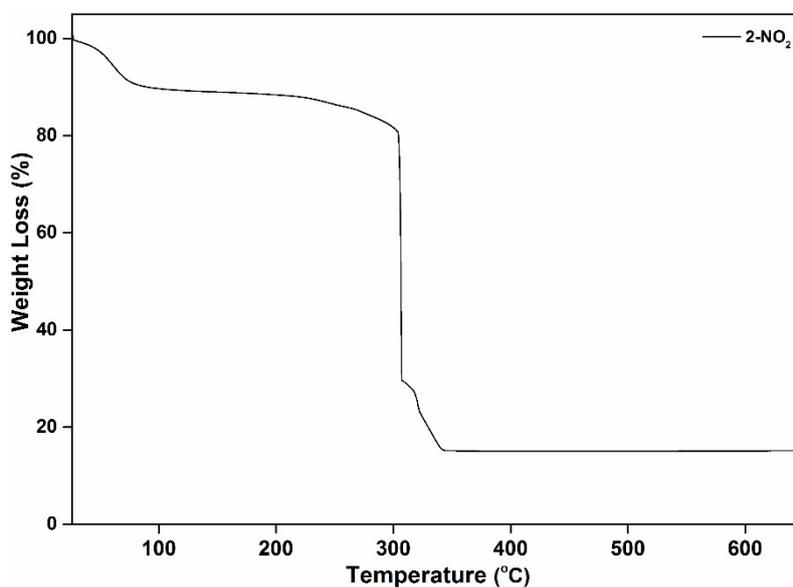
**Figure S6.** TG curves of as-synthesized **2-NO<sub>2</sub>** compound recorded in an air atmosphere in the temperature range of 25-650 °C with a heating rate of 5 °C min<sup>-1</sup>.
