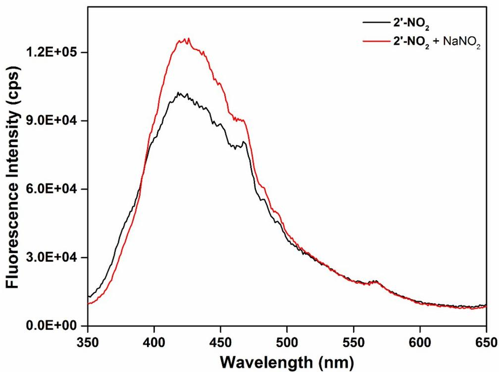
**Figure S29.** Fluorescence response of 2'-NO<sub>2</sub> compound before (black) and after (red) addition of NaNO<sub>2</sub> at 900 s.
