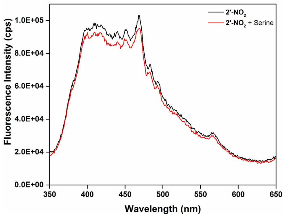
**Figure S24.** Fluorescence response of 2'-NO<sub>2</sub> compound before (black) and after (red) addition of serine at 900 s.
