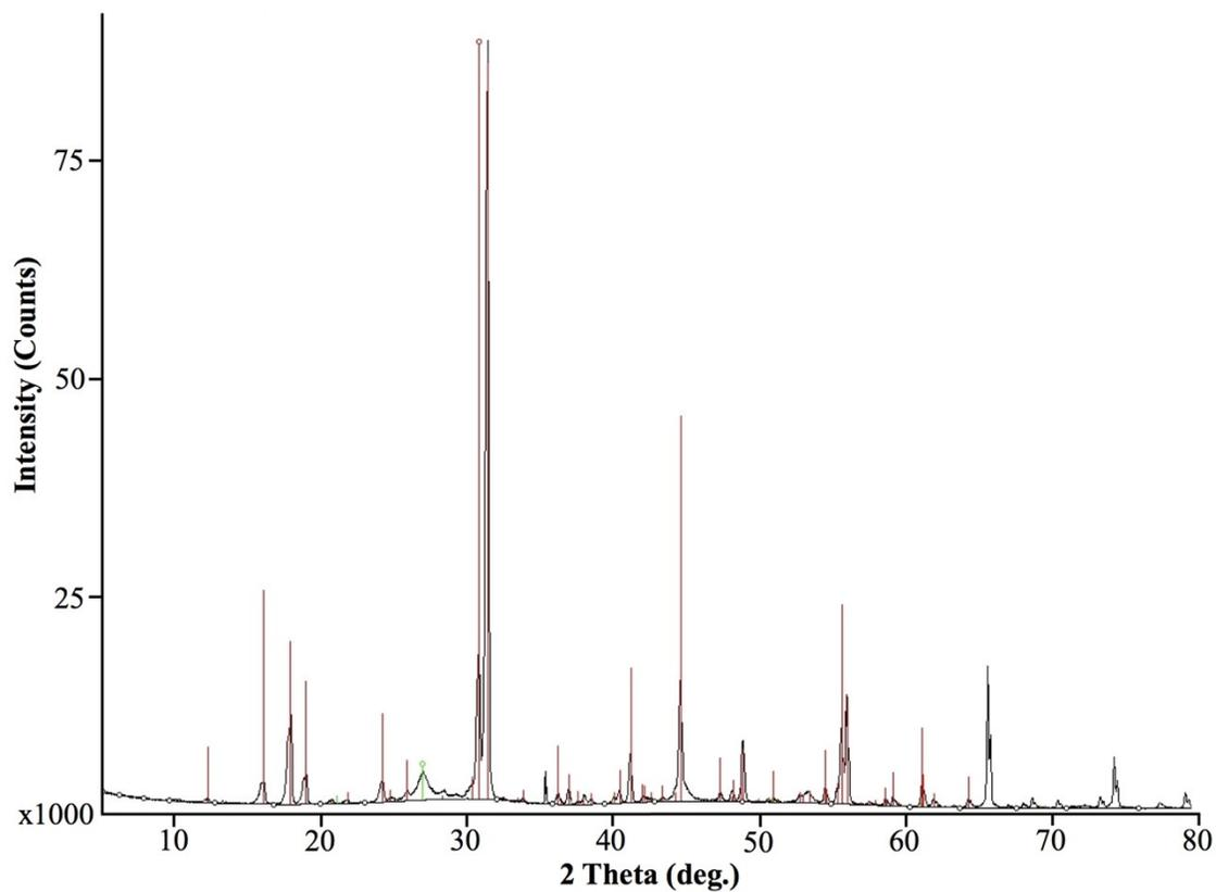
**Figure S-2.** PXRD pattern of  $K_3YSi_2O_7$  doped with 10 % Dy and 0.1 % Eu (**2-Dy,Eu**). The observed pattern is in good agreement with the calculated pattern with a small amount of  $SiO_2$ . The calculated pattern is shown in red and the  $SiO_2$  is shown in green.
