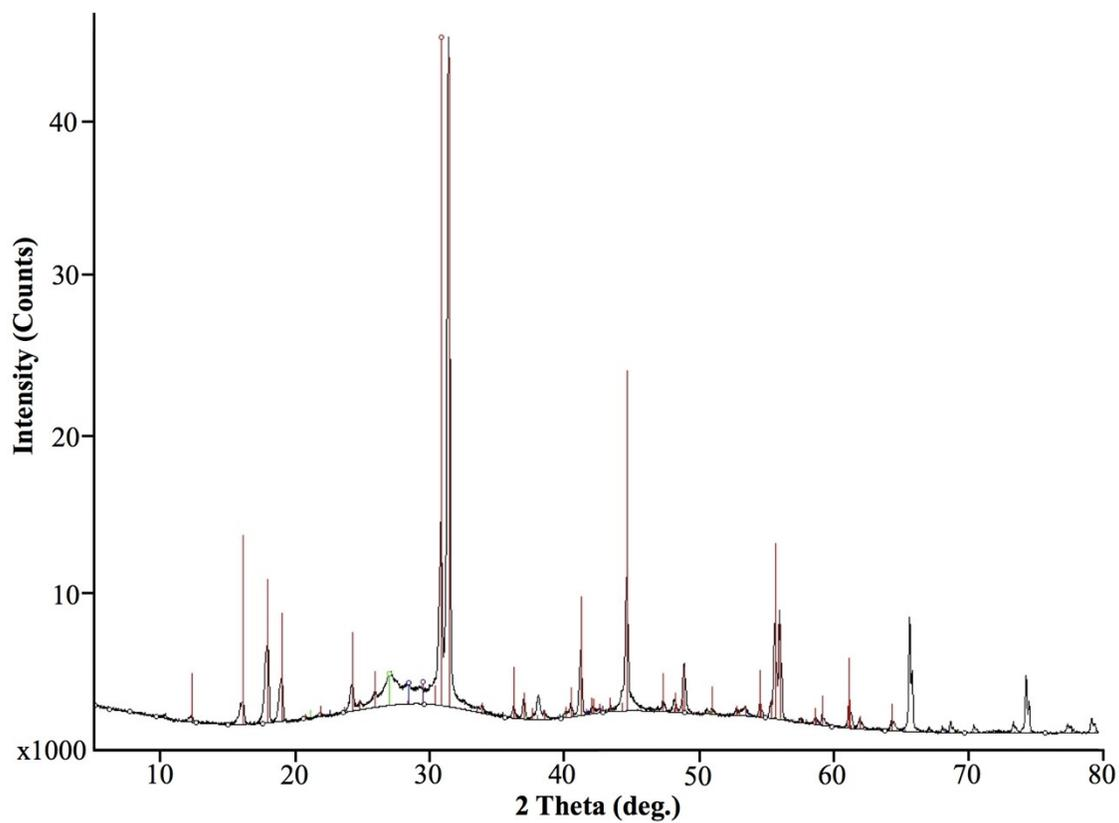
**Figure S-1.** PXRD pattern of  $\text{K}_3\text{YSi}_2\text{O}_7$  (**2**). The observed pattern is in good agreement with the calculated pattern with a small amount of three types of  $\text{SiO}_2$ . The calculated pattern is the red overlay, and the green, blue, and purple overlays are  $\text{SiO}_2$ .
