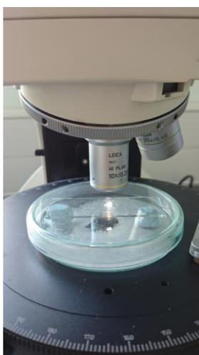
**Figure S12.** Humidity chamber setup, utilising inverted glass petri dishes. The material under investigation was suspended in a chamber above a saturated salt solution (salt + pure water). For the production of RH please see ESI Table S1 (below). All humidity's were checked with a Rotronic A/H hygrometer (temperature and RH).
