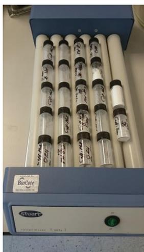
**Figure S19.** Grinding in roller mixer- no detectable difference in turnover to the co-crystal was seen in 24 hours i.e. Rate of co-crystal production is similar with or without water when levels were at ambient conditions (as per previous reports of co-crystal conversion through grinding).
