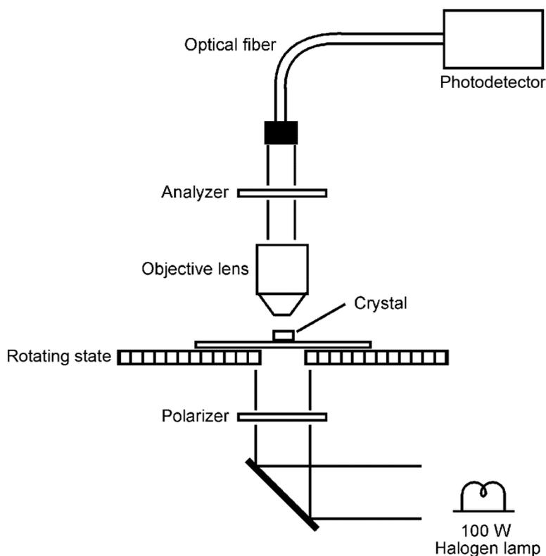
**Fig. S1** Instrumental setup for polarized absorption and fluorescence spectral measurement.
