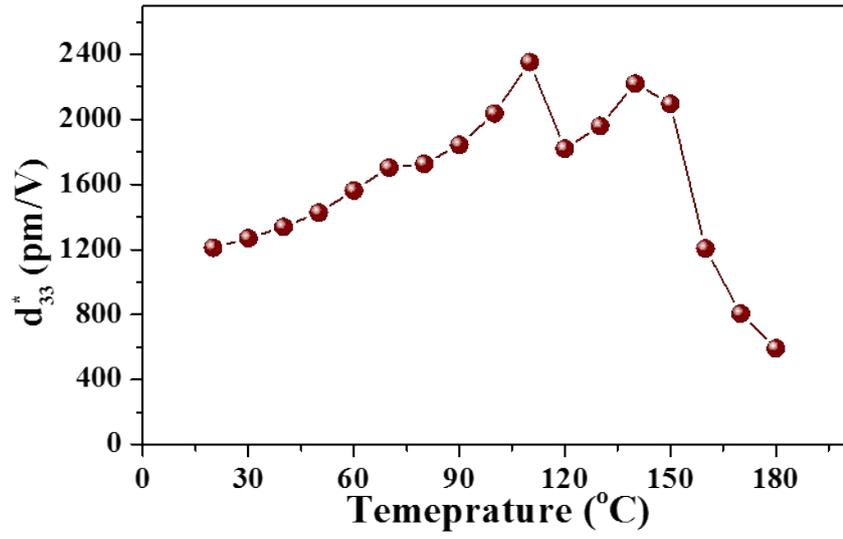
**Fig. S3.**  $d_{33}^*$  values derived from the unipolar strains as a function of temperature for the  $[001]_c$  PIN-PZ-PMN-PT single crystal.
