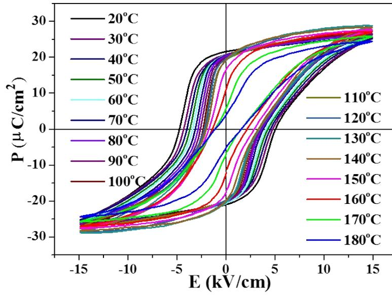
**Fig. S2.** Bipolar polarization hysteresis loop patterns of the [001]<sub>C</sub> PIN-PZ-PMN-PT single crystal at different temperature.
