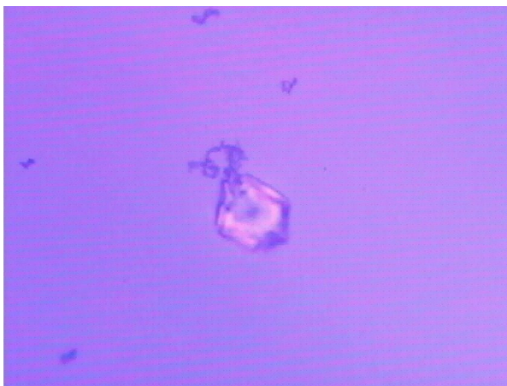
Figure ESI4. A captured micrograph of the in-situ polarized microscopic observation of NaClO 3 crystallization process from the focal spot induced by circularly polarized light laser trapping of Ag nanoparticles at the air/solution interface.
