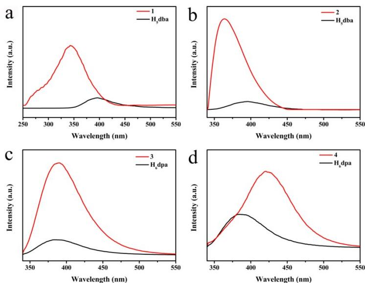
**Fig. S10.** Fluorescent emission spectra of (a) ligand  $H_5L_1$  (black), **1** (red); (b) ligand  $H_5L_1$  (black), **2** (red); (c) ligand  $H_5L_2$  (black), **3** (red); (d) ligand  $H_5L_2$  (black), **4** (red) in solid state at room temperature.
