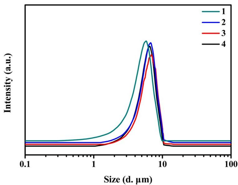
**Fig. S11.** Particle size distribution of compounds **1–4** by DLS measurement. (the average size of compounds **1–4** after dispersing in DMF solvent are 6.1, 6.7, 6.5 and 6.3  $\mu\text{m}$  in diameter, respectively)
