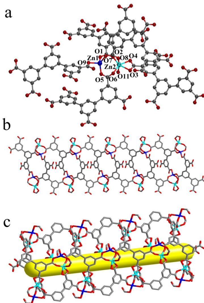
**Fig. S3.** (a) Local coordination environments of the Zn<sup>II</sup> ions in **1**. (b) 1D chain with distorted MOS in **1** along the *c* axis. (c) 1D tube in **1**. (four coordinated Zn<sup>II</sup>(1) ions are marked as blue; six coordinated Zn<sup>II</sup>(2) ions are marked as turquoise ; C, gray; O, red. All hydrogen atoms and coordinated H<sub>2</sub>O are omitted for clarity).
