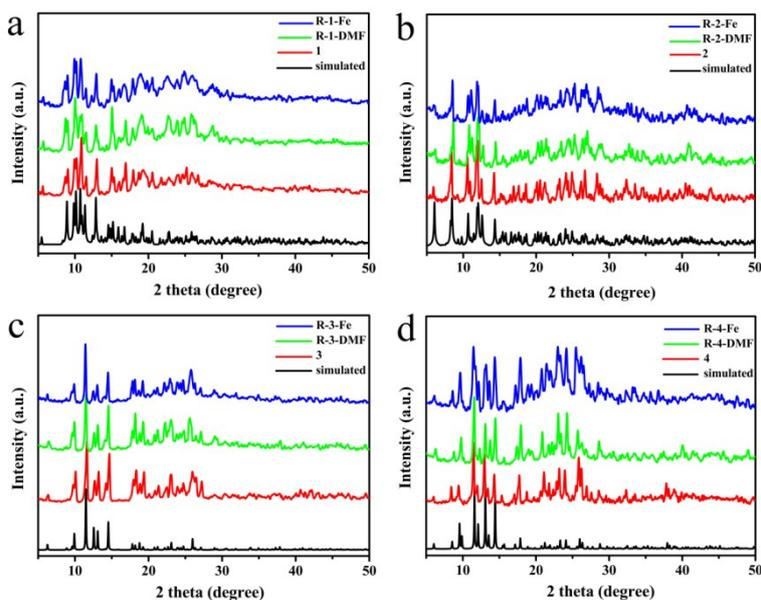
**Fig. S8.** Simulated (black), experimental (red), after recovery through centrifugation and washing with DMF (green) and after immersed in Fe<sup>3+</sup> ions solution with 1.1 mM concentration (blue) powder X-ray diffraction (PXRD) patterns for (a) **1**, (b) **2**, (c) **3**, (d) **4**.
