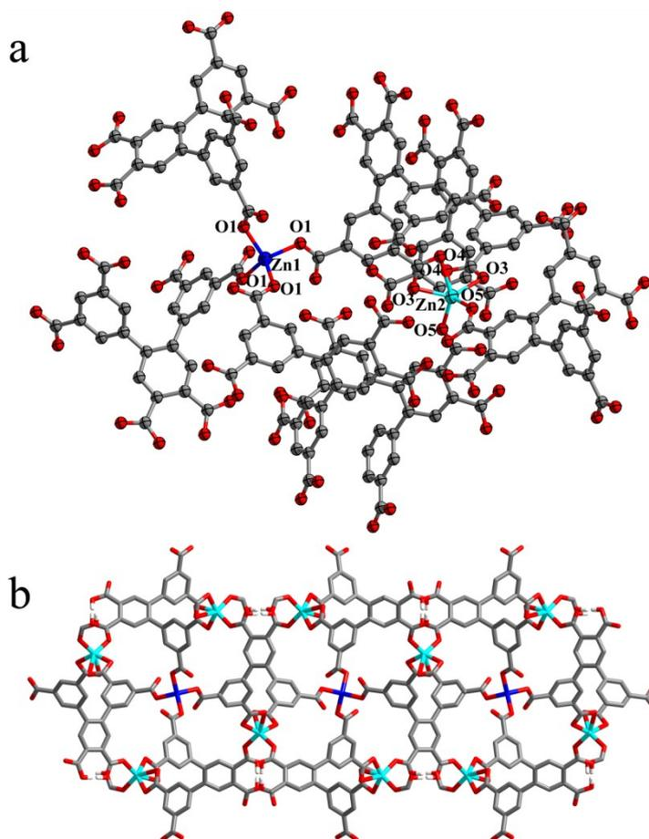
**Fig. S5.** (a) Local coordination environments of the Zn<sup>II</sup> ions in **3**. (b) 1D chain with SBUs in **3** along the *c* axis. (four coordinated Zn<sup>II</sup>(1) ions are marked as blue; six coordinated Zn<sup>II</sup>(2) ions are marked as turquoise; C, gray; O, red. All hydrogen atoms and (CH<sub>3</sub>)<sub>2</sub>NH<sub>2</sub><sup>+</sup> are omitted for clarity).
