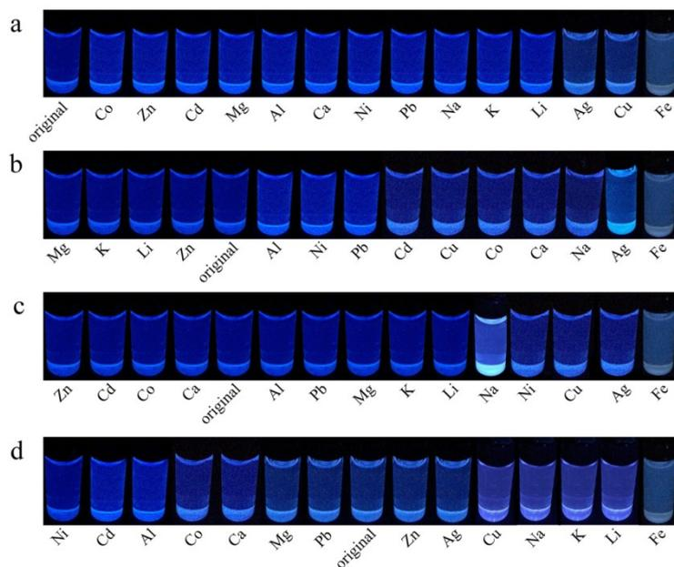
**Fig. S12.** The color change of the luminescent responses for sensing the different metal ions ( $M = \text{Na}^+$ ,  $\text{K}^+$ ,  $\text{Li}^+$ ,  $\text{Ag}^+$ ,  $\text{Mg}^{2+}$ ,  $\text{Ca}^{2+}$ ,  $\text{Pb}^{2+}$ ,  $\text{Co}^{2+}$ ,  $\text{Ni}^{2+}$ ,  $\text{Cu}^{2+}$ ,  $\text{Cd}^{2+}$ ,  $\text{Zn}^{2+}$ ,  $\text{Al}^{3+}$ ,  $\text{Fe}^{3+}$ ) in DMF solution for (a) **1**, (b) **2**, (c) **3**, (d) **4** by the ultraviolet light.
