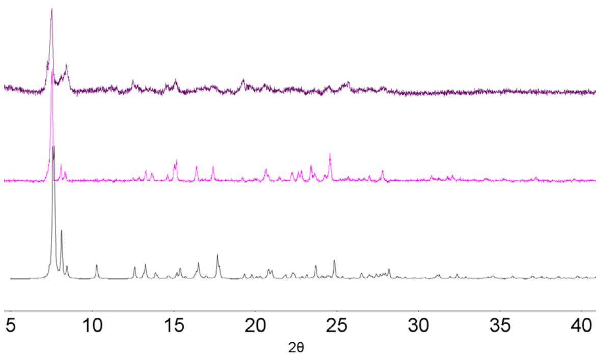
**Fig. S5.** PXRD patterns of **3**; theoretical (black), as synthesised (pink), and heated to 100°C (purple). A loss in crystallinity was observed after heating, indicating the framework is unstable toward solvent loss.
