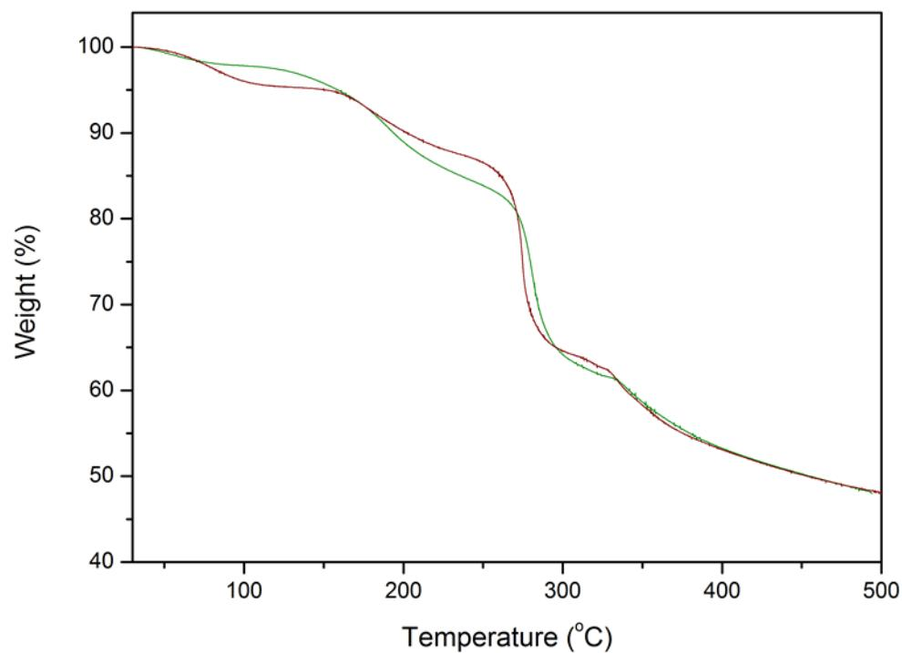
**Fig. S14.** TGA for **2** (green), and **2<sup>act</sup>** (brown) showing DMF loss from the as synthesised framework between 160 and 220°C, and the hygroscopic nature of **2<sup>act</sup>**.
