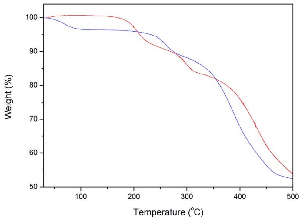
**Fig. S13.** TGA for **1-Cu** (red), and **1-Cu<sup>act</sup>** (blue) showing DMF loss from the as synthesised framework between 160 and 220°C, and the hygroscopic nature of **1-Cu<sup>act</sup>**.
