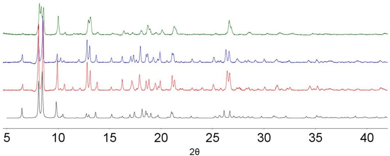
**Fig. S15.** PXRD patterns of **1** theoretical (black), **1<sup>act</sup>** (red), **1-Cu<sup>act</sup>** (blue), and **2<sup>act</sup>** (green), showing retention of crystallinity for **1** and **1-Cu**, with a minor loss of crystallinity observed for **2**.
