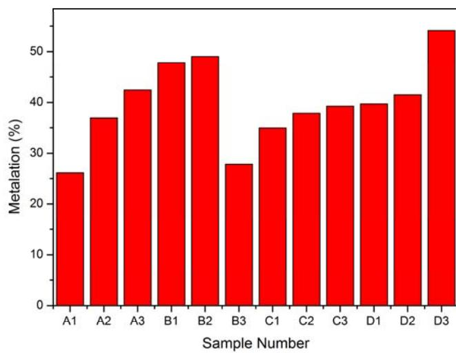
**Fig. S11.** Variation of Cu(I) metalation between samples of **1-Cu** was investigated by ICP-MS. Three individual crystals were studied from four separate vials to gives samples A1-3, B1-3 and so forth.
