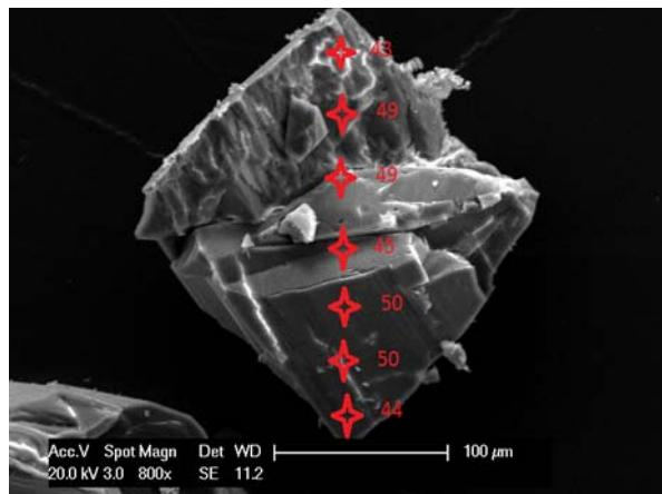
**Fig. S12.** EDX of the exposed inner face of a crystal of **1-Cu** with the metalation percentage of Cu(I) in red, and the approximate collection point shown by the red star symbol.
