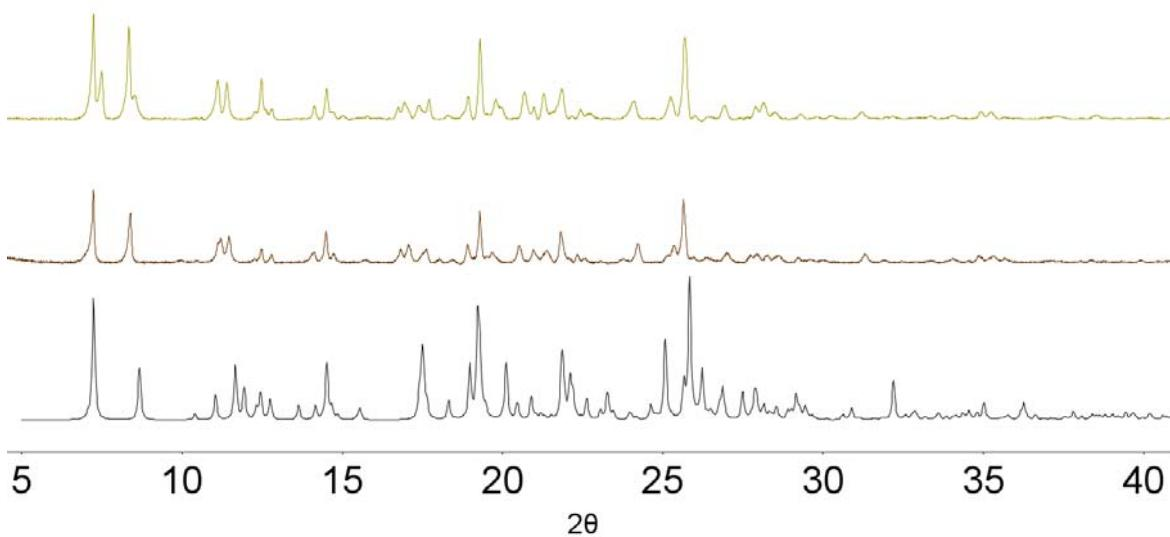
**Fig. S6.** PXRD patterns of **4**; theoretical (black), as synthesised (brown), and heated to 100°C (gold). No loss in crystallinity was observed for this samples after heating.
