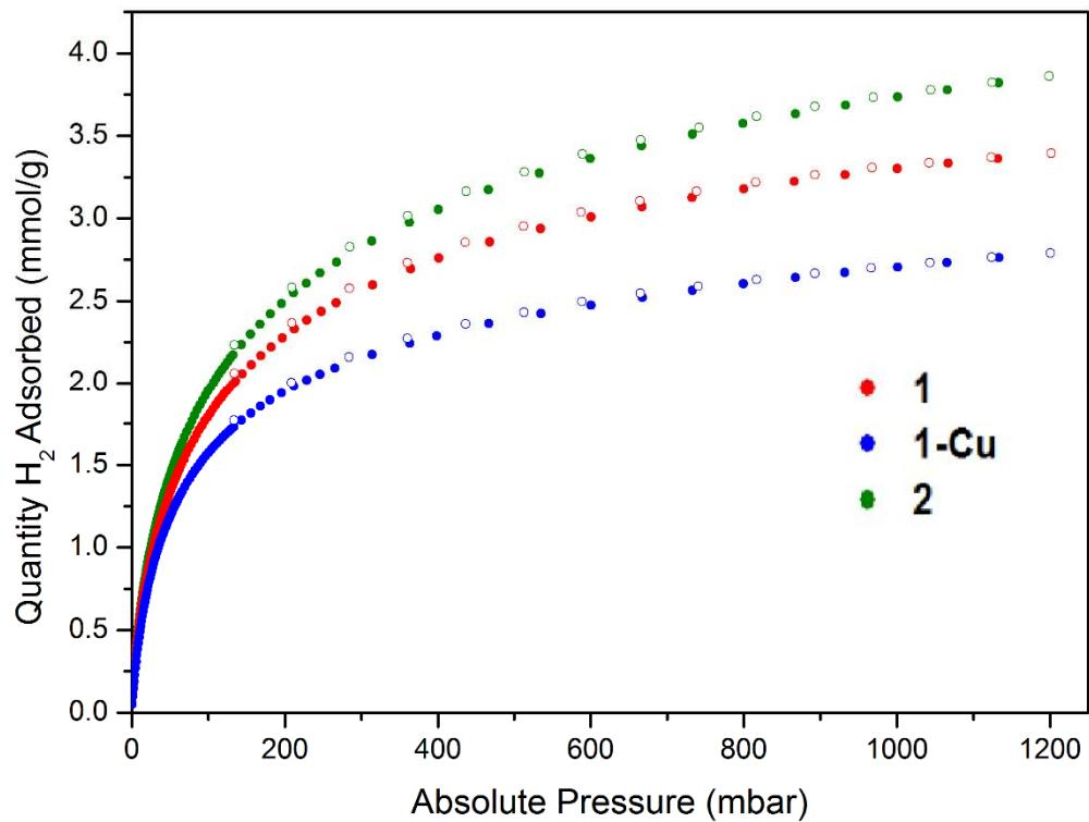
**Fig. S19.** H<sub>2</sub> adsorption isotherms for **1**, **1-Cu**, and **2** at 87 K. Filled circles indicate adsorption while empty circles indicate desorption.
