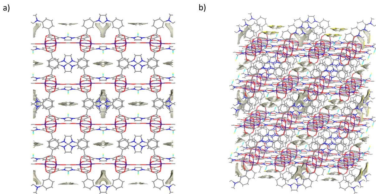
**Fig. S17.** Solvent accessible pore space in **1-CuA** viewed **a)** down the c axis and **b)** tilted off the c axis. The accessible pore volume has been greatly reduced compared to that of **1** due to the NHC-Cu-Br moiety protruding into the pore, reflecting the significantly lower BET surface area calculated ( $160 \text{ m}^2\text{g}^{-1}$ ).
