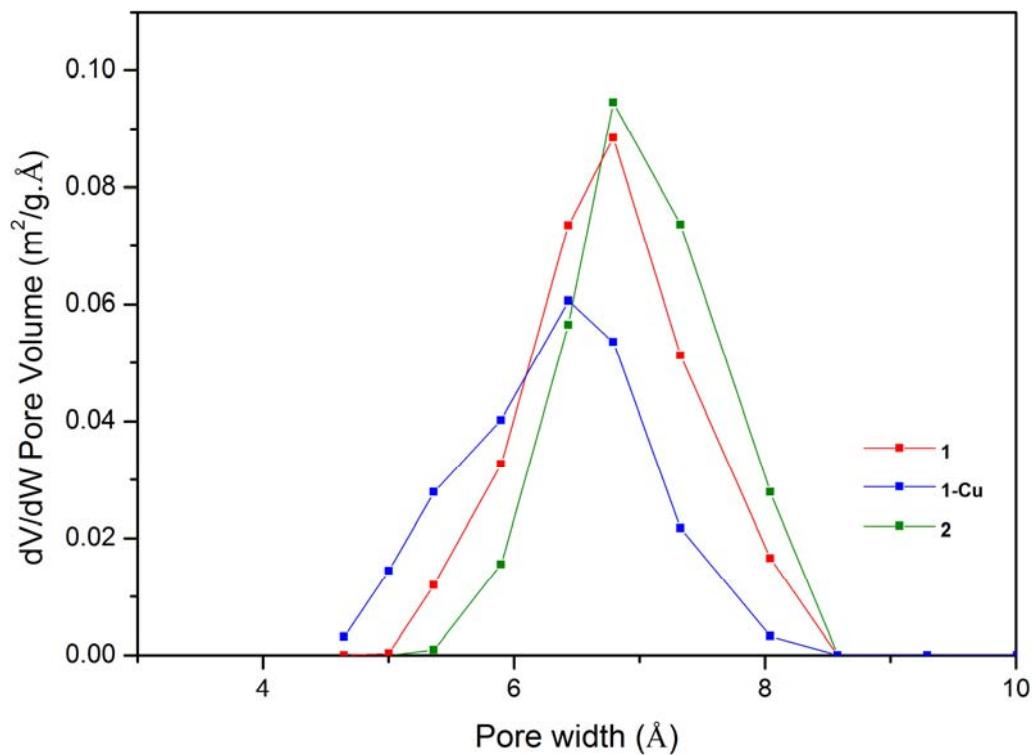
**Fig. S20.** Calculated pore size distributions for **1**, **1-Cu**, and **2**, indicating the slightly smaller pores in **1-Cu** resulting from partial metalation of the imidazolium present in **1** to form an NHC-CuBr moiety.
