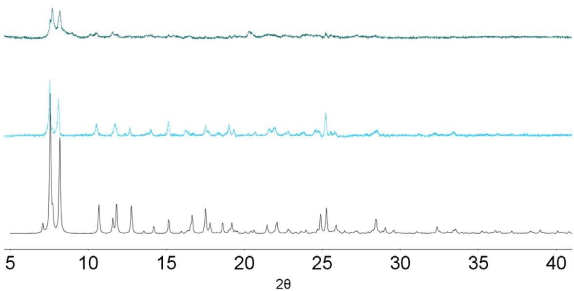
**Fig. S7.** PXRD patterns of **5**; theoretical (black), as synthesised (light blue), and heated to 100°C (dark aqua). A loss in crystallinity was observed after heating, indicating the framework is unstable toward solvent loss.
