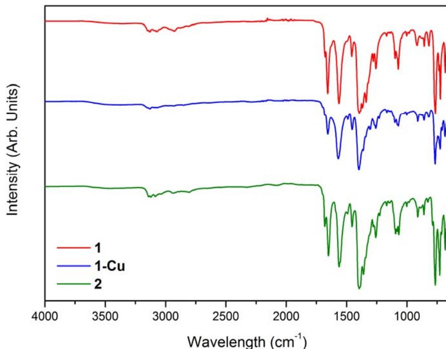
**Fig. S1.** FTIR spectra for **1**, **1-Cu**, and **2**, showing similar features due to the isomorphous nature of all three MOFs.
