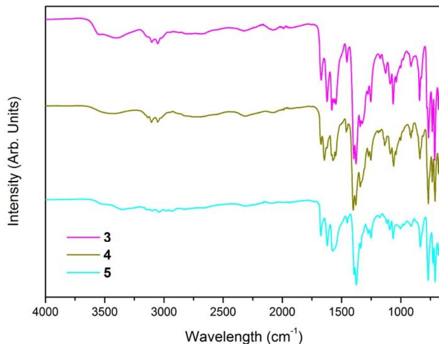
**Fig. S2.** FTIR spectra for **3**, **4**, and **5**, showing similar features due to the isostructural nature of all three MOFs.
