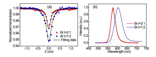
Fig S3. (a) The Z-scan results of the two perovskite QDs with different ratios of Br and I. (b) Normalized TP PL spectra of the two QDs. We can found that the TPA of the QDs with more I  $(0.061 \times 10^{-2} \text{ cm/GW})$  is better than the QD with more Br  $(0.055 \times 10^{-2} \text{ cm/GW})$ .
