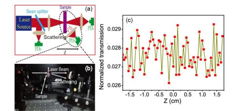
Fig. S2. (a, b) Z-scan experiment set-up:  $PD_1/PD_0$  reflects the nonlinear properties of the samples and  $PD_2/PD_0$  reflects the scattering signals. (c) Scattering results of the perovskite sample when we were carrying out the open-aperture Z-scans experiments.
