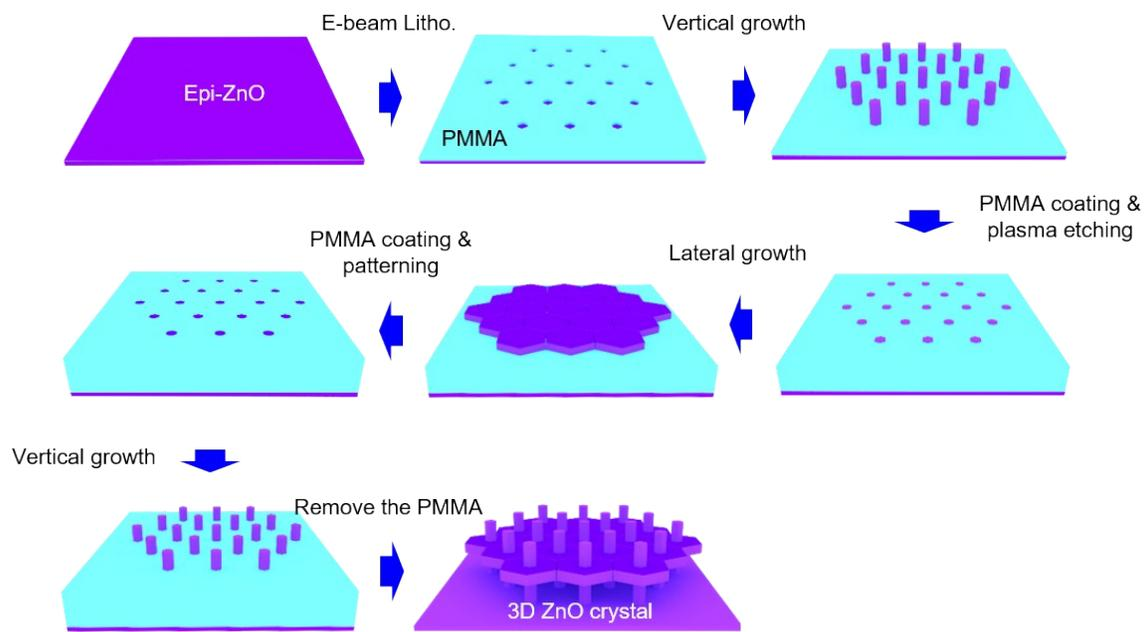
**Fig. S2** Schematic illustrating the hydrothermal process for multistage growth of 3D structures.
