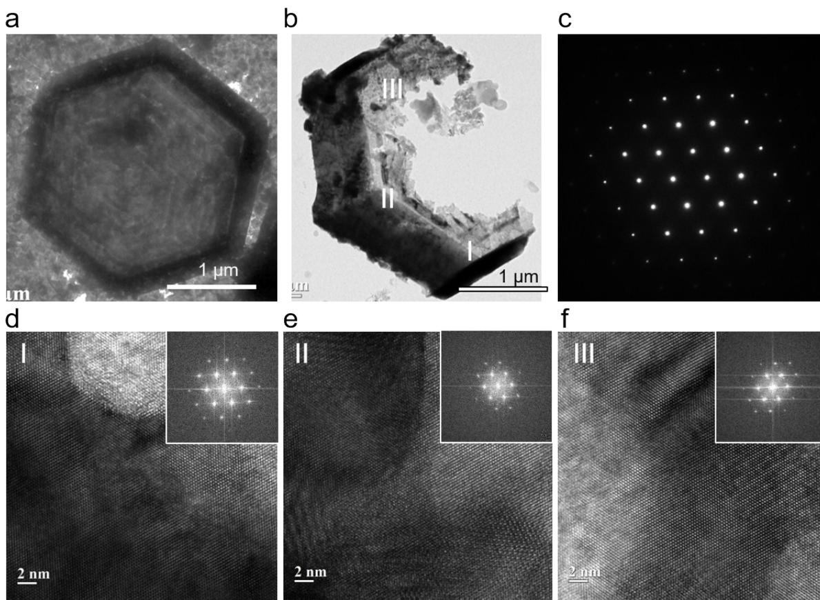
**Fig. S5** (a) low-magnification TEM images of 3D tubular structured GaN crystal that was made after etching the core ZnO hexaplate. (b, c) A fragment of GaN crystal and selective area electron-diffraction pattern showing the single crystal characteristics. (d)–(f) The high-magnification TEM images taken from regions I (d), II (e), and III (f) in the image of (b), with the corresponding FFT images (insets).
