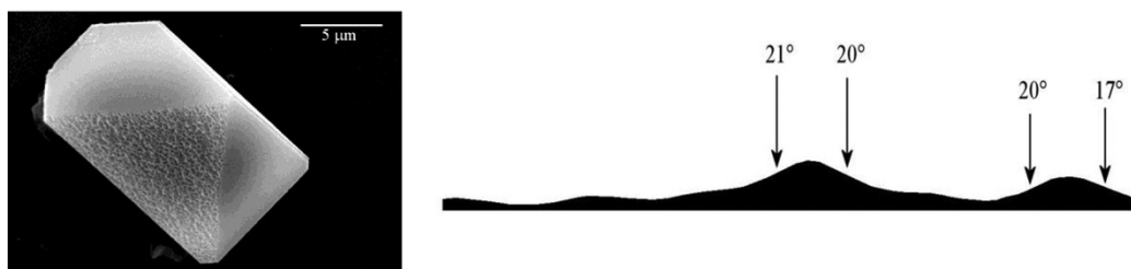
Fig. 3 Calcite crystal nucleated and grown from lithium bearing solution at high supersaturation values ( \beta \geq 37 ): the \{00.1\} faces begin to roughen (left side). The slopes of the growth hillocks on the \{00.1\} faces (right side).
