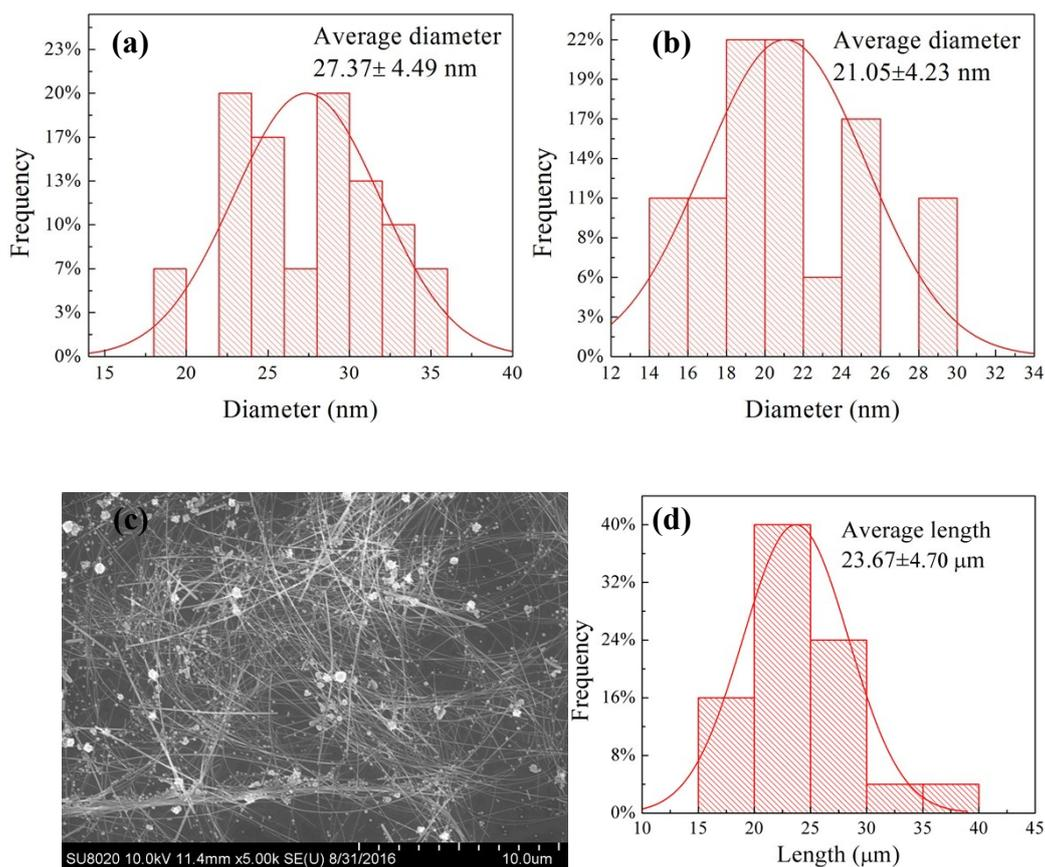
**Fig. S10.** Statistics for diameter distribution of AgNWs synthesized using only Bromine ions at (a) low and (b) high concentration. (c) SEM characterization of products and (d) statistics for length distribution of AgNWs synthesized at high concentration.
