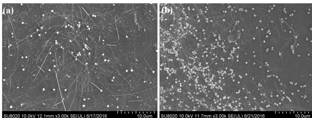
**Fig. S6.** SEM images of the products synthesized by first heating to 180°C and then cooling to 160°C with a holding time of 30 min: (a) with the addition of 1 mL H<sub>2</sub>O, (b) without H<sub>2</sub>O.
