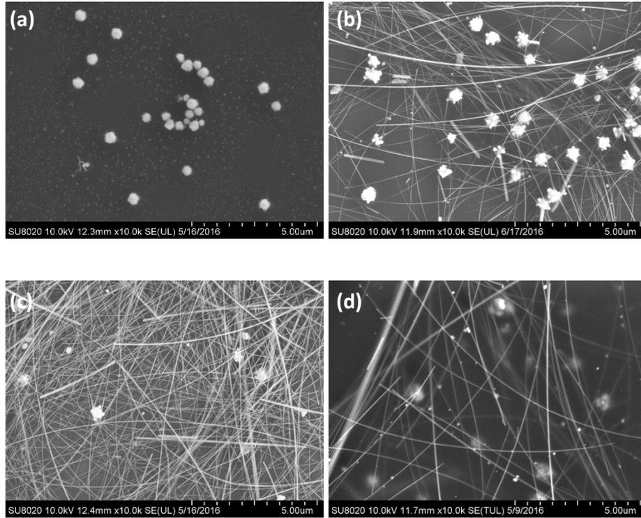
**Fig. S3.** SEM images of the product synthesized at different process temperatures for 2 h after lowering from 180°C: (a) 140°C, (b) 150°C, (c) 160°C, and (d) 170°C.
