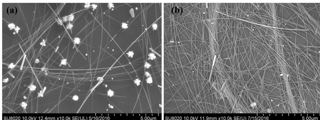
**Fig. S8.** SEM images of the products, synthesized by using different concentration of Br<sup>-</sup> and Cl<sup>-</sup> ions as well as nucleation times: (a) 100% of its original value as well as 13 min, (b) 80% of its original value as well as 17 min.
