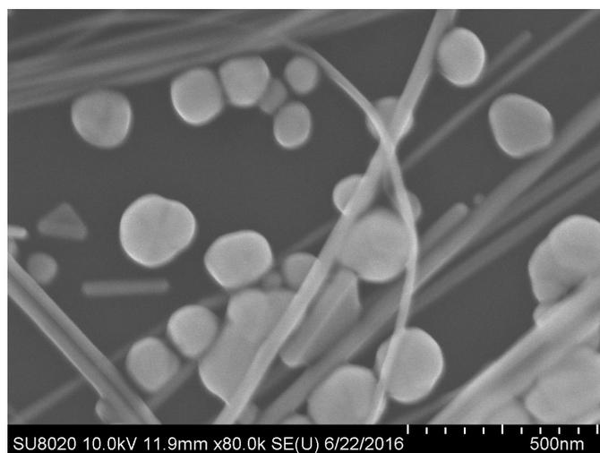
**Fig. S2.** SEM image of AgNWs together with multiple twinned particles, synthesized at constant 180°C for 1 h.
