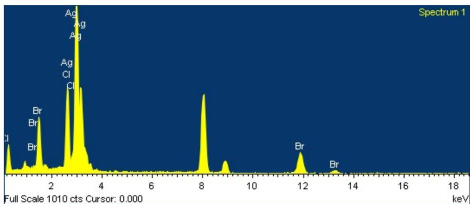
**Fig. S1.** EDX spectrum of the product by mixing the precursor at room temperature.
