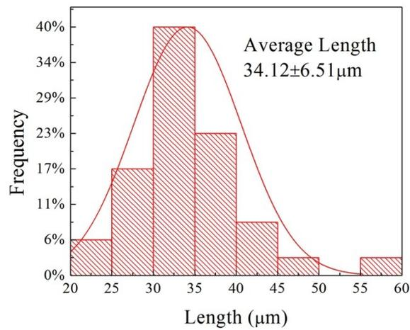
**Fig. S4.** Statistics for length distribution of AgNWs, synthesized by first heating to 180°C and then cooling to 160°C with a holding time of 2 h.
