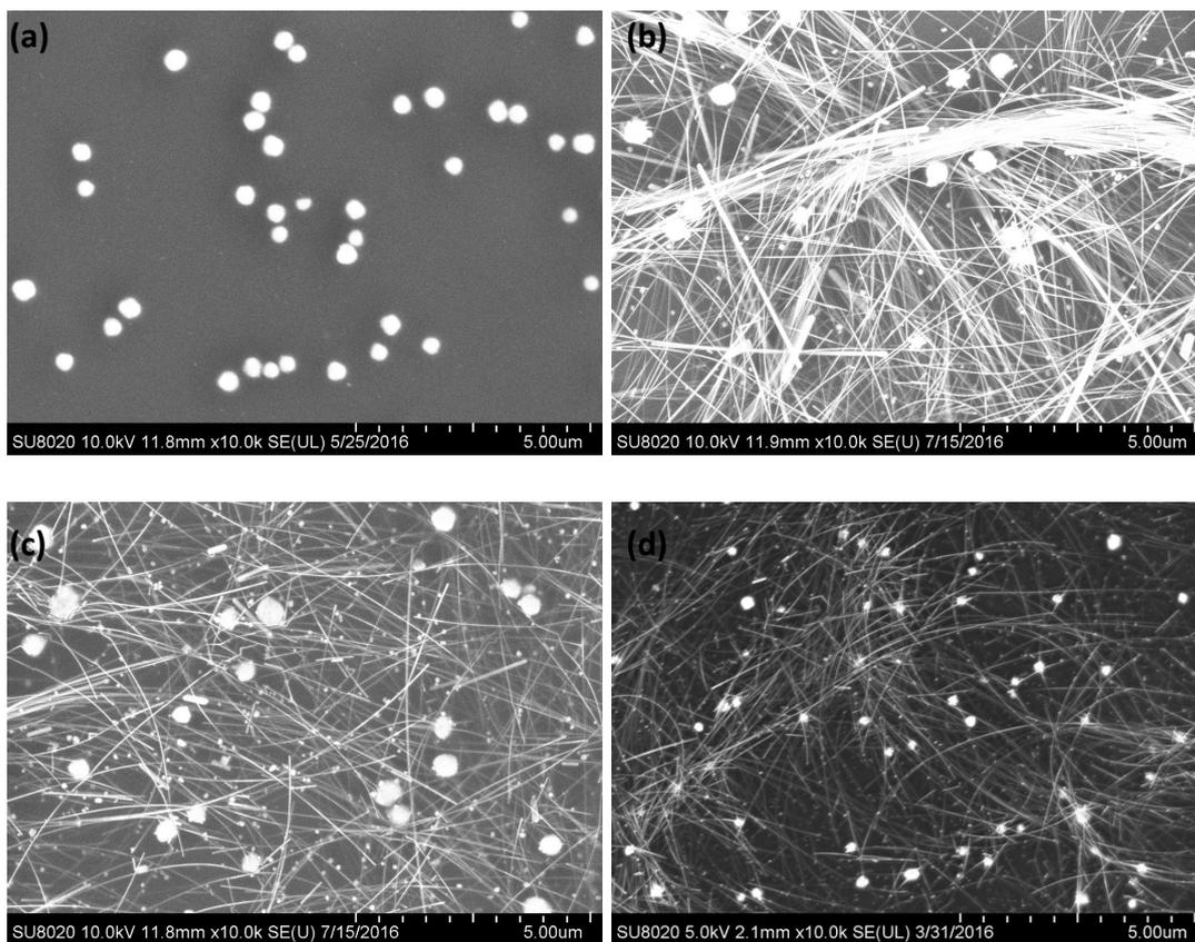
**Fig. S5.** SEM images of products synthesized for 2 h at constant temperatures of (a) 140°C, (b) 150°C, (c) 160°C, and (d) 170°C.
