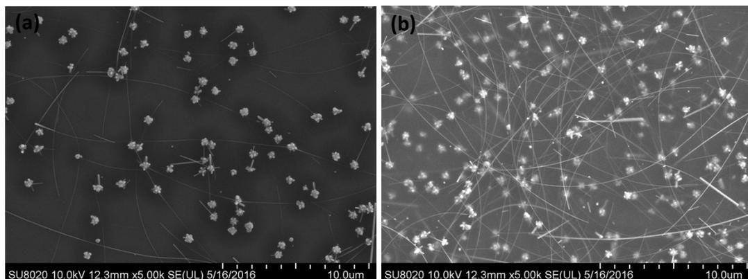
**Fig. S7.** SEM images of the product synthesized by first heating to 180°C, then cooling to 140°C with a holding time of 1 h, and then heating to 160°C with different holding times of (a) 30 min, (b) 60 min.
