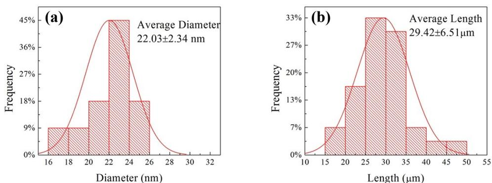
**Fig. S9.** Statistics for size distribution of AgNWs, synthesized by first heating to  $180^\circ\text{C}$  in 17 min and then cooling to  $160^\circ\text{C}$  with a holding time of 60 min: (a) diameter, (b) length. The concentration of Br<sup>-</sup> and Cl<sup>-</sup> ions was reduced to 80% of its original value.
