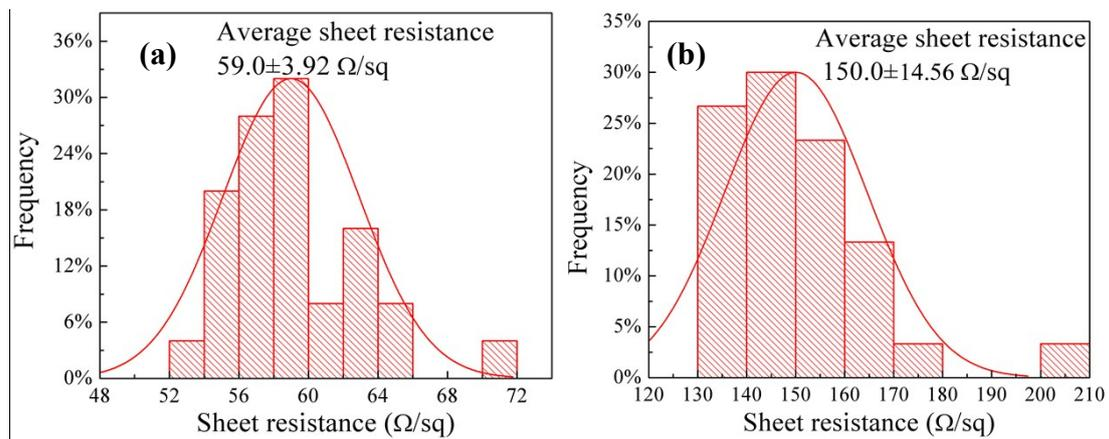
**Fig. S11.** Statistics for distribution of their sheet resistance: (a) TCFs made of AgNWs (controlled), (b) TCFs made of AgNWs (non-controlled).
