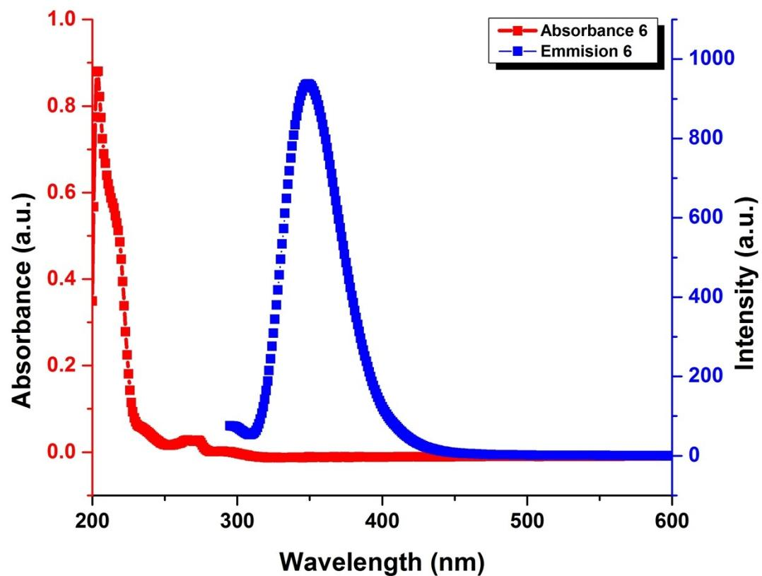
**Fig. S21** Absorbance and emission spectrum of **6**.
