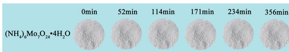
Fig. S1 Color variations of (\text{NH}_4)_6\text{Mo}_7\text{O}_{24}\cdot 4\text{H}_2\text{O} at different time (in min) under the irradiation of xenon lamp.
