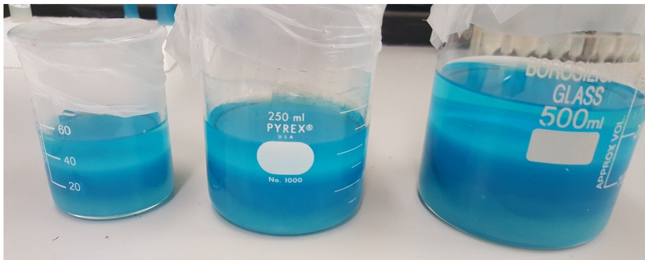
Fig. S1: Room-temperature synthesis of MOF-199 using RDF at different scales.
