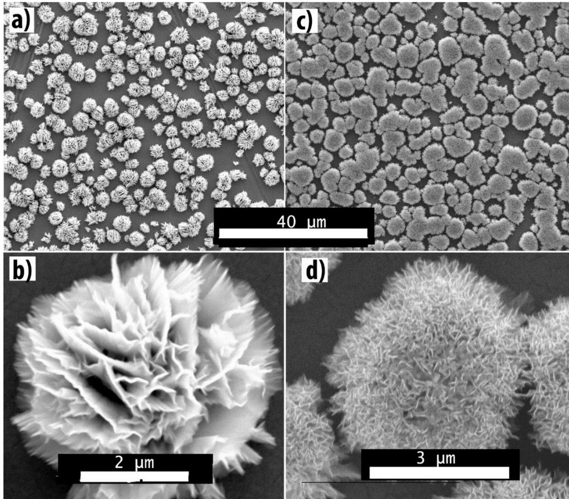
Figure S2: Comparison of microstructures corresponding to deposition at 490 °C for 60 min but using different precursor concentration solutions a) and b) a standard concentration of 0.03 mol/l corresponding to a coverage area fraction of 40% and c) and d) 0.06 mol/l which leads to a coverage area fraction of 70%. Other than the change in microflower density, the petal density is also increased when using high precursor concentration (b compared to d).
