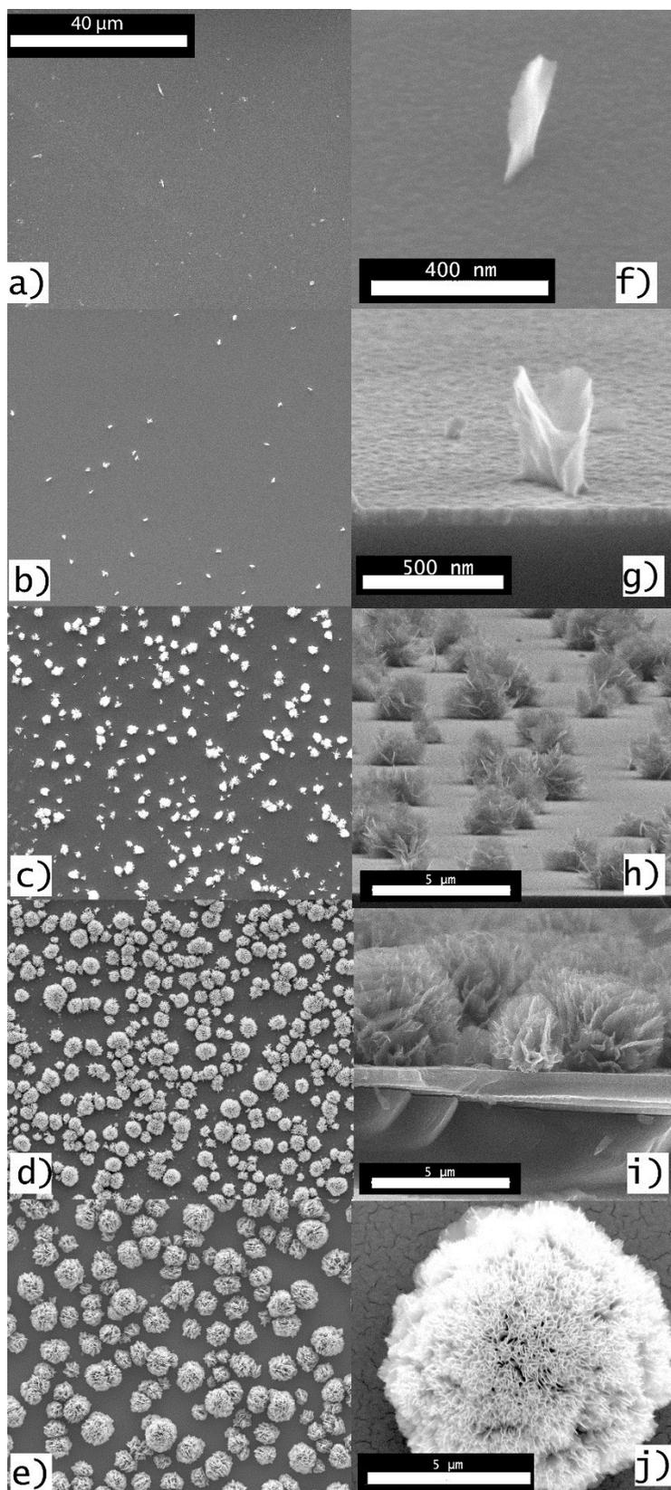
Figure S1: On left, SEM images of features developed on the surface of TiO<sub>2</sub> thin film samples for different deposition times obtained at the same magnification: a) 2 min, b) 8 min, c) 10 min, d) 60 min and f) 120 min
