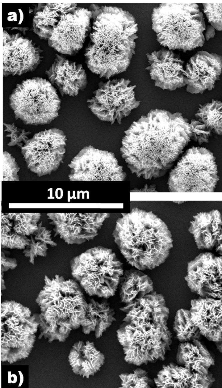
Figure S4: Top view of TiO<sub>2</sub> films deposited at 490 °C for a) 90 min in a single run and for b) 90 min but in two separate runs (60 min + 30 min).
