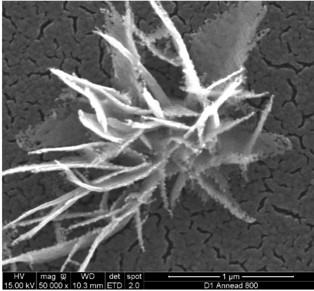
Figure S3: Top view of a sample annealed at 800 °C. The TiO<sub>2</sub> film beneath the flower presents cracks produced by shrinking during the annealing process.
