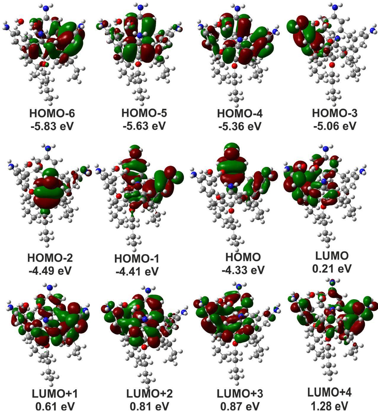
**Figure S2.** Molecular orbitals calculated at the B3LYP/6-31G\* level of theory on the crystal geometry of **1a**, together with water molecule bearing O2W and that fraction bearing O1W.
