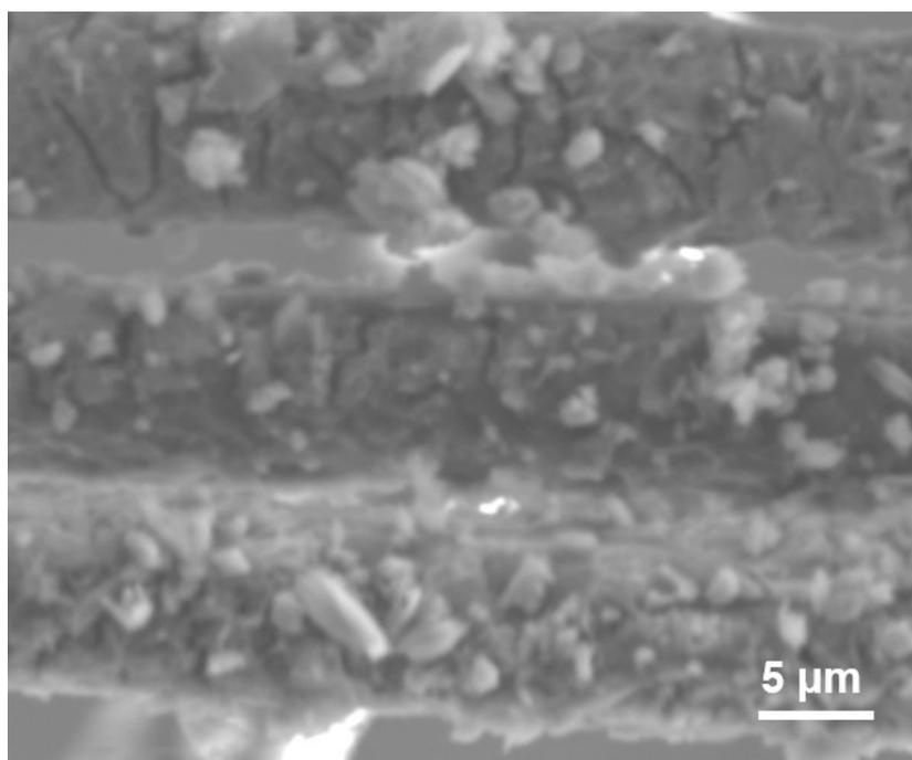
**Fig. S13.** EPMA secondary electron image of CNPCF-PPY-50 nanocomposite electrode after completing 5000 charge/discharge cycles.
