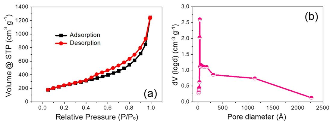
**Fig. S3.** (a)  $N_2$  sorption isotherms and (b) BJH pore-size distribution curve of CNPs.
