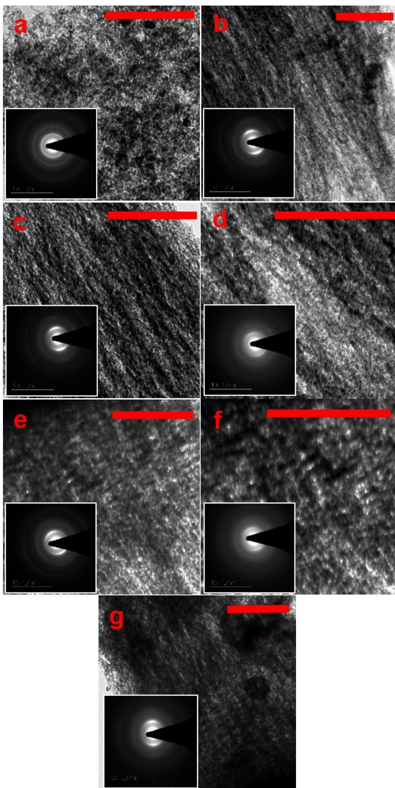
**Fig. S4.** TEM images of CNPCF-PPY-10 (a), CNPCF-PPY-20 (b), CNPCF-PPY-30 (c), CNPCF-PPY-40 (d), CNPCF-PPY-50 (e), CNPCF-PPY-60 (f) and CNPCF-PPY-120 (g) nanocomposites [inset shows their corresponding selected area electron diffraction (SAED) pattern].
