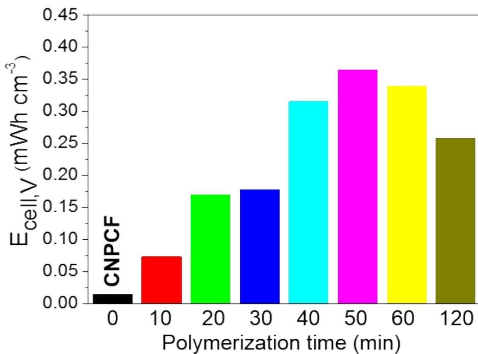
**Fig. S12.** Plot of volumetric energy density of CNPCF and CNPCF-PPY SC cells.
