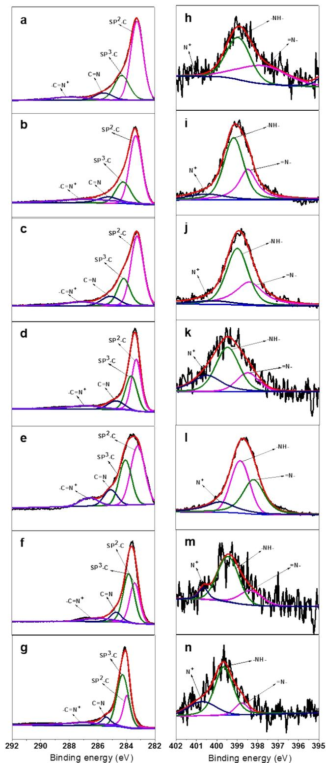
**Fig. S6.** XPS high-resolution spectra of CNPCF-PPY nanocomposites. XPS de-convolution C 1s spectra (a-g) and N 1s spectra (h-n): CNPCF-PPY-10 (a,h), CNPCF-PPY-20 (b,i), CNPCF-PPY-30 (c,j), CNPCF-PPY-40 (d,k), CNPCF-PPY-50 (e,l), CNPCF-PPY-60 (f,m) and CNPCF-PPY-120 (g,n) nanocomposites.
