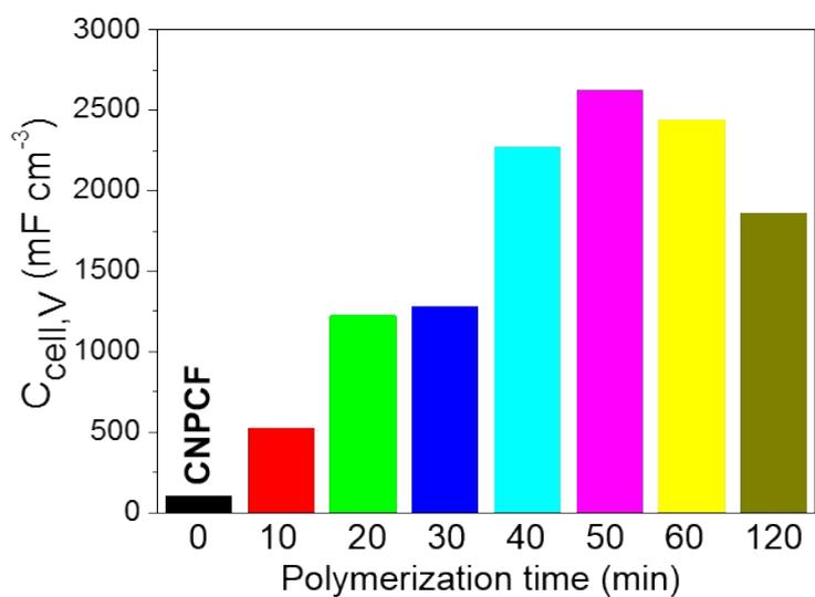
**Fig. S11.** Plot of volumetric capacitance of CNPCF and CNPCF-PPY SC cells.
