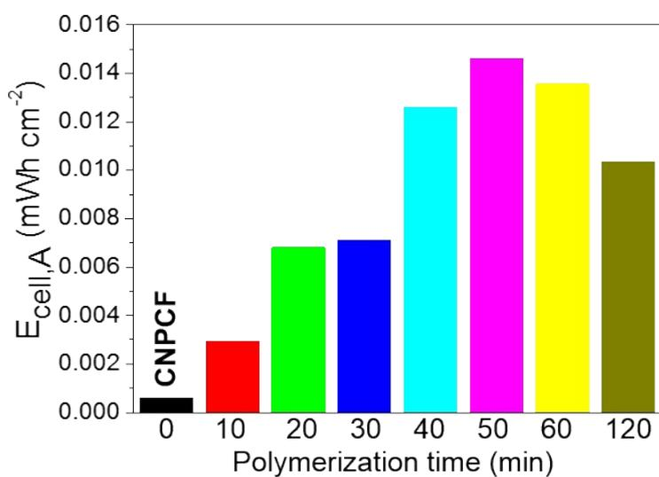
**Fig. S10.** Plot of areal energy density of CNPCF and CNPCF-PPY SC cells.
