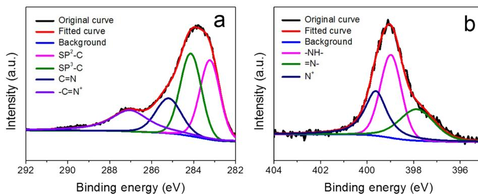
**Fig. S15.** XPS C 1s (a) and N 1s (b) de-convolution spectra of CNPCF-PPY-50 nanocomposite electrode after completing 5000 charge/discharge cycles.
