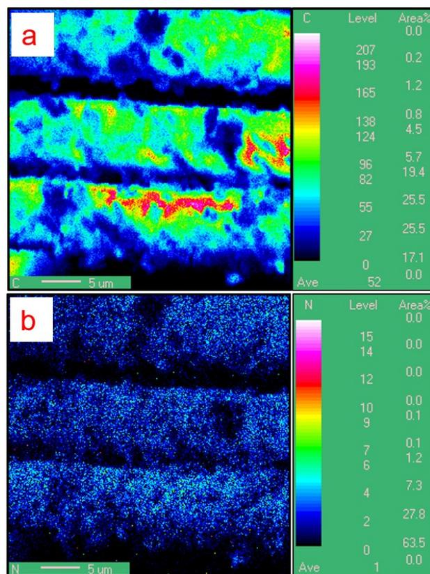
**Fig. S14.** EPMA 2D elemental mapping of CNPCF-PPY-50 nanocomposite electrode after completing 5000 charge/discharge cycles.
