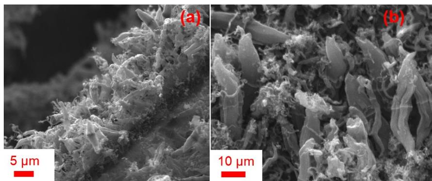
**Fig. S1.** (a,b) SEM images of CNPs synthesized on CF at different magnifications.
