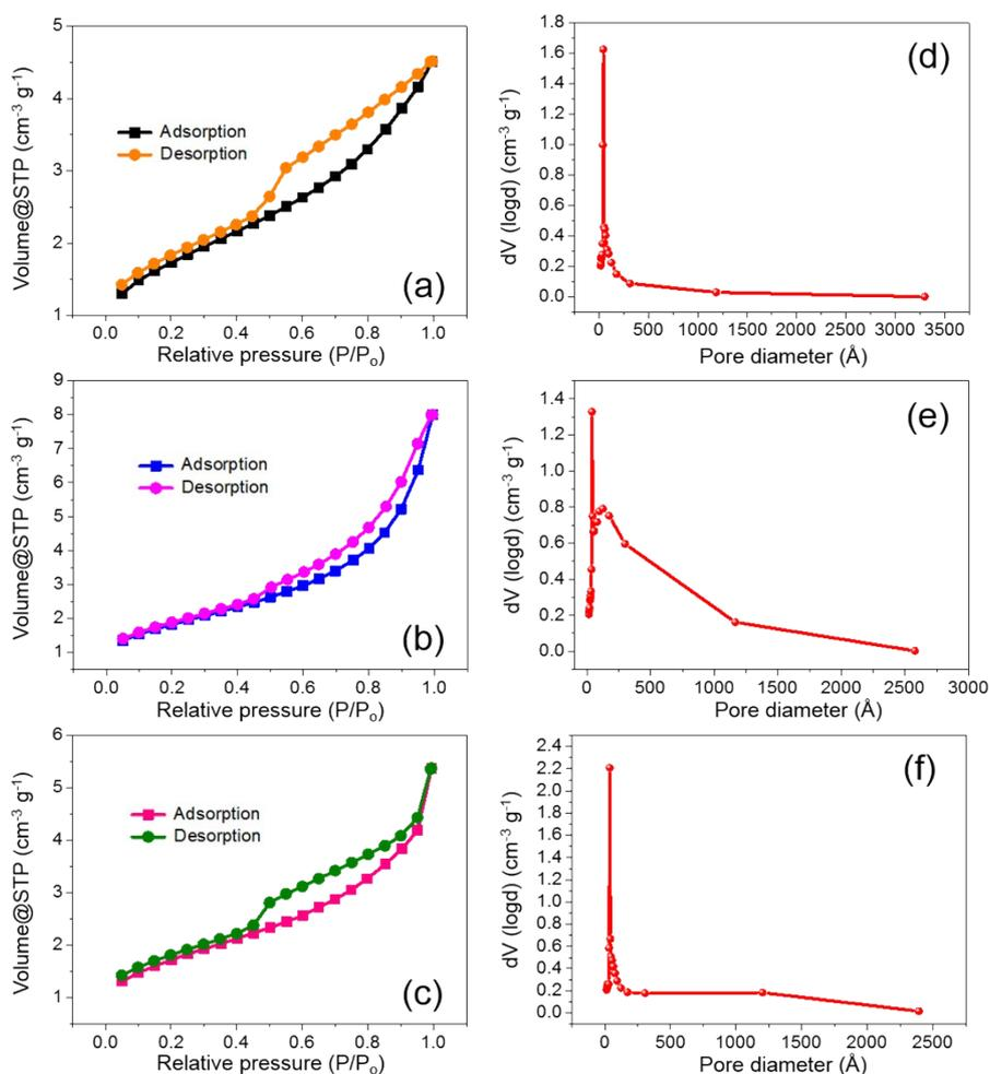
**Fig. S8.** (a-c)  $N_2$  sorption isotherms and (d-f) BJH pore-size distribution curve of CNPCF-PPY-40 (a,d), CNPCF-PPY-50 (b,e) and CNPCF-PPY-60 (c,f) nanocomposite.
