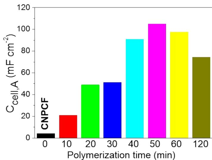
**Fig. S9.** Plot of areal capacitance of CNPCF and CNPCF-PPY SC cells.
