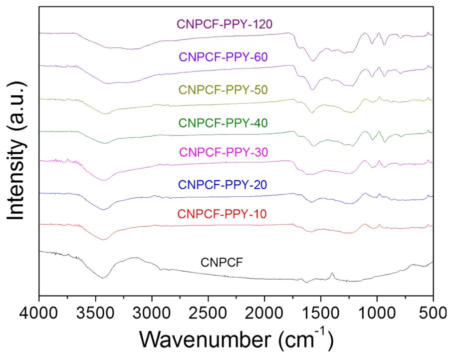
**Fig. S5.** FTIR spectra of CNPCF and CNPCF-PPY nanocomposites.
