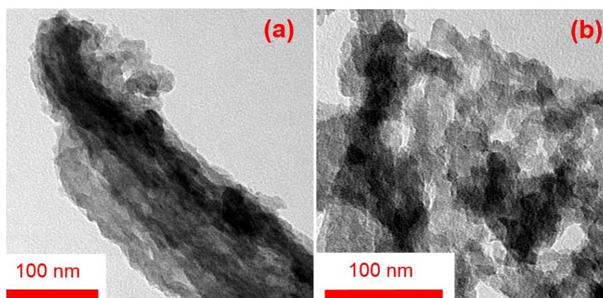
**Fig. S2.** (a,b) TEM images of the tip portion of a CNP at different magnifications.
