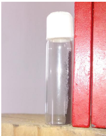
Fig. S17: Separation of Ag@Ni/Zn 0.8 Mg 0.2 O NHS catalyst by magnetic bar.
