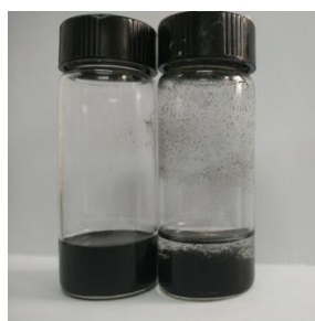
Figure S2. The images of the solution of the first step in the SOW-SWNTs dispersing process with or without DDA: the DDA (1 g) - oil (1 g) - SWNTs (1 mg) mixture (left); and the oil (1 g) –SWNTs (1 mg) mixture (right).
