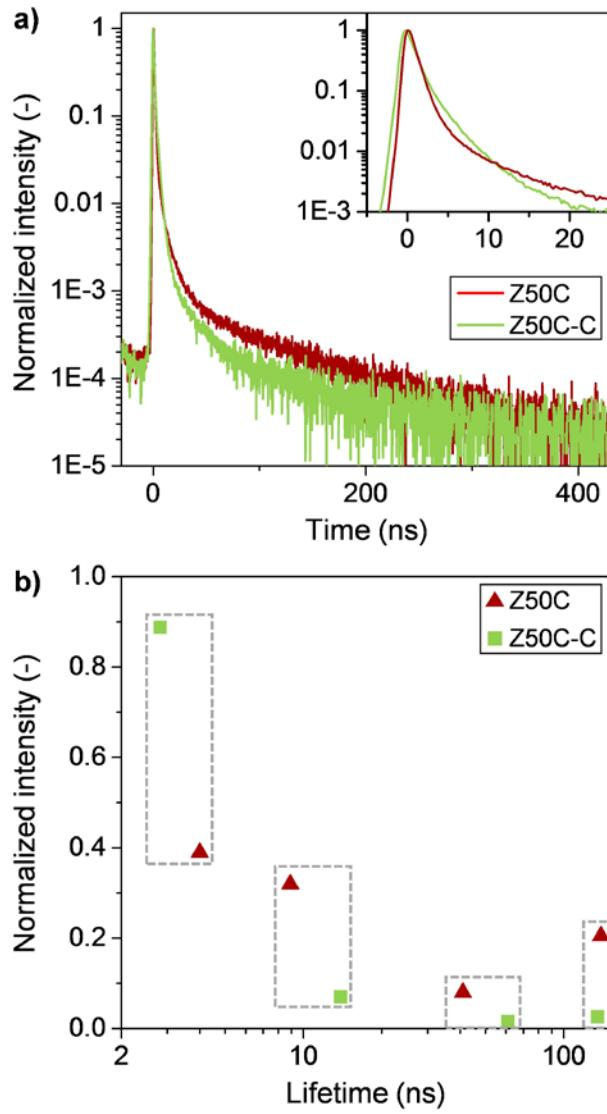
**Fig. S1** a) Normalised PALS spectra of Z50C and Z50C-C collected with the BaF<sub>2</sub> detector in the beam set-up at 5 keV and b) lifetime components and relative fractions derived using PAScual.
