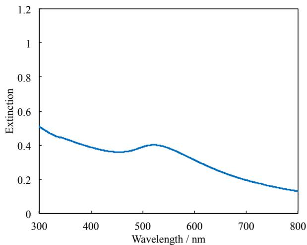
Figure S2. Extinction spectra of obtained Au nanoparticles synthesized at Au:TC:SDS = 1:3:3.
