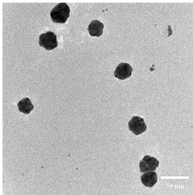
Figure S4. Large aggregates of particles ( $\sim 20$  nm) were obtained after synthesizing gold nanoparticles using SDS alone without TC.
