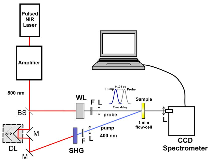
**Figure S1.** Schematic diagram of the experimental pump-probe setup. BS – beam splitter; DL – optical delay line; M – 100% reflection mirror; L, F – set of focusing lenses, neutral density and/or interferometer filters; WL – LiF or sapphire plate for generating white-light supercontinuum; SHG – BBO crystal for second harmonic generation.
