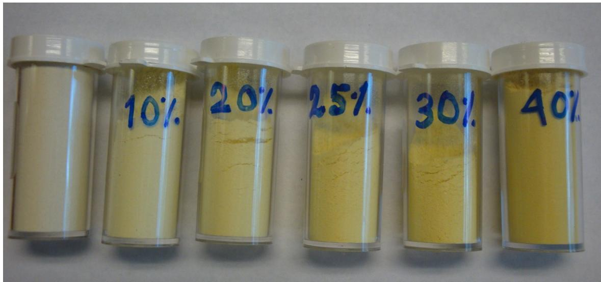
Figure S3. Visible color change in  $\text{Ce}_{1-x}\text{Sn}_x\text{O}_2$  with increasing Sn substitutions.
