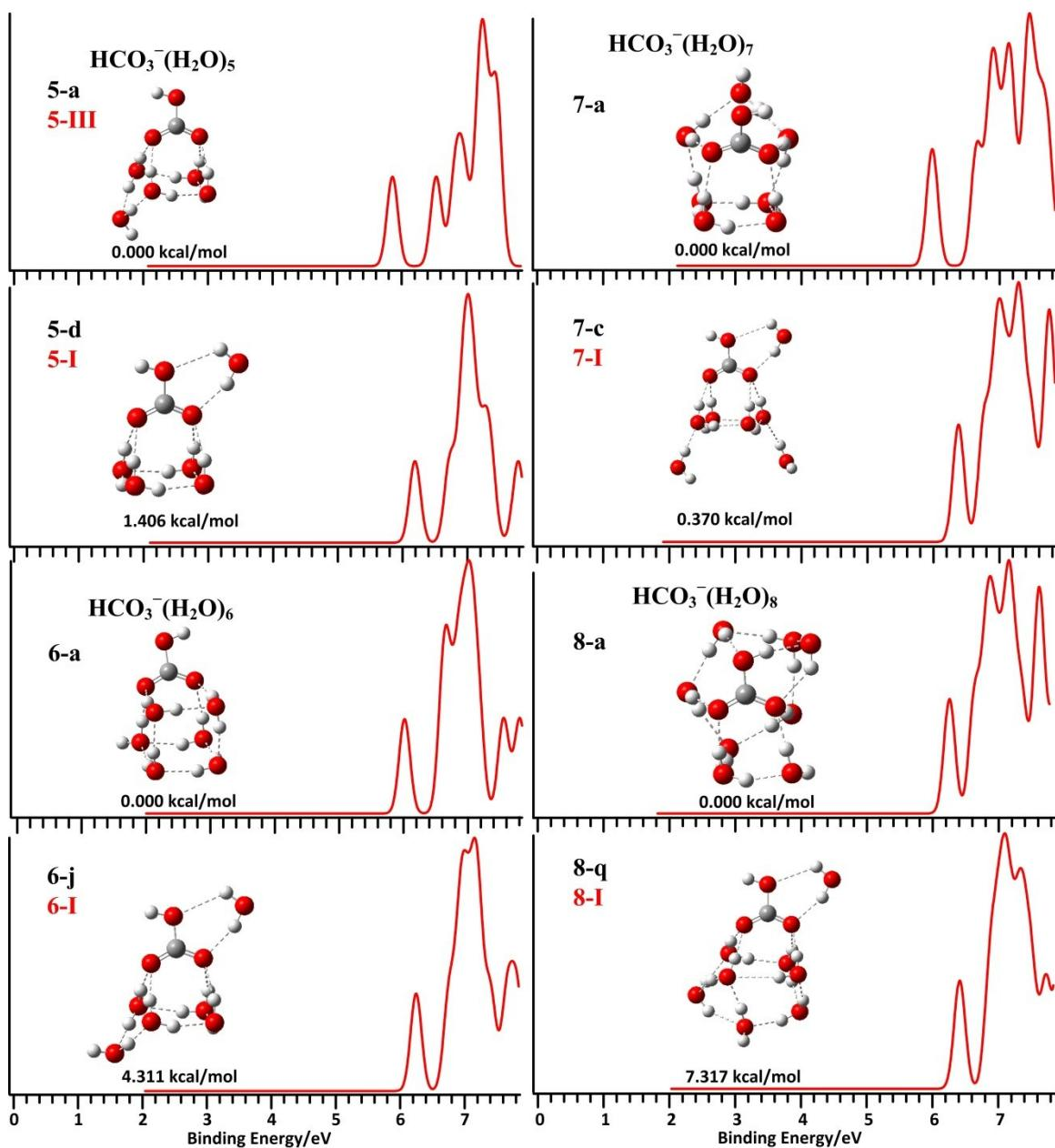
Figure S15. Simulated PES spectra of  $\text{HCO}_3^-(\text{H}_2\text{O})_n$ ,  $n=5-8$  accompany with structures, and relative energies (in kcal/mol) of the low-lying isomers at the B3LYP/6-311++(3df,3pd) level of theory, marked n-a and n-b, respectively.
