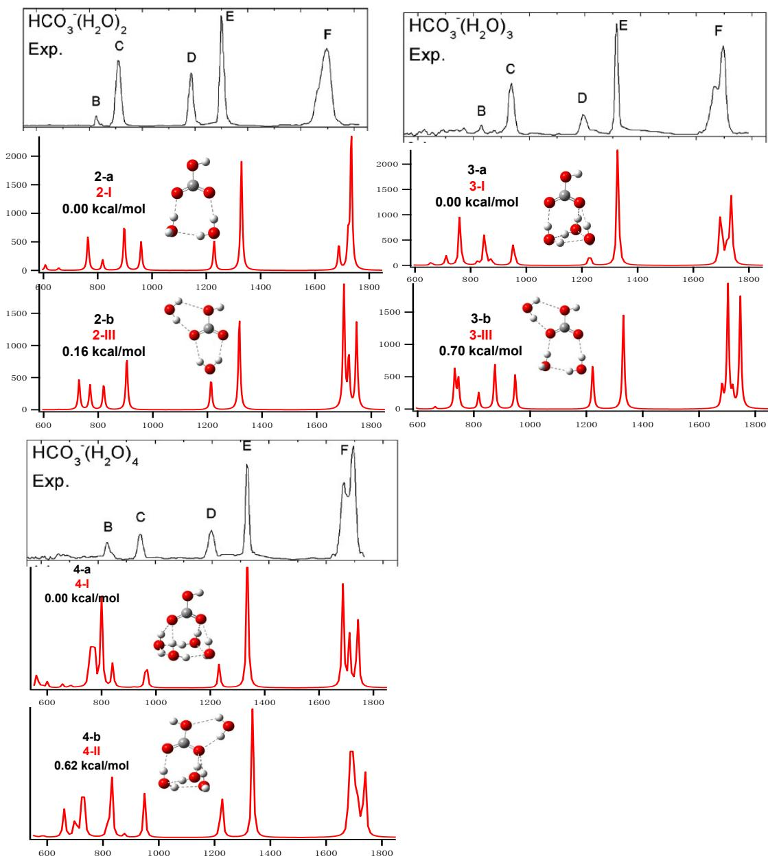
Fig. S18 Experimental (copied from Ref. 20) and theoretical infrared spectra of  $\text{HCO}_3^-(\text{H}_2\text{O})_n$ ,  $n=2-4$  clusters.
