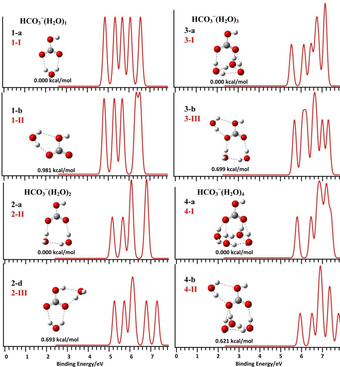
Figure S14. Simulated PES spectra of  $\text{HCO}_3^-(\text{H}_2\text{O})_n$ ,  $n=1-4$  accompany with structures, and relative energies (in kcal/mol) of the low-lying isomers at the B3LYP/6-311++(3df,3pd) level of theory, marked  $n\text{-a}$  and  $n\text{-b}$ , respectively. Any structures that are similar to those in the work of Neumark and Asmis are also labeled in red.
