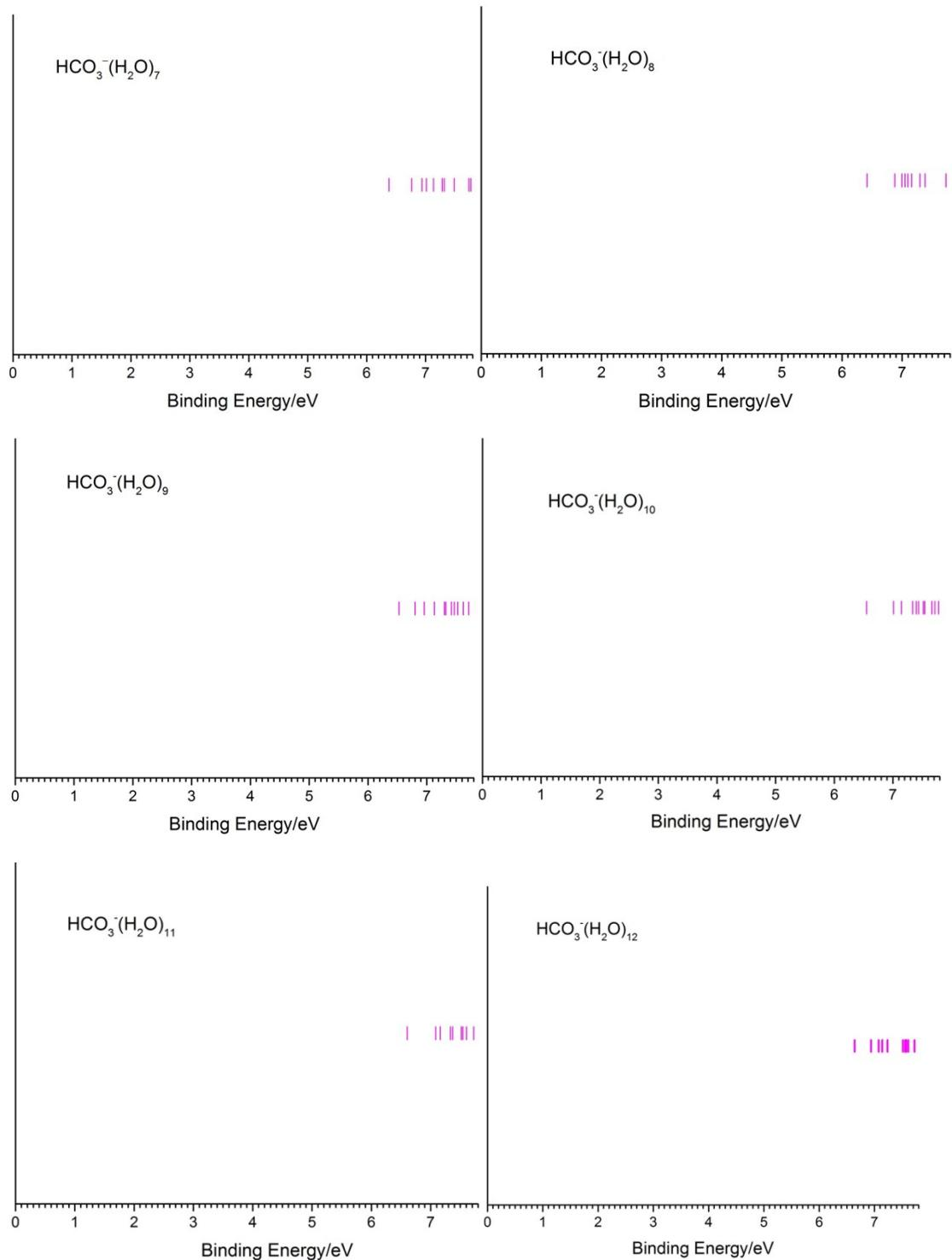
Figure S13. The stick density of states (DOS) spectra of  $\text{HCO}_3^-(\text{H}_2\text{O})_{7-12}$ .
