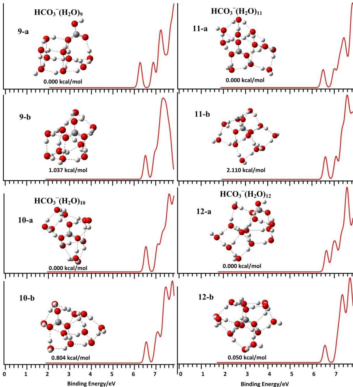
Figure S16. Simulated PES spectra of  $\text{HCO}_3^-(\text{H}_2\text{O})_n$ ,  $n=9-12$  accompany with structures, and relative energies (in kcal/mol) of the low-lying isomers at the B3LYP/6-311++(3df,3pd) level of theory, marked n-a and n-b, respectively.
