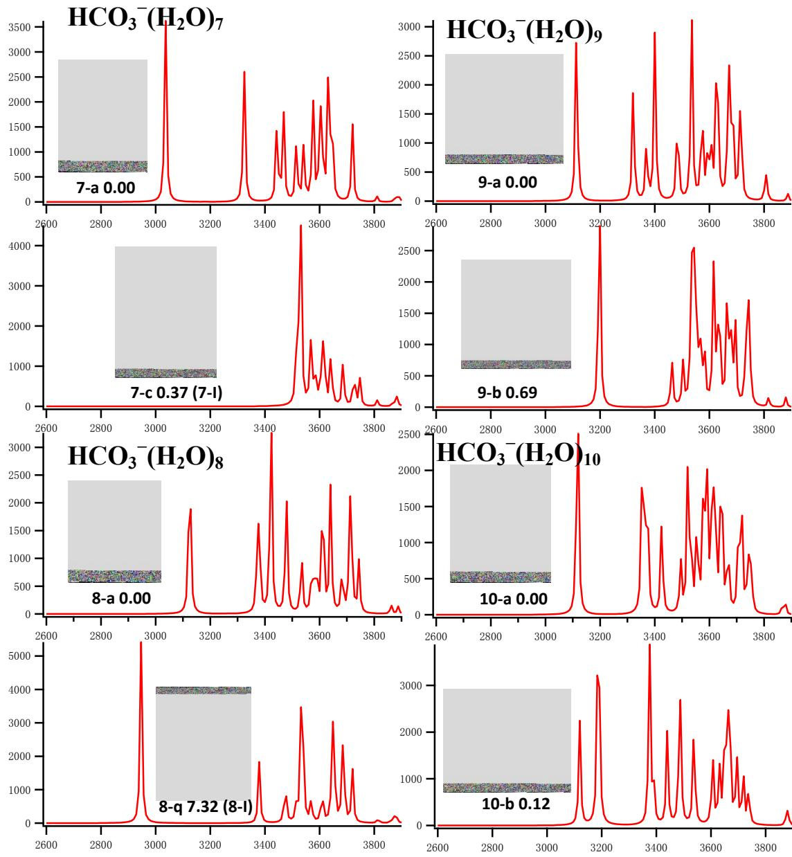
Fig. S23 Simulated IR spectra (O-H stretching mode: 2600-3900  $\text{cm}^{-1}$ ) of  $\text{HCO}_3^-(\text{H}_2\text{O})_n$ ,  $n=7-10$  clusters at B3LYP/6-311++G(3df, 3pd).
