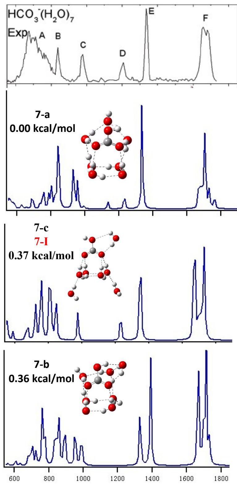
Fig. S20 Experimental (copied from Ref. 20) and theoretical infrared spectra of  $\text{HCO}_3^-(\text{H}_2\text{O})_7$  clusters.
