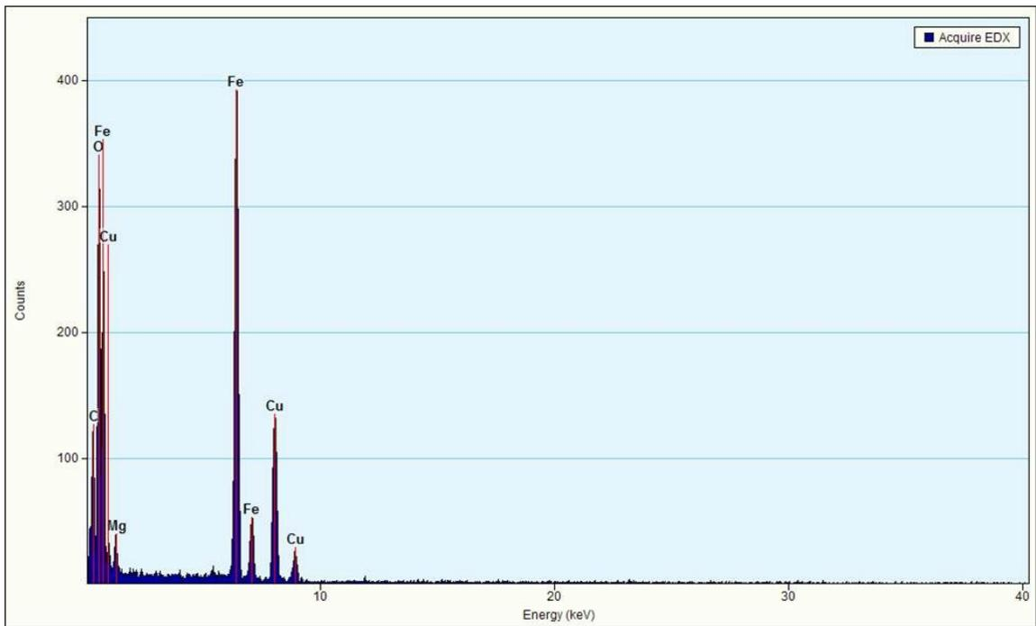
**Figure S3.** EDS of MgFe<sub>2</sub>O<sub>4</sub>. C and Cu signal originates from the sample holder.
