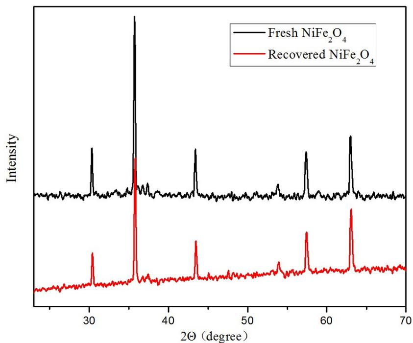
**Figure S8.** XRD of fresh  $\text{NiFe}_2\text{O}_4$  and recovered  $\text{NiFe}_2\text{O}_4$  for the chemical water oxidation.
