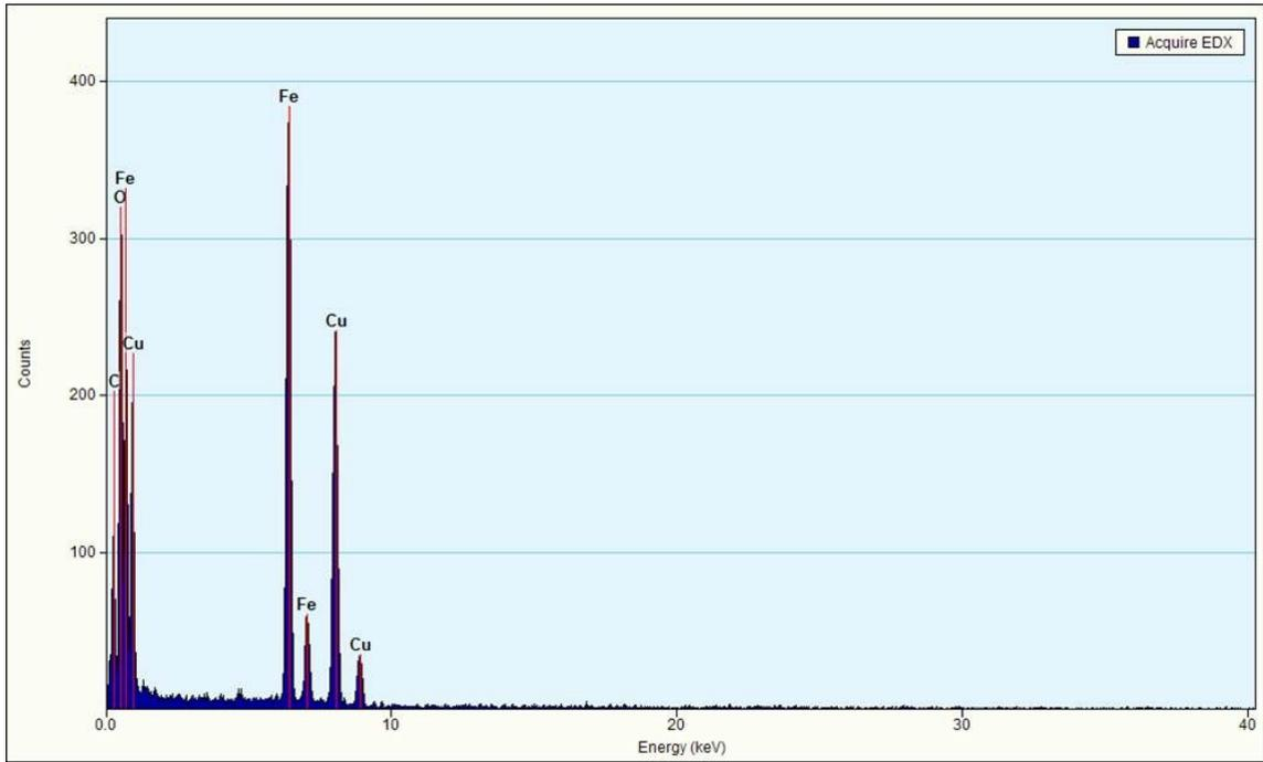
**Figure S1.** EDS of CuFe<sub>2</sub>O<sub>4</sub>. C and Cu signal originates from the sample holder and CuFe<sub>2</sub>O<sub>4</sub>.
