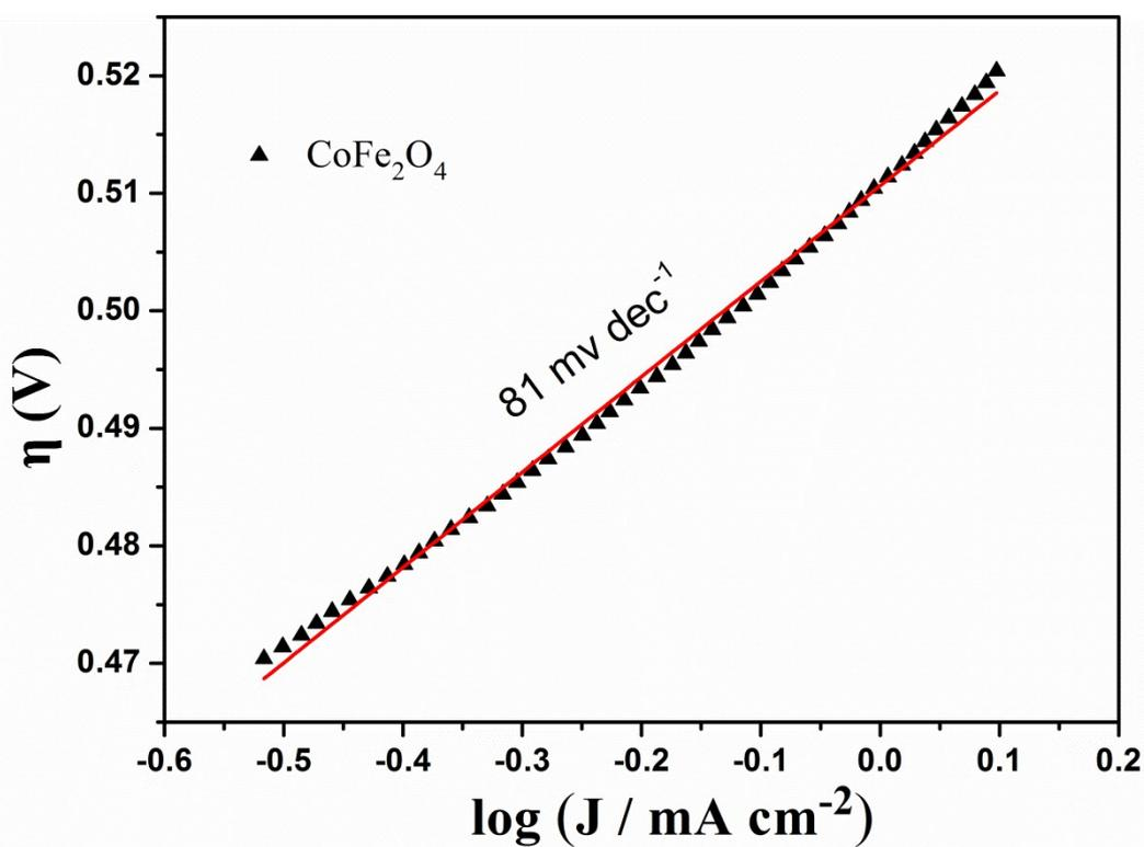
Figure S6. Tafel plot of catalyst CoFe<sub>2</sub>O<sub>4</sub>.
