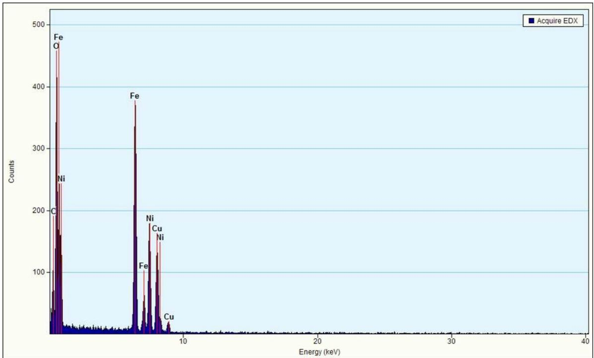
**Figure S2.** EDS of NiFe<sub>2</sub>O<sub>4</sub>. C and Cu signal originates from the sample holder.
