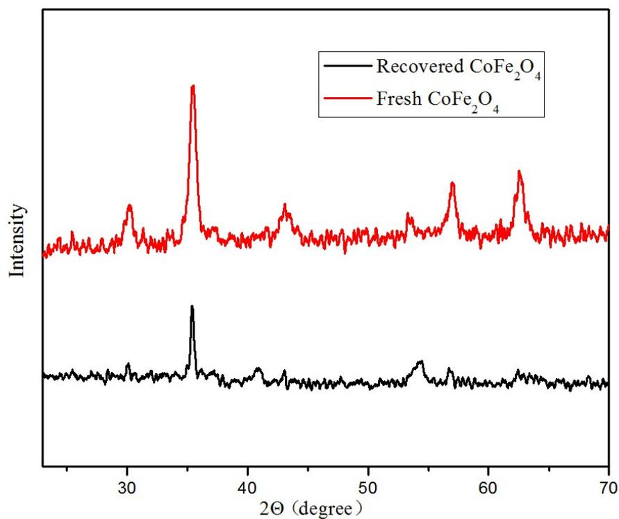
**Figure S7.** XRD of fresh  $\text{CoFe}_2\text{O}_4$  and recovered  $\text{CoFe}_2\text{O}_4$  for the photocatalytic water oxidation.
