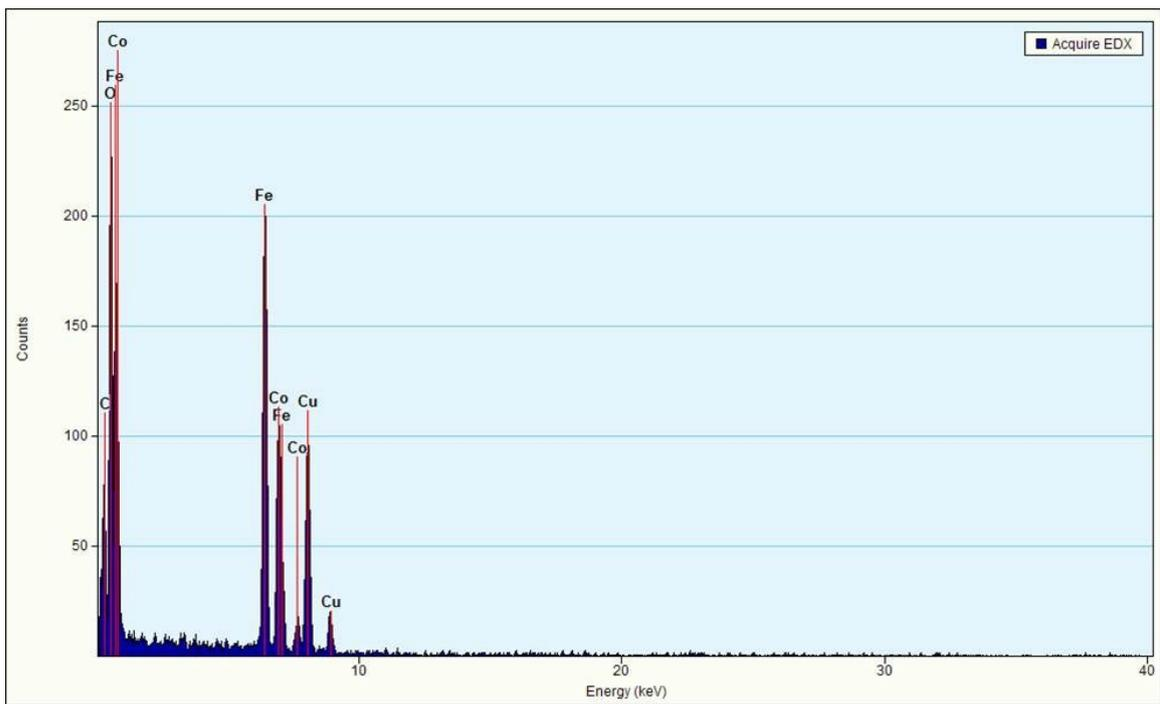
**Figure S4.** EDS of CoFe<sub>2</sub>O<sub>4</sub>. C and Cu signal originates from the sample holder.
