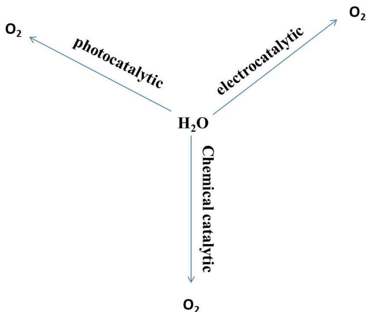
**Scheme S1.** Three driving forces commonly used in evaluating water-oxidation activities of homogeneous and heterogeneous WOCs.
