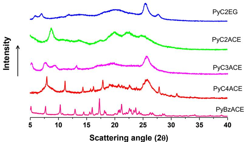
**SI Figure 10.** WAXS spectra were measured with the powdered samples of different perylene-derivatives within the range of  $2\theta = 5\text{-}40$  at  $20^\circ\text{C}$ .
