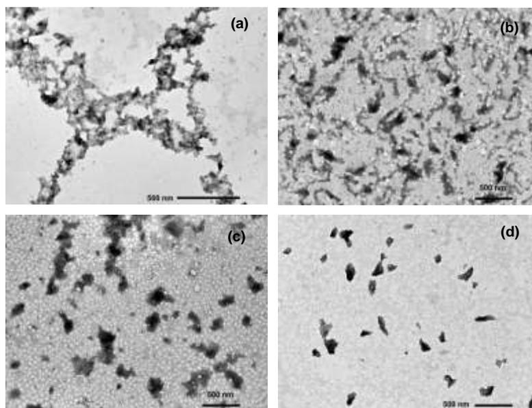
**SI Figure 16.** TEM images of ONPs –Polymer/ small molecule hybrid: Polymer/ small molecules are, (a) Pro (b) poly-lysine (c) poly-amine, and (d) arginine.
