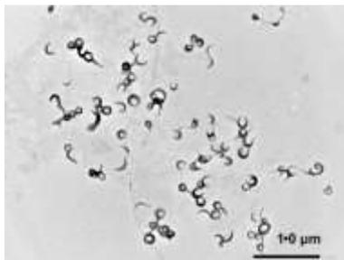
SI Figure 14. The TEM image of the ONPs was observed in the presence of  $K^+$ -ions.
