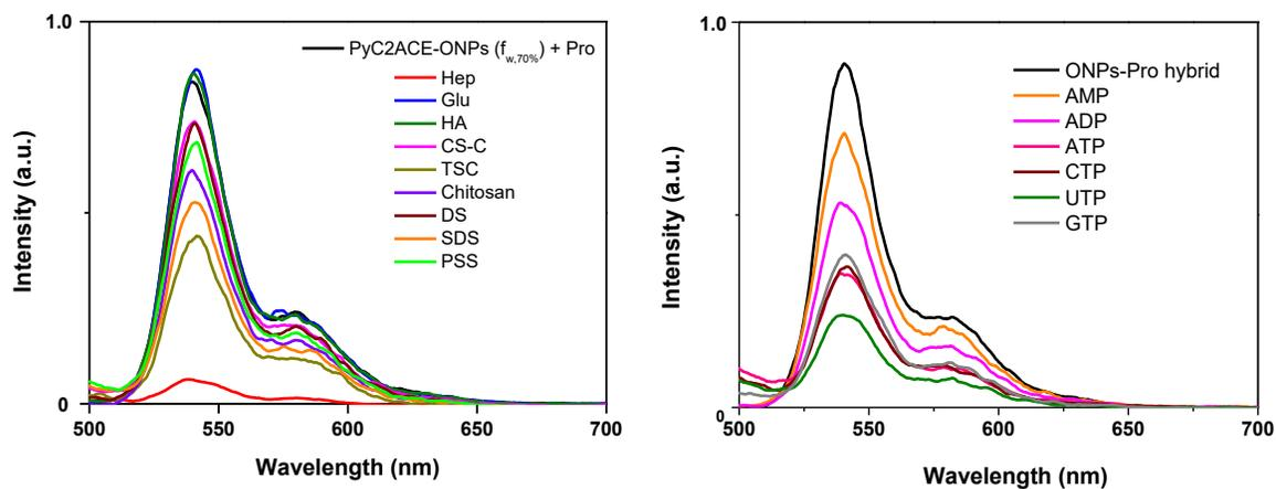
**SI Figure 18.** The FL intensity change of ONPs-Pro hybrid solution in the presence of different anionic guests (state II).
