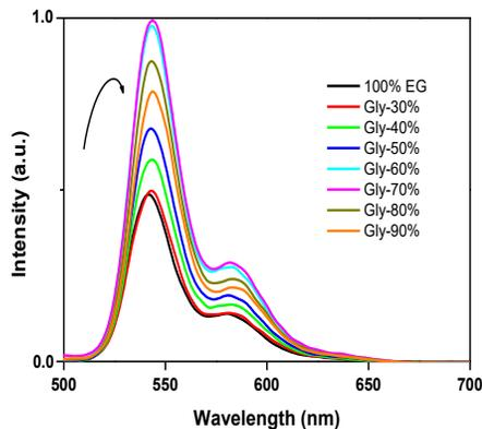
**SI Figure 12.** The relative FL intensity of PyC2ACE (10.0  $\mu$ M) was plotted with the increasing solvent viscosity by the addition of glycerol.
