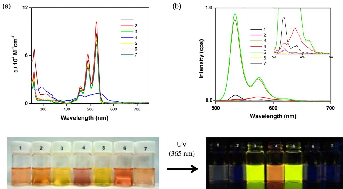
**SI Figure 1.** (a) Absorbance, and (b) fluorescence spectra of the synthesized ACE-derivatives in chloroform at 10.0  $\mu\text{M}$  concentration, and 20  $^{\circ}\text{C}$  temperature [inset (a): Zoomed FL graph]. (below): The visual images of the solutions in  $\text{CHCl}_3$  under normal light and under UV light at 365 nm. [Compounds: (1) PyC2ACE, (2) PyC2EG, (3) PyC3ACE, (4) ClPyC3ACE, (5) PyC4ACE, (6) PyBzACE, and (7) PyC2DMA]
