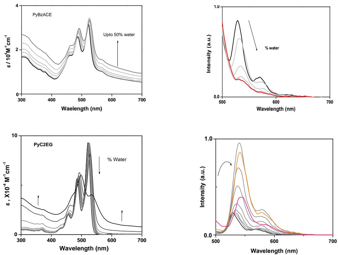
**SI Figure 4.** Absorbance (left) and fluorescence (right) spectral change was monitored against the solvent ratio change (water-THF) in a homogeneous solution of perylene derivatives at a constant concentration of  $10.0 \mu\text{M}$  and at  $20^\circ\text{C}$ .
