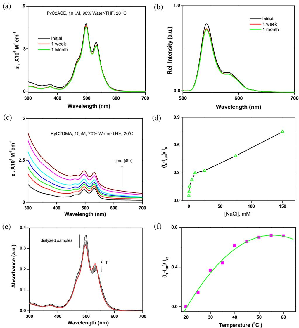
**SI Figure 9.** (a-b) Absorbance and FL spectra evaluation of the PyC2ACE ONPs from initial to 1 month, (c) Absorbance spectra of PyC2DMA in  $f_{w,70\%}$  over 4 hrs., and (d-f) Absorbance and relative FL spectra of PyC2ACE in  $f_{w,90\%}$  in presence of salt and temperature as external stimuli.
