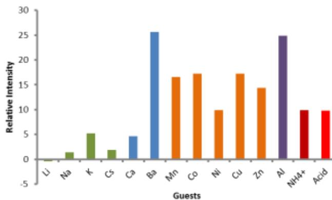
**SI Figure 3.** Relative fluorescence enhancement suppressing the PeT effect of PyC2ACE fluorophore (10  $\mu\text{M}$ , THF) in presence excess amount (10 times) of different cationic guests (100  $\mu\text{M}$ ).
