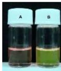
SI Figure 15. Absorbance spectral change of the PyC2ACE-ONP (6.8  $\mu$ M) solution in absence and in the presence of  $K^+$ -ions or **Pro** in in  $f_{w,90\%}$  and 1.0 mM HEPES buffer at 20  $^{\circ}$ C. Corresponding visual color change under the normal light of the hybrid solution in the absence (A) and presence (B) of **Pro**.
