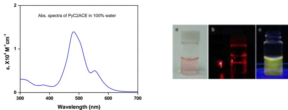
**SI Figure 2.** (left) Absorbance spectra of PyC2ACE in 100% aqueous solution at 10.0  $\mu\text{M}$  concentration and 25  $^\circ\text{C}$ ; (right) Images of the physical state of the solution in different conditions, (a) under normal light, (b) Rayleigh's scattering measured by using red-laser (635 nm), and (c) fluorescence image under UV-light (at 365 nm).
