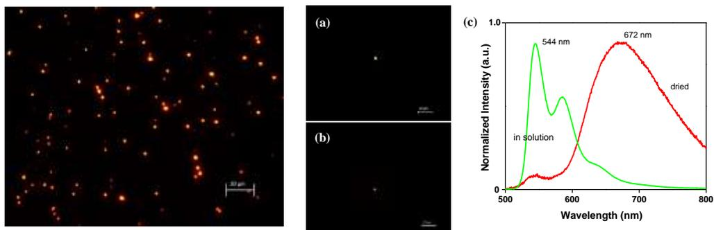
**SI Figure 5.** (left) The collective image of dried PyC2ACE OPNs in  $f_{w,70\%}$  at  $10.0 \mu\text{M}$  and  $20^\circ\text{C}$ . Single particle characterization by excitation of 450-490 nm: (a) solution state image; (b) dried state image, and (c) their corresponding FL spectra.
