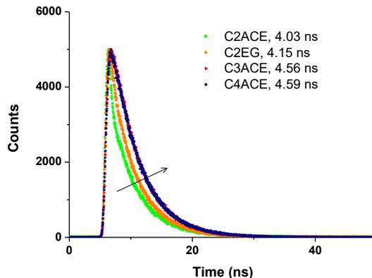
**SI Figure 11.** Fluorescence decay profiles were measured for the samples at  $10.0\ \mu\text{M}$  concentration, and  $20^\circ\text{C}$ .
