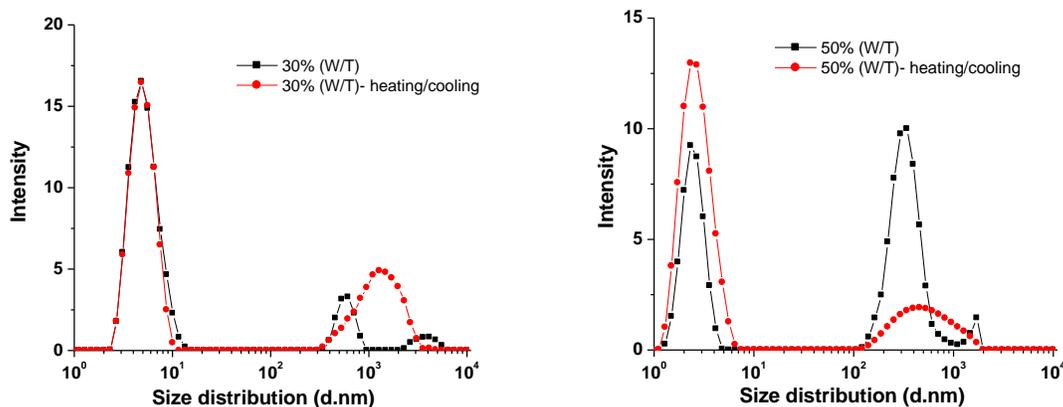
SI Figure 8. Particle size distribution is plotted against the data collected in DLS experiment for PyC2ACE in  $f_{w,30\%}$  and  $f_{w,50\%}$  at 10.0  $\mu\text{M}$  and 20  $^{\circ}\text{C}$ , after simple solvent mixing and following heating-cooling method.
