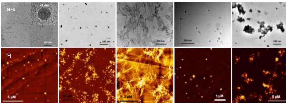
**Figure 6.** (a-e) TEM and (f-j) AFM images were observed for the nano-aggregates of PyC2ACE, PyC2EG, PyC3ACE, PyC4ACE, and PyBzACE derivatives prepared at  $f_{w,70\%}$ ,  $10.0 \mu\text{M}$  and  $20^\circ\text{C}$ , then aging for 1 hr [inset of Figure 4a: TEM image of a single-nanoparticle having diameter of 44 nm].
