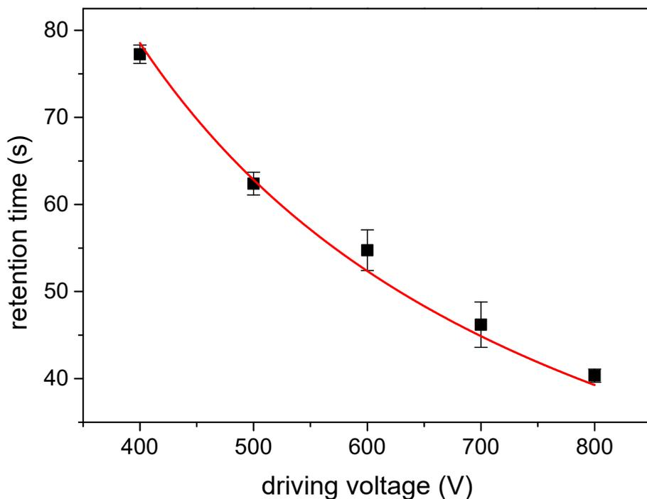
**Fig S6.** The retention time of cascade reaction product ( $\text{H}_2\text{O}_2$ ) as a function of separation voltage. Substrate concentration: 12 mM lactose.
