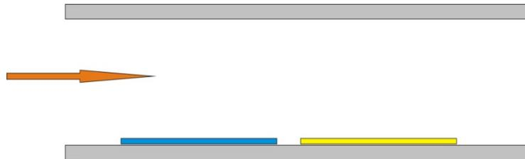
**Fig S2.** Computation domain in the FEM model. The blue and yellow regions denote the immobilized enzymes in the microchannel. The gray region represents the channel wall of microchip. The arrow with orange color represents flow direction of fluid.
