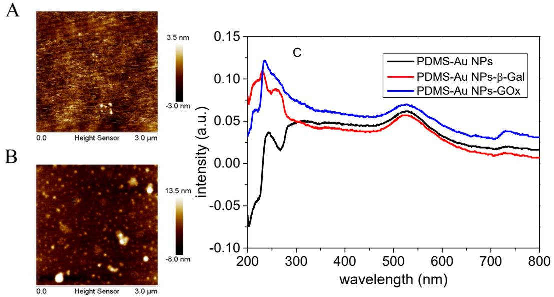
**Fig. S1.** AFM images of a bare PDMS surface (A) and Au-films PDMS surface (B). (C) UV-vis absorbance spectra of gold nanoparticles patterned PDMS (black curve) and after enzymes immobilization (red curve).
