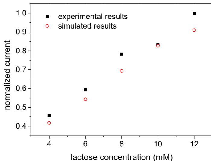
**Fig. S3** Relationship between lactose concentration and the electrochemical response current in microchannel. (■, square) experimental results; (○, circle) simulated results. Experimental and Simulated currents of  $\text{H}_2\text{O}_2$  were normalized by using the current for 12 mM lactose at a 50  $\mu\text{m}$  gap distance.
