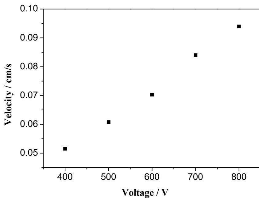
**Fig S5.** The velocity versus separation voltage in microchannel without enzymes.
