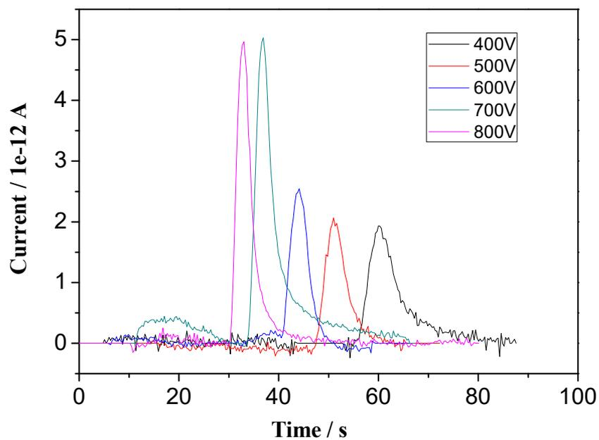
**Fig S4.** The eluted curves for H<sub>2</sub>O<sub>2</sub> in microchannel without enzymes under different separation voltages.
