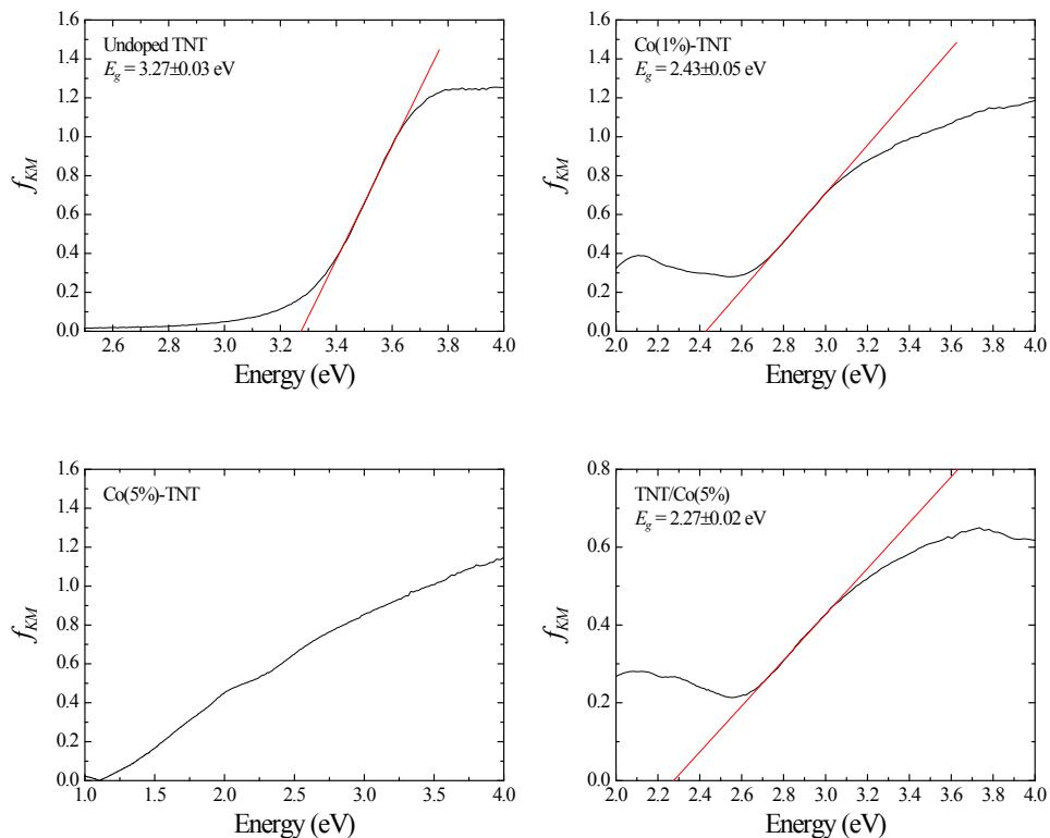
**Fig. S3 –** Tauc plots for TNT, Co(1%)-TNT, Co(5%)-TNT and TNT/Co(5%) samples.
