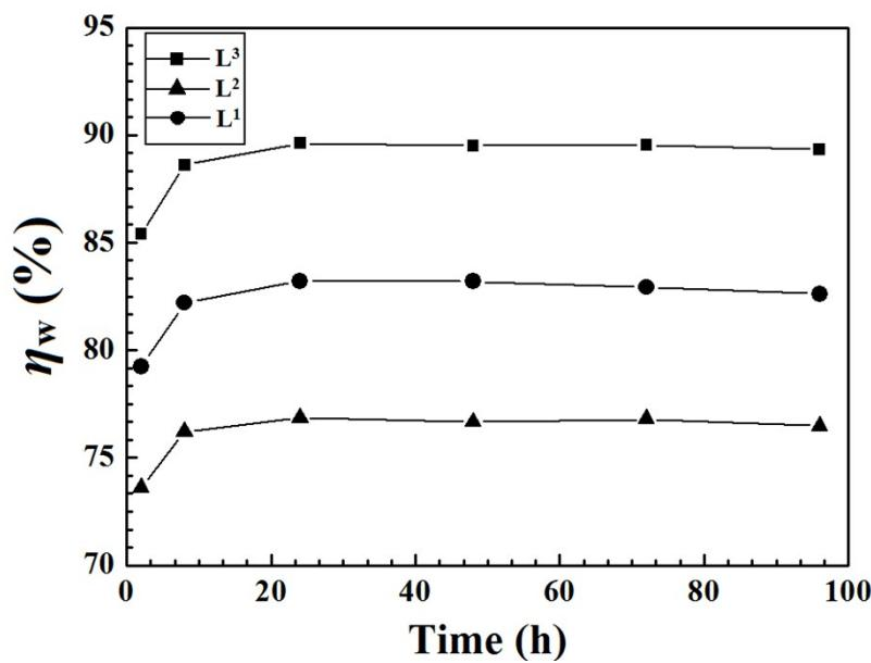
**Fig. S10** Variation of inhibition efficiency obtained from weight loss measurement at 1 mM concentration of three Schiff bases having different immersion time (1-96 hr) towards corrosion of mild steel in 1M HCl.
