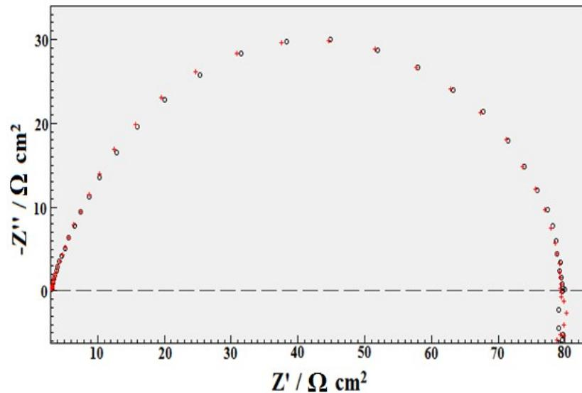
**Fig. S9** EIS fitting curve of  $L^3$  inhibitor having 1mM concentration.
