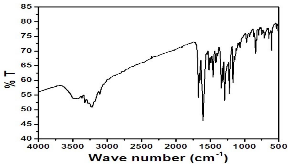
Fig. S3 FTIR spectrum of  $\text{L}^3$ .
