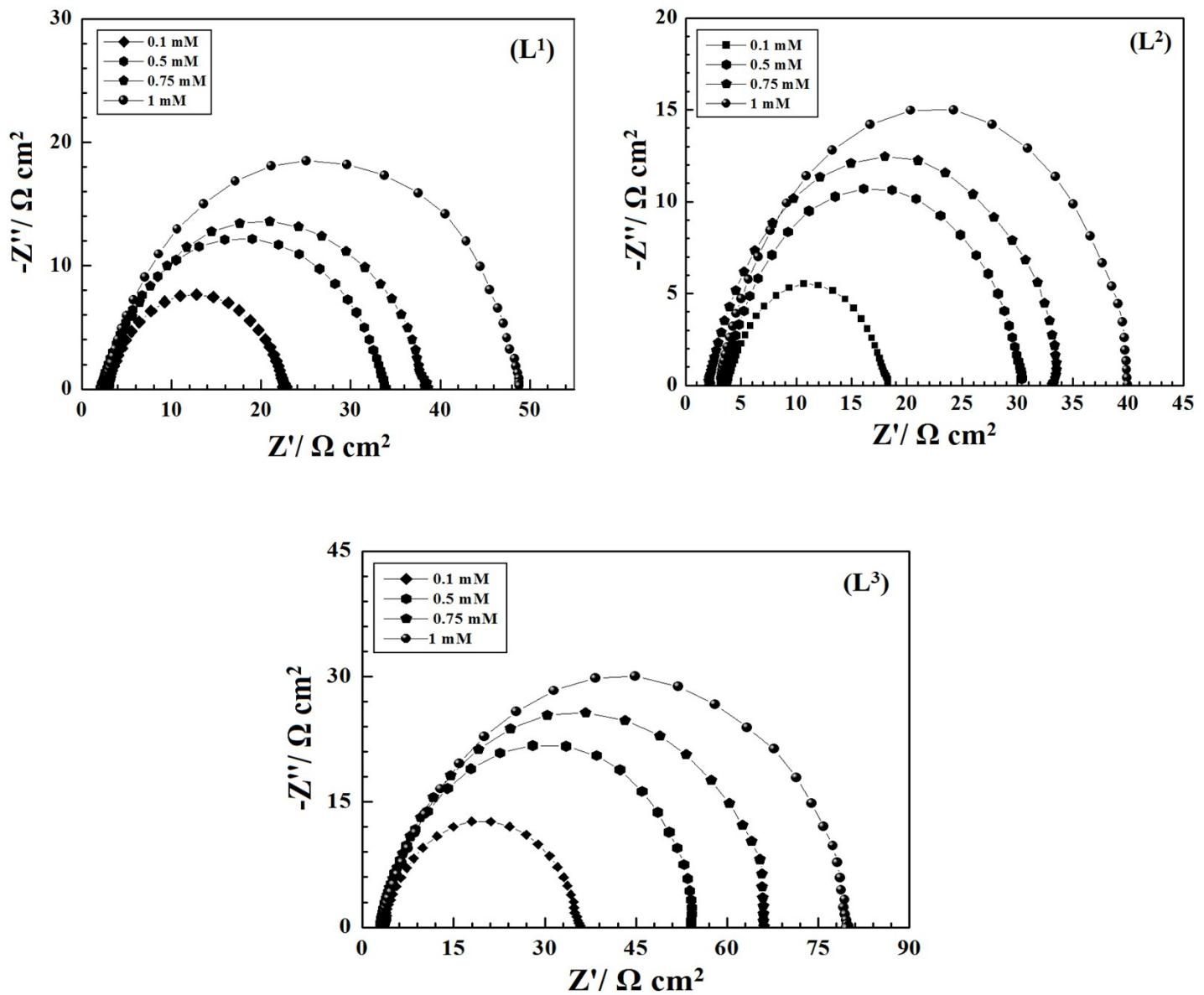
**Fig. S8** Nyquist impedance diagram for mild steel in 1 M HCl solution in presence of Schiff bases ( $L^1$ ,  $L^2$  and  $L^3$ ) with different inhibitor concentration.
