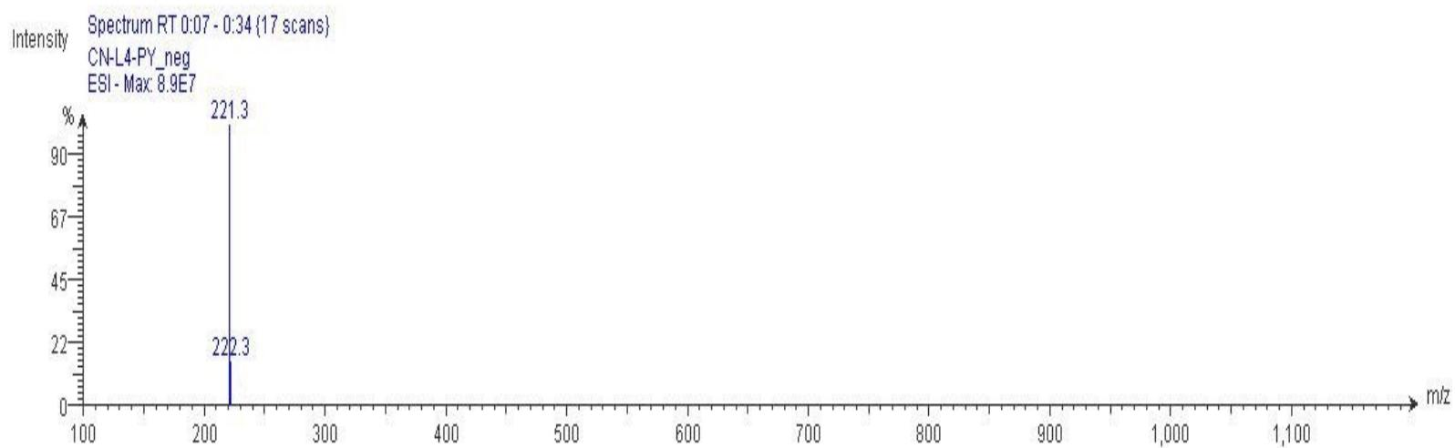
**Fig. S5** ESI-MS spectrum of  $L^2$  in methanol.
