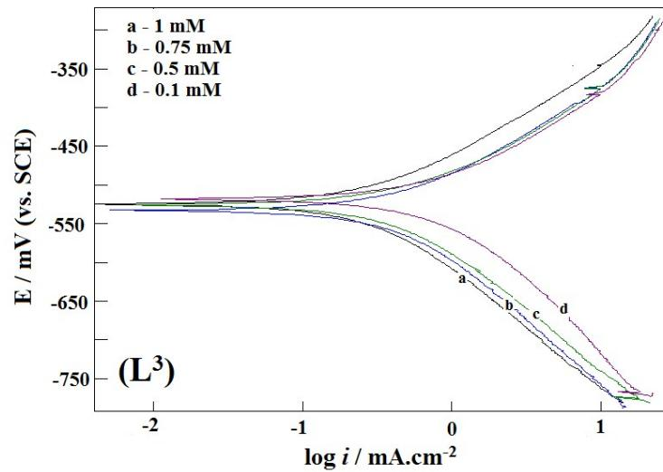
**Fig. S7** Tafel polarization curves for mild steel in 1 M HCl solution in the presence of Schiff bases ( $L^1$ ,  $L^2$  and  $L^3$ ) with varying inhibitor concentration.
