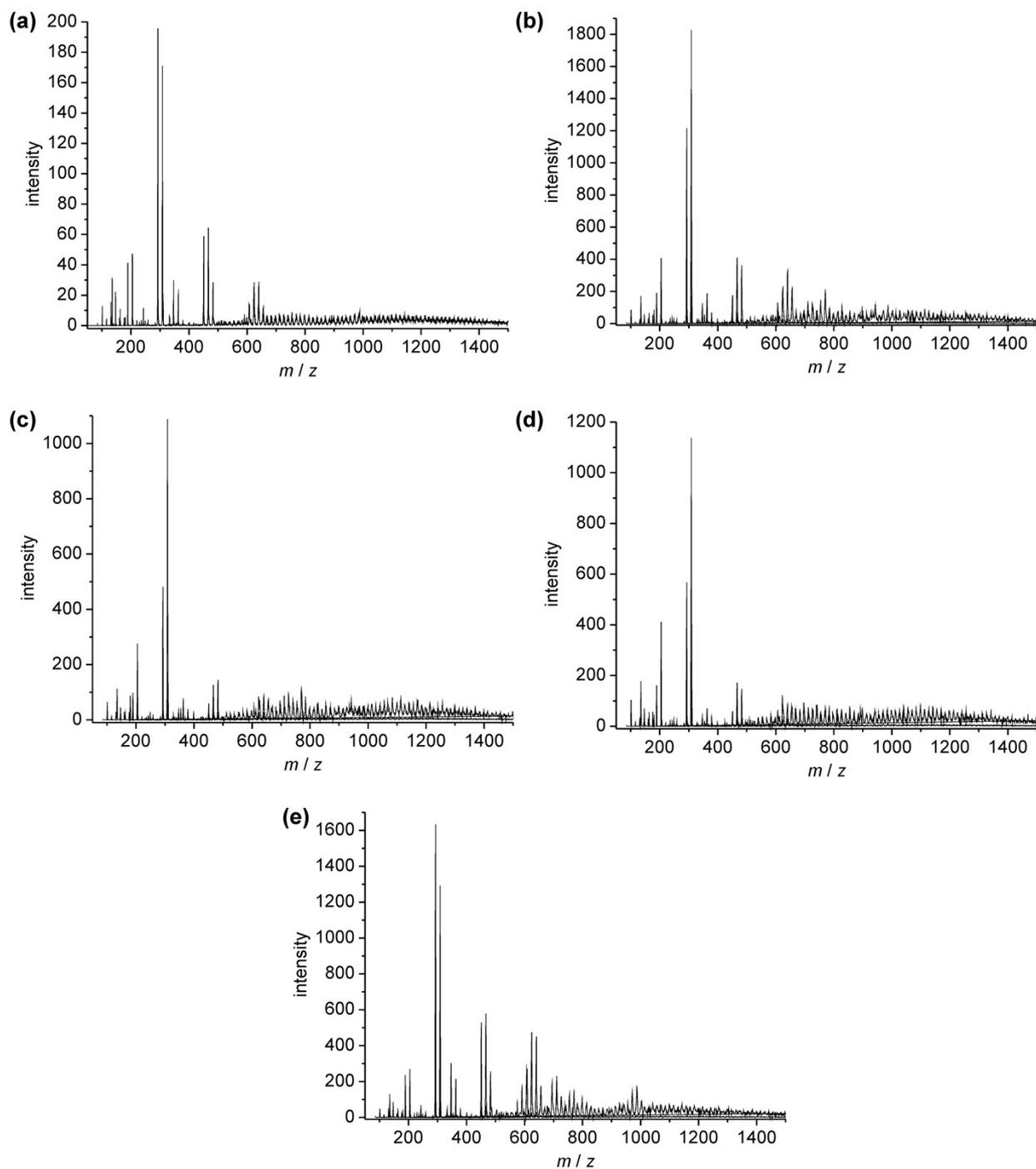
**Fig. S6.** Comparison of full ESI mass spectra of degradation products of (a) E1, (b) E2, (c) E3, (d) EE2, and (e) DES estrogens after treatment with ferrate(V).
