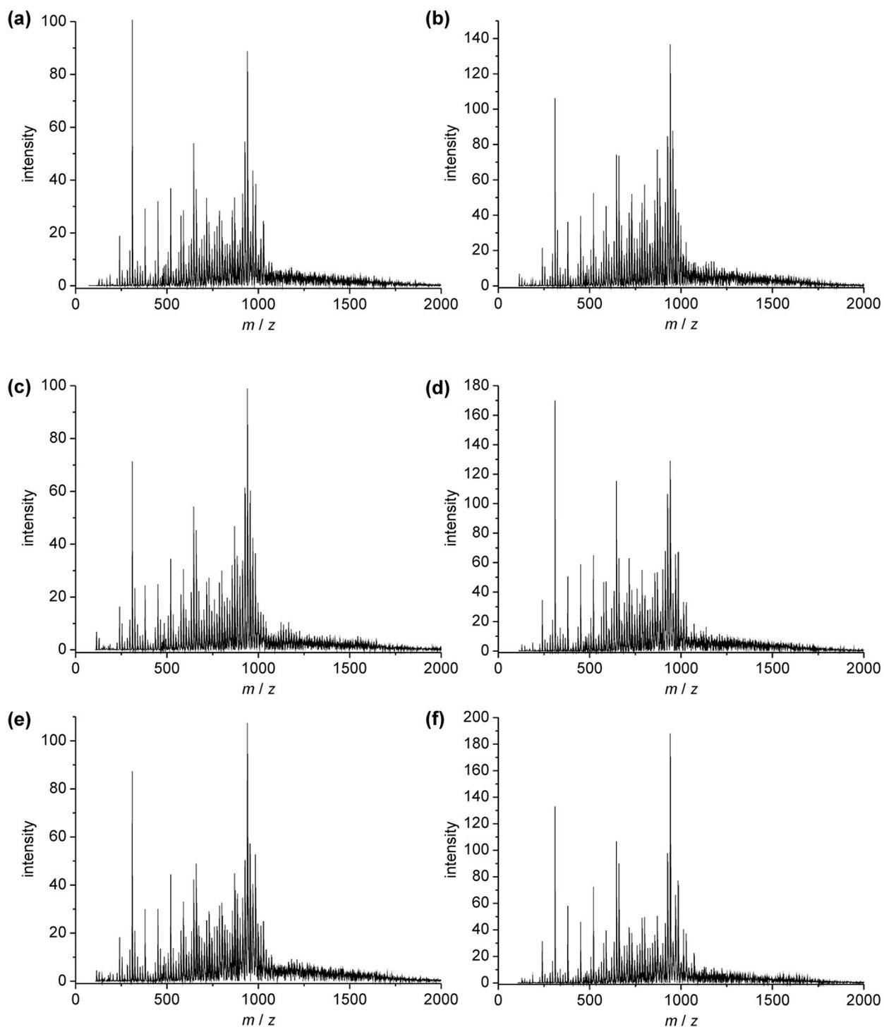
**Fig. S7.** Comparison of full ESI mass spectra of degradation products of (a) E1, (b) E2, (c) E3, (d) EE2, and (e) DES estrogens after treatment with ferrate(VI) together with (f) ESI mass spectrum of pure  $K_2FeO_4$  decomposed in water/MeOH.
