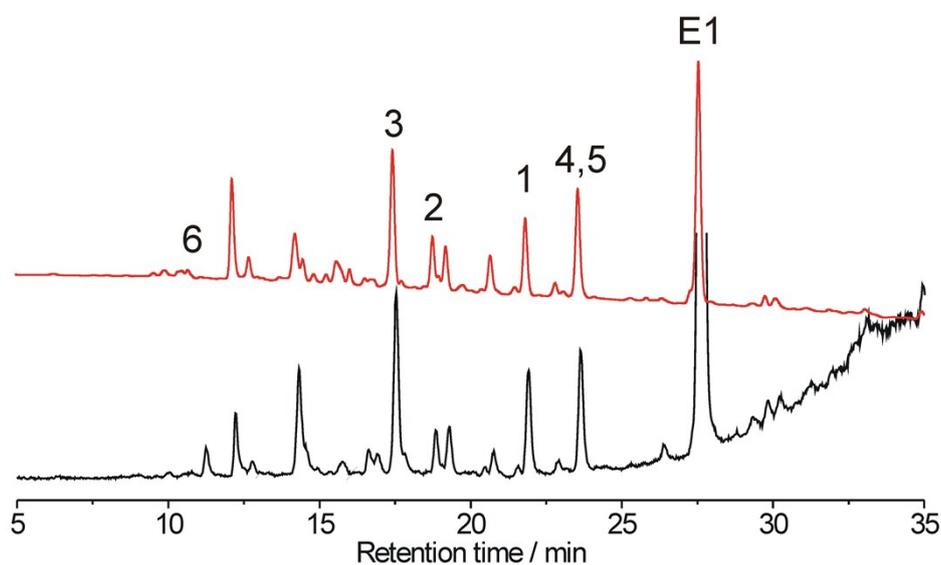
**Fig. S8.** Data from HPLC-MS analysis of E1 degradation by ferrate(VI) (UV-VIS detector (230 nm) – in red color, positive MS mode (total ion current) in black color) together with the table summarizing the proposed structures of the observed intermediates with the corresponding masses, retention times, and assignment (positions) in chromatogram. The intermediates are numbered according to the oxidation pathway.
