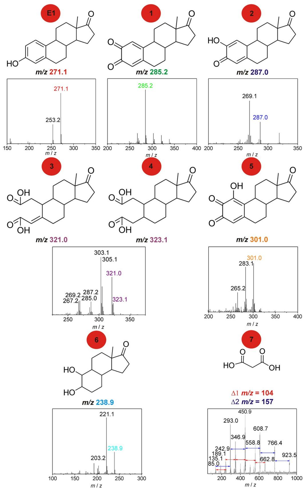
**Fig. S9.** Structural formulas and ESI mass spectra of intermediates of E1 degradation by ferrate(VI).
