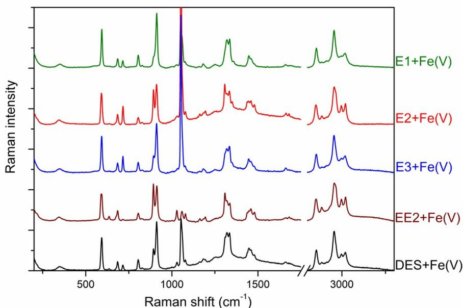
**Fig. S3.** Comparison of the Raman spectra of degradation products of E1, E2, E3, EE2, and DES estrogens after treatment with ferrate(V). The spectra are normalized with respect to the peak located at  $2953\text{ cm}^{-1}$  for the sake of the visualization of less intensive peaks.
