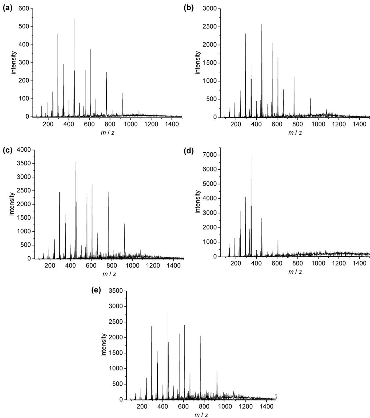
**Fig. S5.** Comparison of full ESI mass spectra of degradation products of (a) E1, (b) E2, (c) E3, (d) EE2, and (e) DES estrogens after treatment with ferrate(IV).
