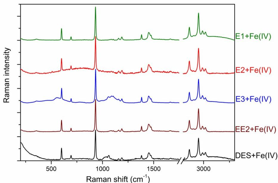
**Fig. S2.** Comparison of the Raman spectra of degradation products of E1, E2, E3, EE2, and DES estrogens after the treatment with ferrate(IV). The spectra are normalized with respect to the most intensive peak (located at  $934\text{ cm}^{-1}$ ).
