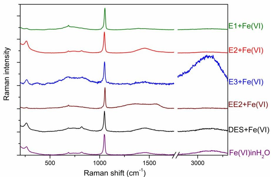
**Fig. S4.** Comparison of the Raman spectra of degradation products of E1, E2, E3, EE2, and DES estrogens after treatment with ferrate(VI). Raman spectrum of  $K_2FeO_4$  dissolved in water is shown for the sake of a direct comparison. The spectra are normalized with respect to the most intensive peak (located at  $1048\text{ cm}^{-1}$ ).
