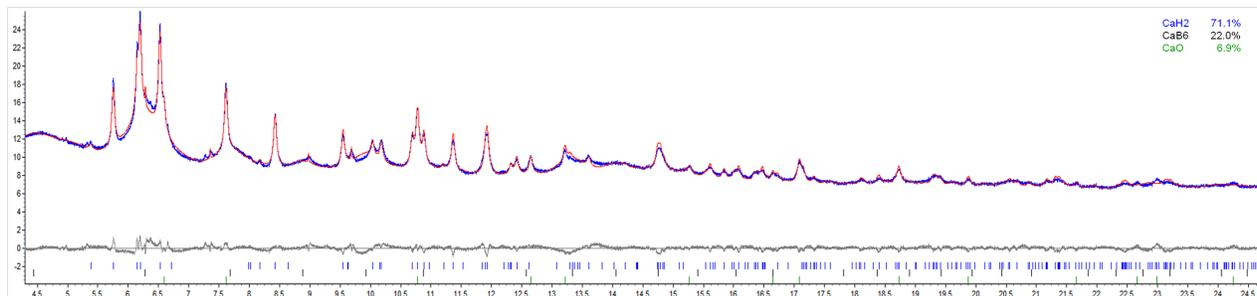
**Fig. 3** Measured data and Rietveld refinement of the sample annealed at 400 °C for 2 h. The data are shown on a  $2\theta$  scale in degrees. The used x-ray wavelength was  $\lambda = 0.32 \text{ \AA}$ .
