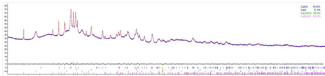
**Fig. 2** Measured data and Rietveld refinement of the sample annealed at 400 °C for 0.5 h. The data are shown on a 2 $\theta$  scale in degrees. The used x-ray wavelength was  $\lambda = 0.4 \text{ \AA}$ .
