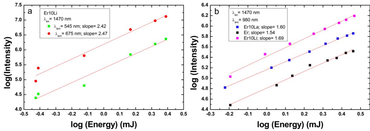
**Fig. S6** Integrated up - conversion emission intensities corresponding to 545, 675 and 980 nm based emission of Er as a function of laser energy pulse (excitation wavelength = 1470 nm)
