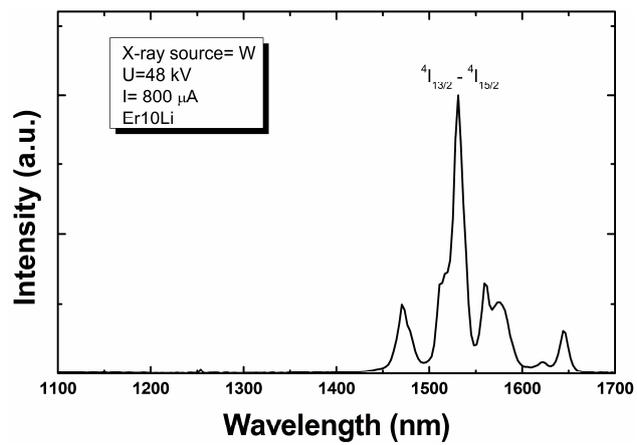
**Fig. S4.** Near - infrared emission at 1500 nm of Er10Li – CeO<sub>2</sub> measured under X-ray excitation.
