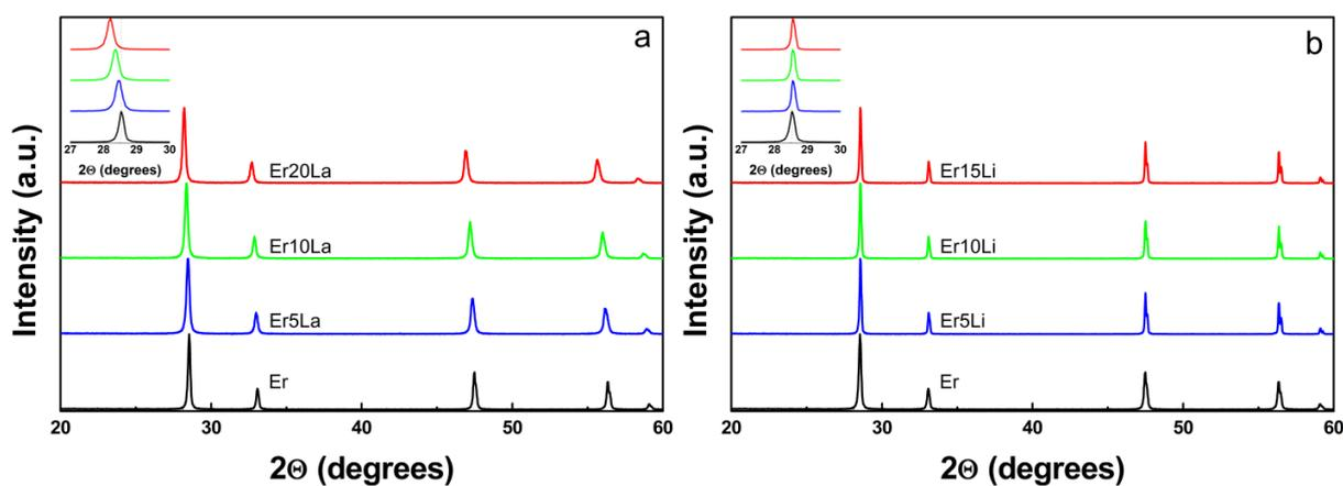
**Fig. S1.** Effects of La (a) and Li (b) co - doping on the phase and crystallite size (XRD patterns) of Er - CeO<sub>2</sub>.
