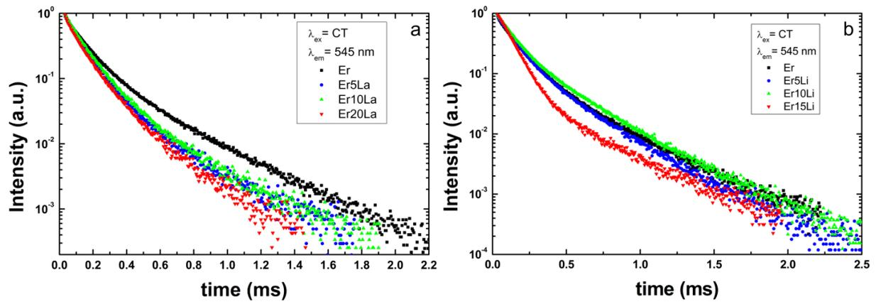
**Fig. S3** Effects of La (a) and Li (b) co - doping on the charge – transfer (CT) excited emission decays of Er - CeO<sub>2</sub> measured at 545 nm.
