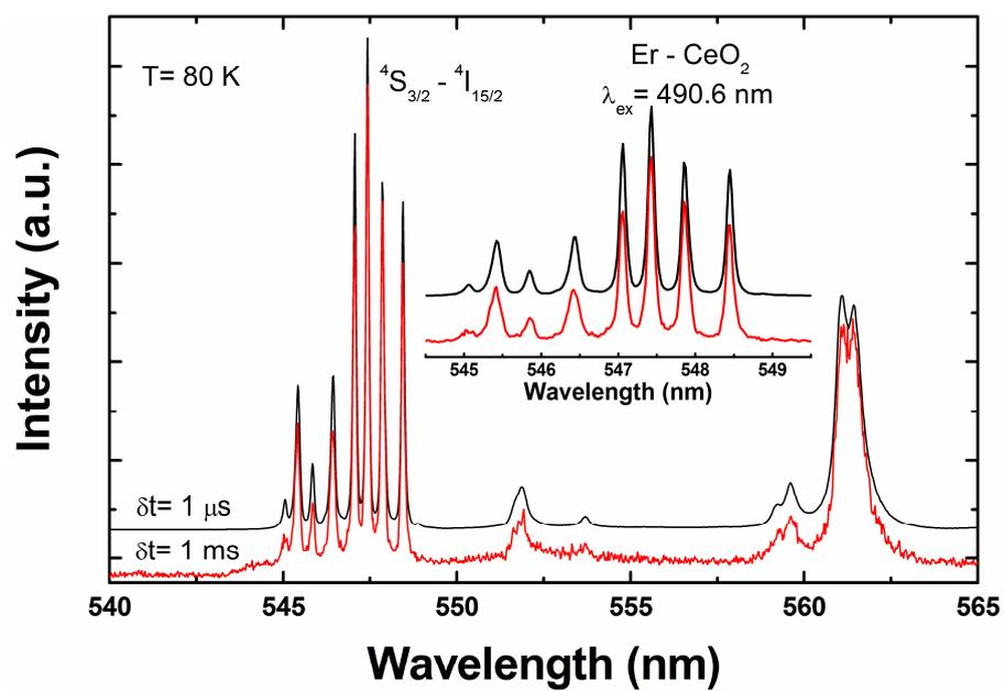
**Fig. S7** Time – gated emission spectra of Er – CeO<sub>2</sub> highlighting the  ${}^4S_{3/2} - {}^4I_{15/2}$  transition measured at 80 K.
