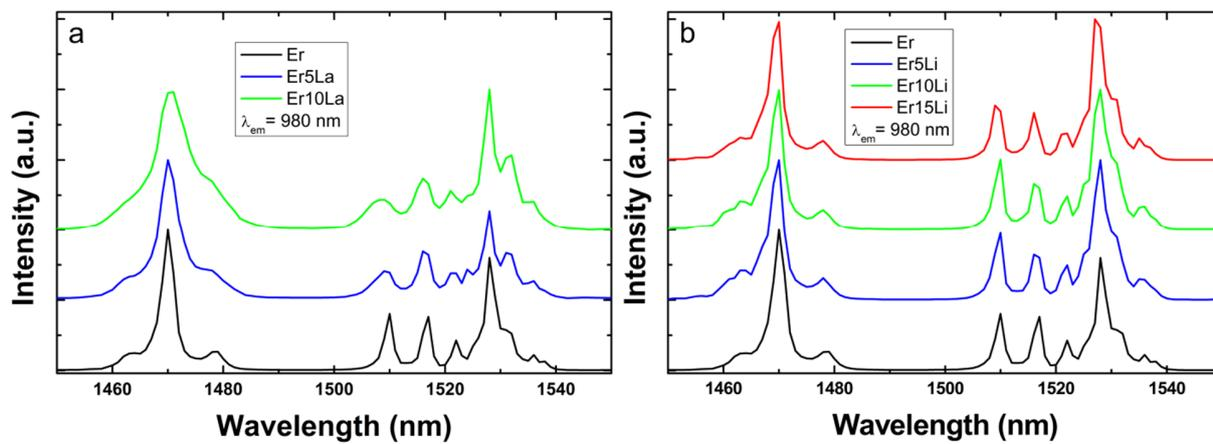
**Fig. S5.** Effects of La (a) and Li (b) co - doping on the up – conversion excitation spectra of Er - CeO<sub>2</sub> monitoring the near – infrared emission at 980 nm.
