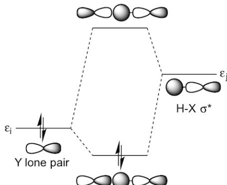
**Figure S1.** Simplified representation of the donor- acceptor interaction between localised NBO fragment orbitals upon H-bond formation (X-H $\cdots$ Y).
