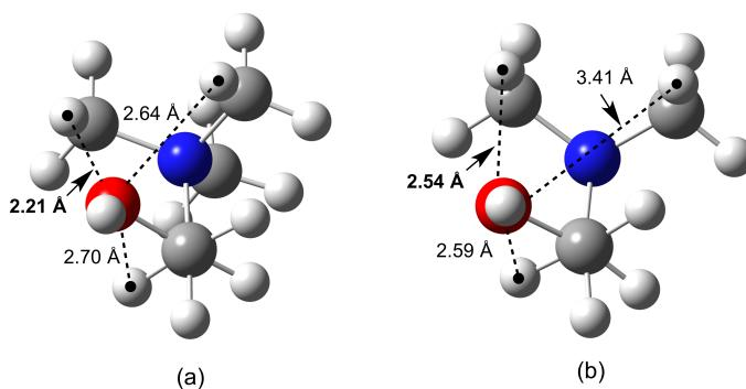
**Figure S4.** CH...OH interaction distances within (a) gauche choline and (b) gauche *N,N*-dimethylethanamine
